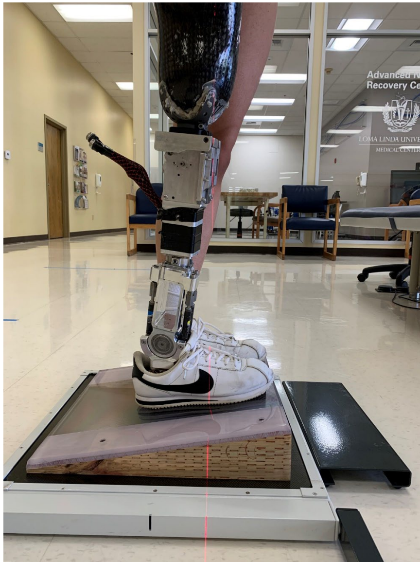
Figure 25 RPL with APxA demonstrates knee and ankle stability on a 10° incline. The laser line demonstrates the true center of gravity symmetrically passing through both extremities
