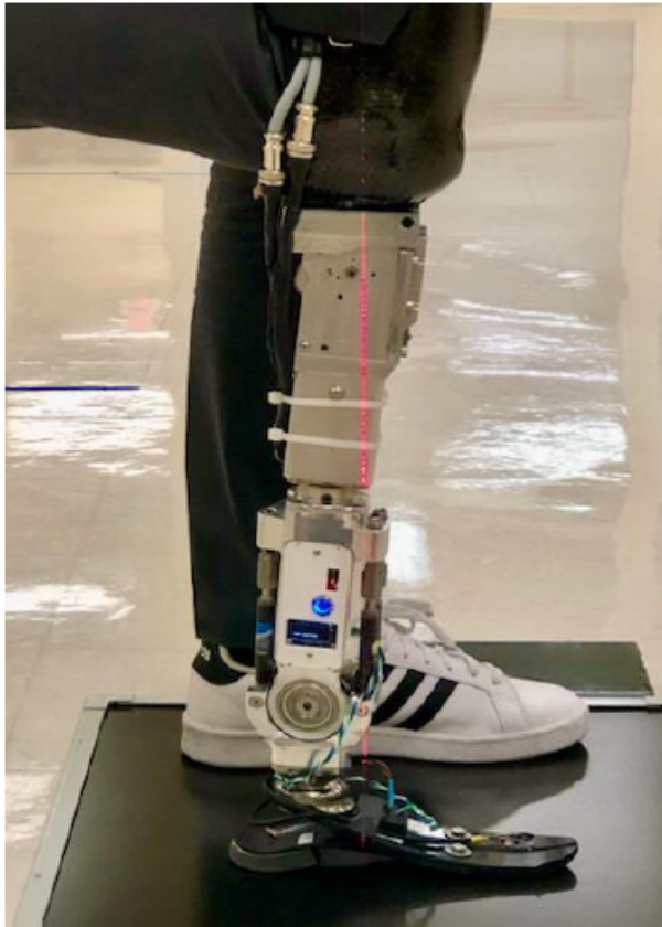
FIGURE 6: COMPLETED PROSTHESIS ON NON-AMPUTEE HUMAN SUBJECT WITH TUNED BIOLOGICALLY CORRECT ALIGNMENT
