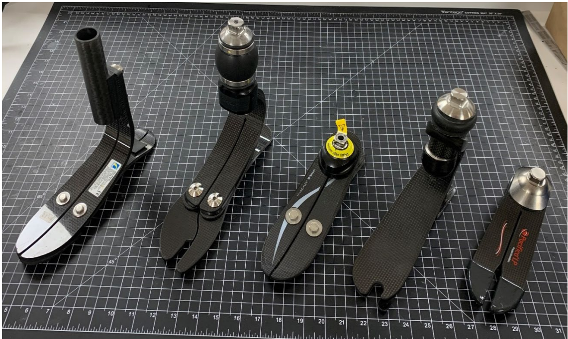
Figure 12 Examples of COTS CC Feet, left to right Össur Vari-Flex®, Össur Pro-Flex® with VSP, Össur LP Vari-Flex®, Freedom Innovations Renegade®, Freedom Innovations Pathfinder®.
