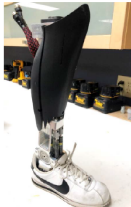
FIGURE 2: CONFIGURED PROTOTYPE WITH 3D PRINTED COSMETIC PROTECTIVE FAIRING
