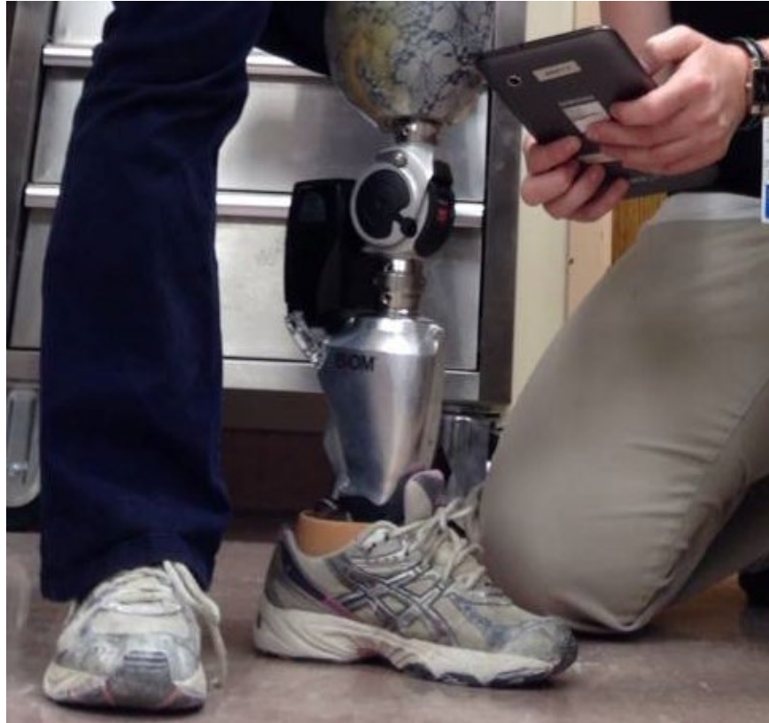
Figure 18 First generation BiOM® powered ankle being programmatically tuned by the prosthetist using an HMI mobile device
