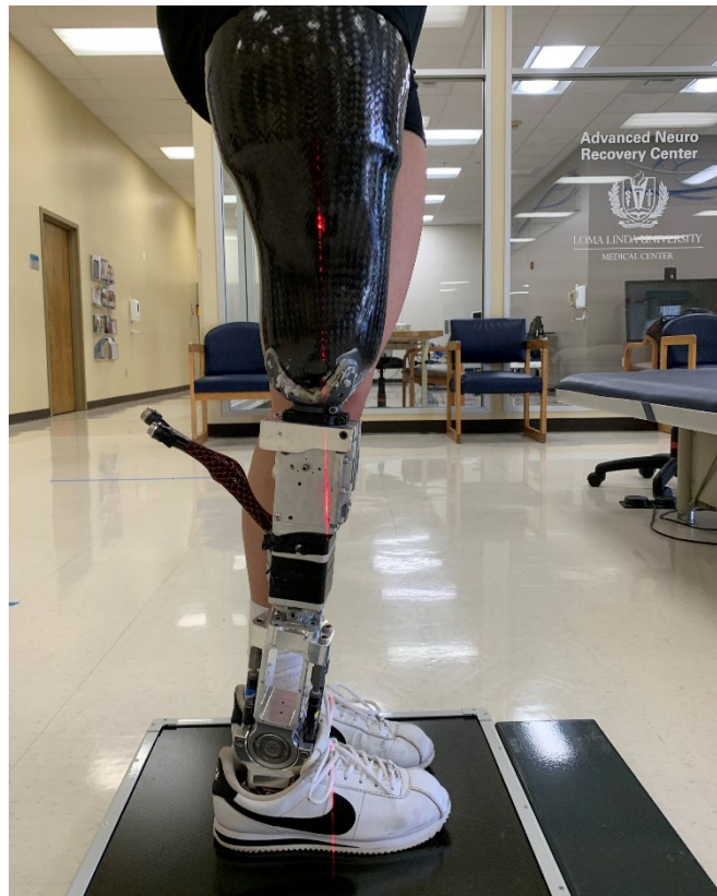
Figure 4 LASAR Posture®. Laser line, represents vertical ground reaction in relationship to the trochanter, knee, and ankle (TKA)
