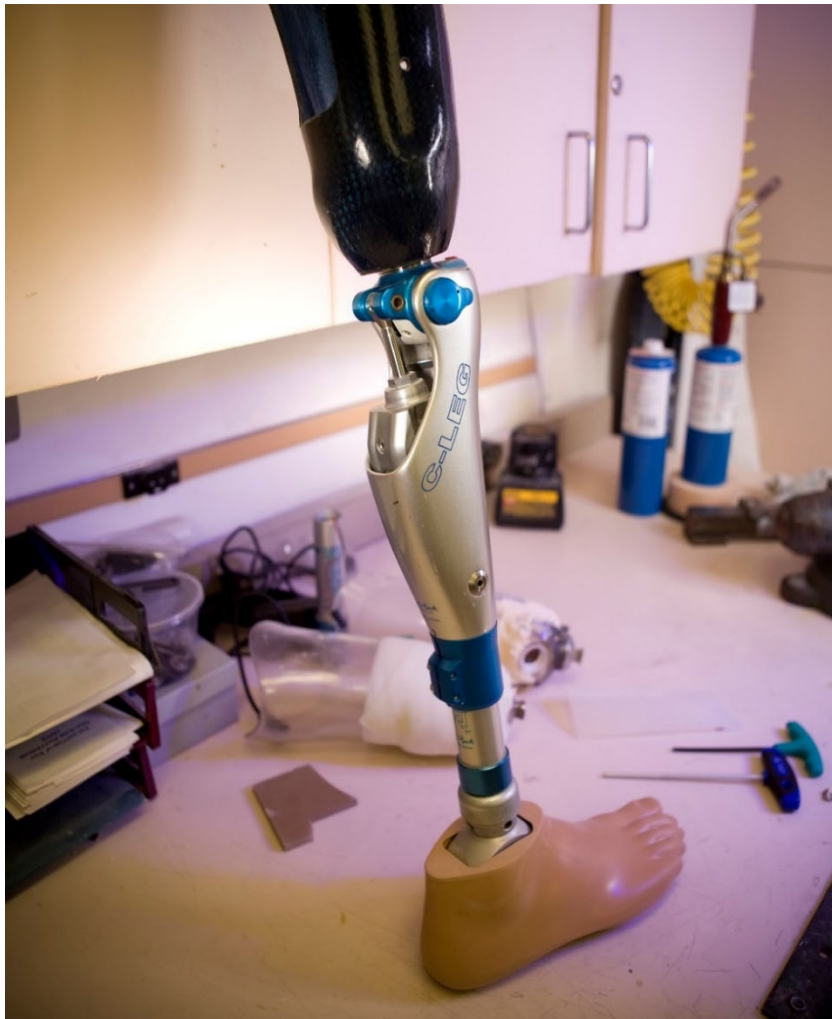
Figure 13 First generation Ottobock C-Leg® sa-MPK – image courtesy of Loma Linda University Health.
