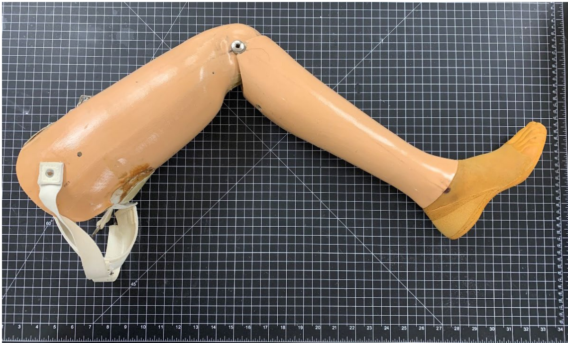
Figure 5 Non-modular type prosthesis with single-axis, constant friction knee and SACH foot.
