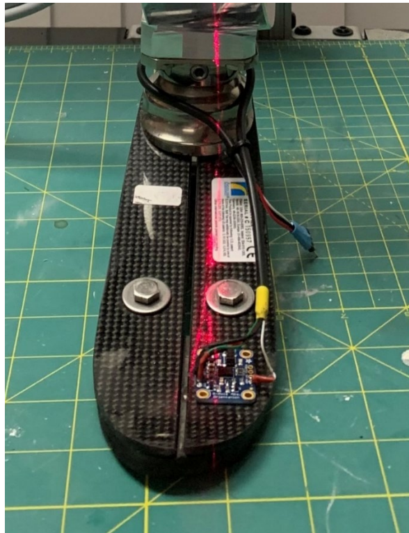
Figure 20 CC foot instrumented with BNO550 IMU.
