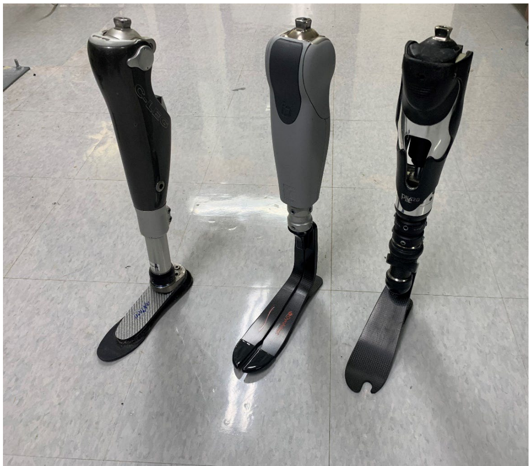
Figure 16 Examples of sa-MPK with CC feet. Left to right, C-Leg®, Rheo®, and Plie®.
