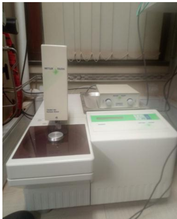
Figure 8. A Mettler Toledo DSC (821e/700) Equipment (Department of Geology, University of Free State, South Africa)
