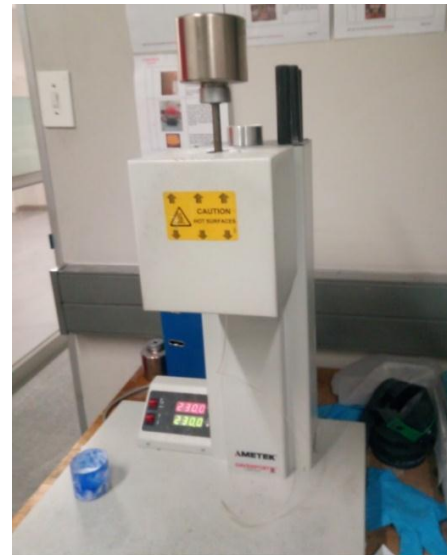
Figure 10. MFI Tester from Ametex Ltd (Centre for Rapid Prototyping and Manufacturing, Central University of Technology, Free State)
