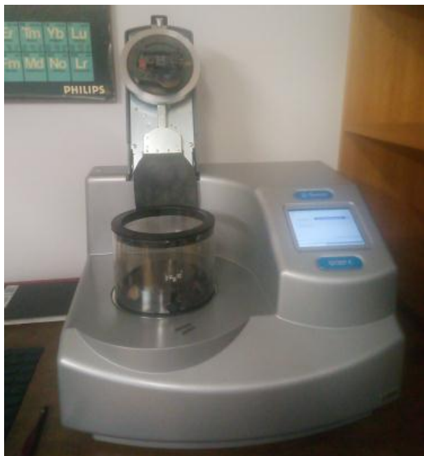
Figure 6. A Carbon Coater (Department of Geology, University of Free State, South Africa)
