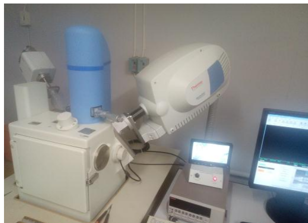
Figure 7. A JSM-6610LV Scanning Electron Microscope (Department of Geology, University of Free State, South Africa)
