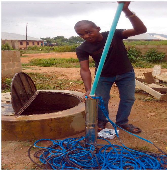
Fig. 6. Showing recovery test in unscreened well in study area.
