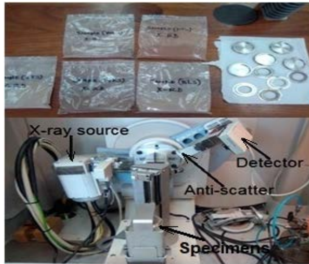
Figure 1. Sample preparation by front loading and multipurpose diffractometer used for the XRD test
