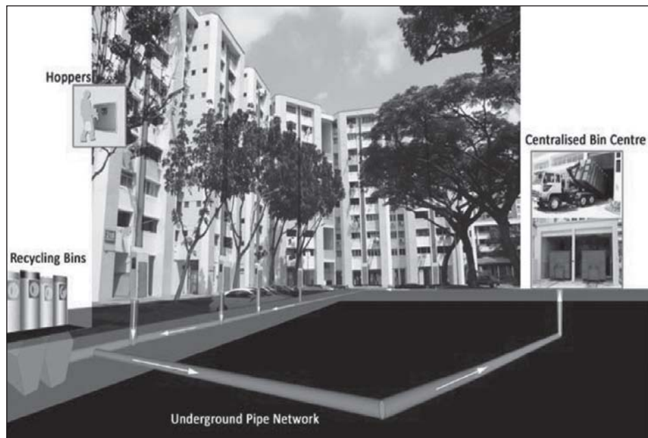
FIGURE 5 Pneumatic Waste Conveyance Systems (PWCS)
