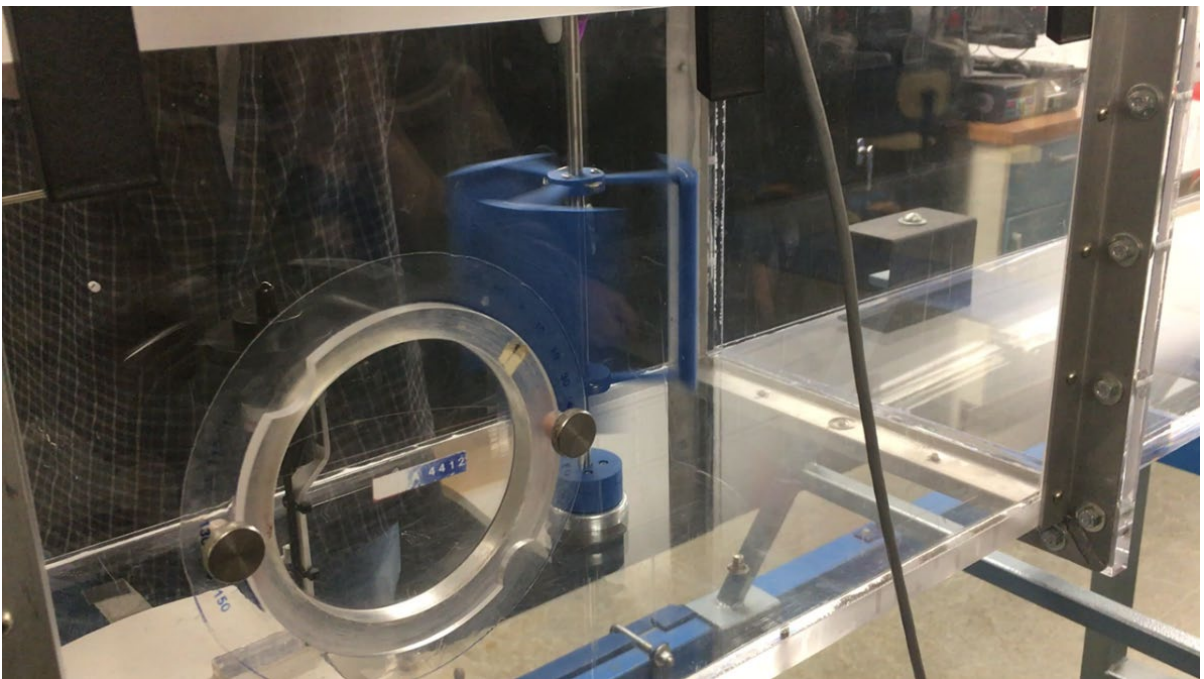
Figure 13: Scale model of an airfoil design VAWT being tested in the wind tunnel.
