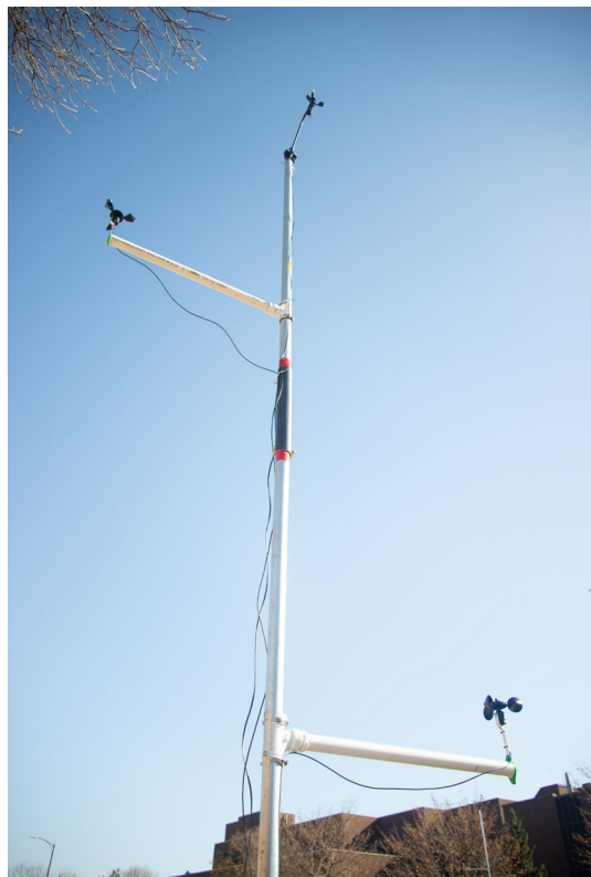
Figure 10: Anemometer tower assembled with three mounted sensors.
