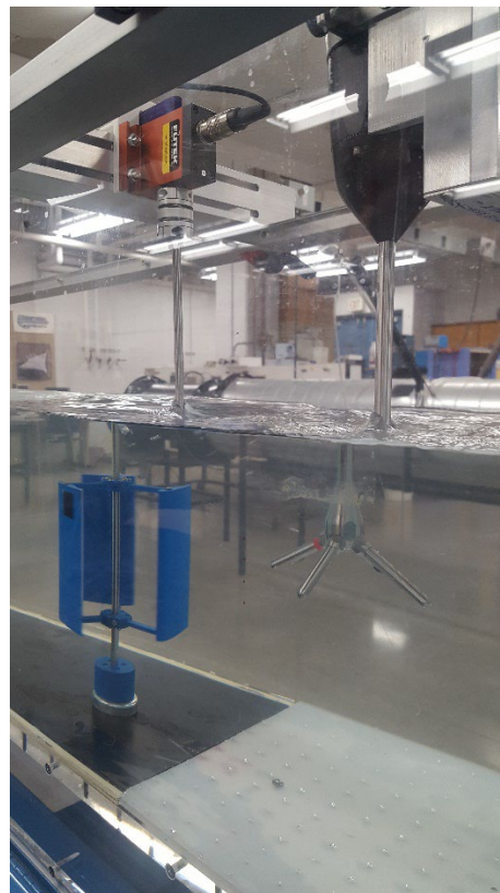
Figure 17: Vectrino shown measuring flow field around a model VAWT in the water channel.
