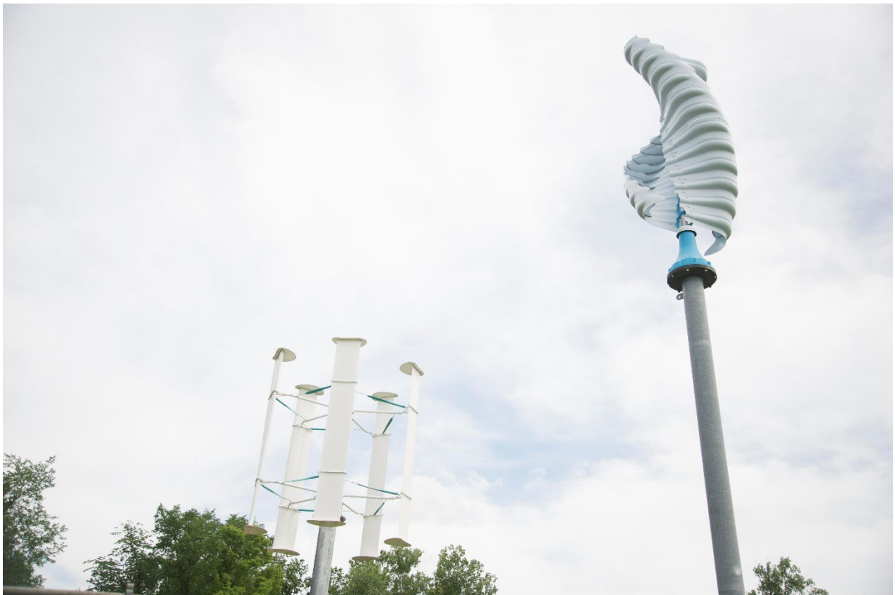
Figure 2: Test VAWTs installed on the Minnesota State University, Mankato campus (Darrieus on the left and Savonius on the right).
