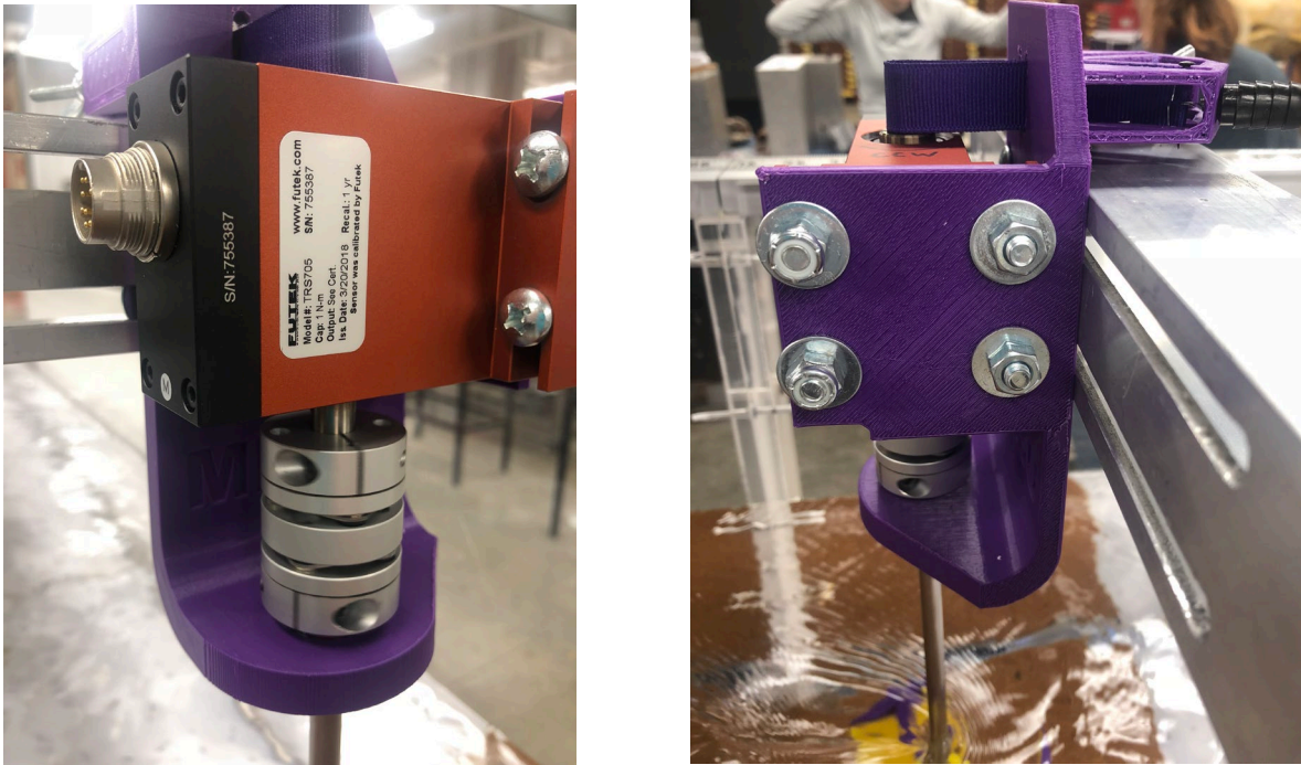
Figure 18: The Futek torque sensor and its 3D printed mount for the water channel.
