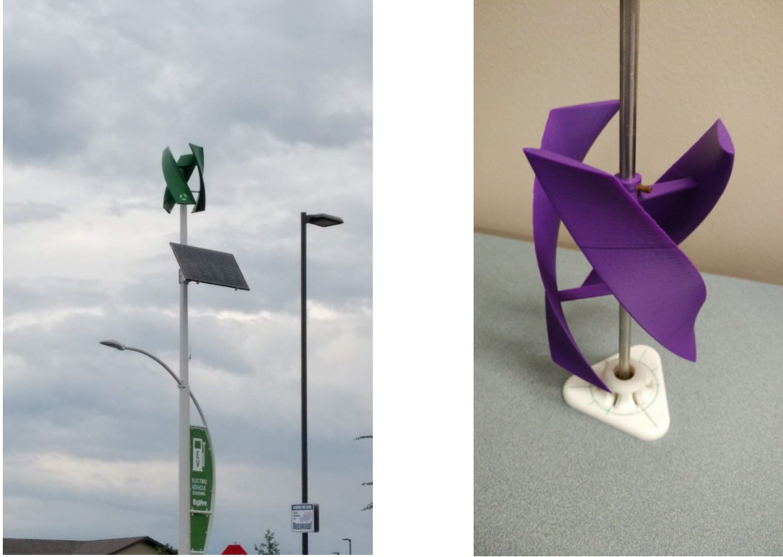
Figure 14: An electric vehicle charging station at HyVee (left). A scale model of the same VAWT that was 3D printed (right).
