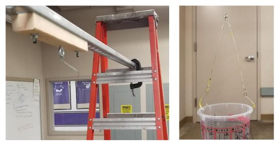
Figure 6. Simple paint pendulum set-up
