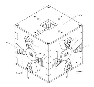
Figure 3.9: Three-dimensional face and contact identifier layout view.
