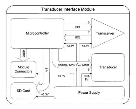
Figure 2.2: Transducer Interface Module block diagram.
