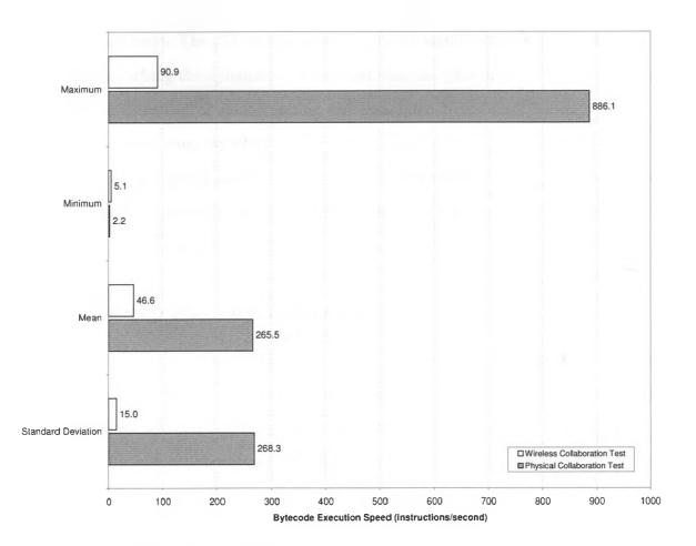
Figure 7.7: Virtual machine bytecode execution speeds.
