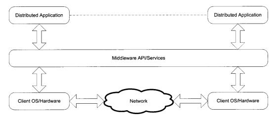
Figure 4.1: Middleware operation block diagram.
