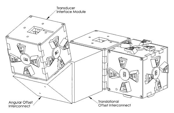
Figure 2.1: Transducer Interface Modules and interconnects.
