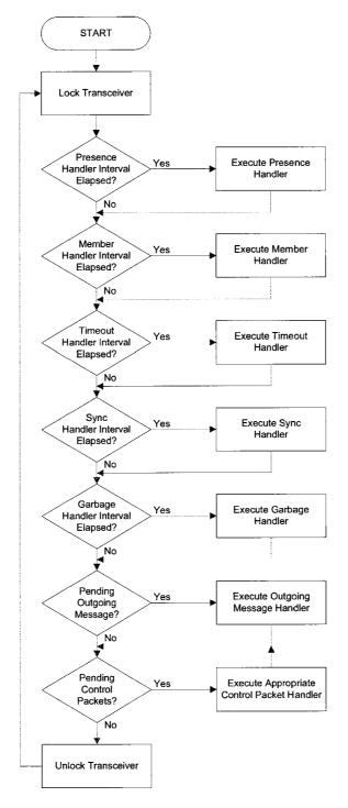
Figure 3.8: Network communication task operation.
