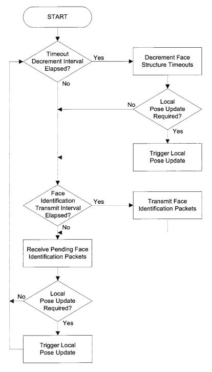
Figure 3.12: Face communication task operation.
