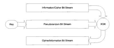
Figure 3.3: Stream cipher operation block diagram.
