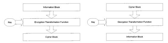
Figure 3.4: Block cipher operation block diagram.
