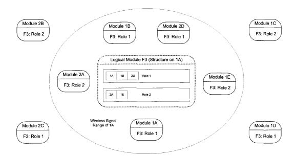
Figure 6.1: Logical module operation block diagram.
