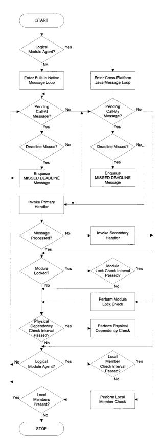
Figure 4.4: Module message handler task operation.
