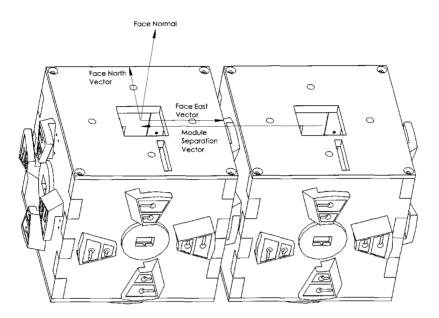
Figure 5.1: Module pose vectors.
