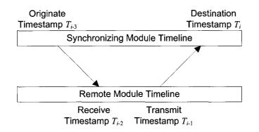
Figure 3.2: Time synchronization packet exchange.
