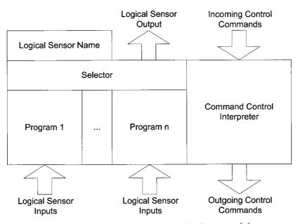
Figure 1.1: Logical sensor block diagram [2].
