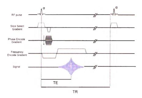
Figure 1.11: Gradient Echo Pulse Sequence
