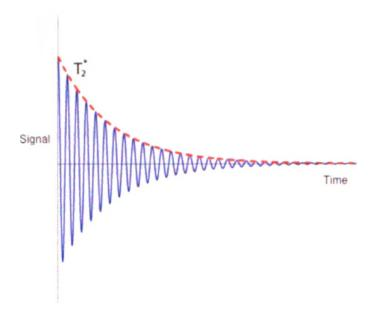
Figure 1.6: FID Curve of a Sample
