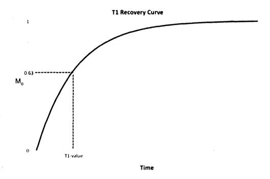
Figure 1.7: T1 Recovery Curve After a 90° Pulse
