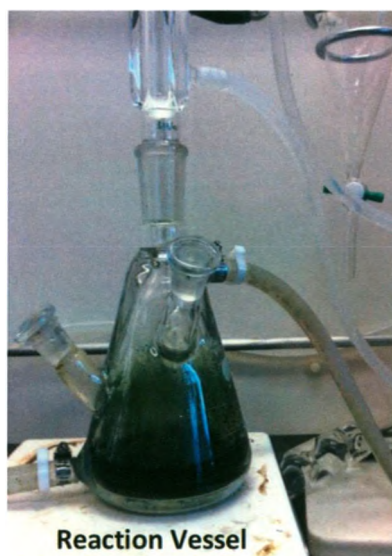
Figure 3.10: Transesterification reaction vessel design
