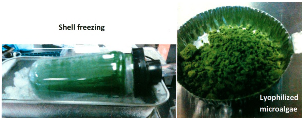
Figure 3.8: Shell freezing technique and the lyophilized UTEX 2714
