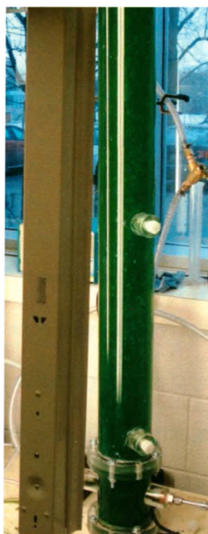
Figure 3.4: Tubular photo bioreactor in operation
