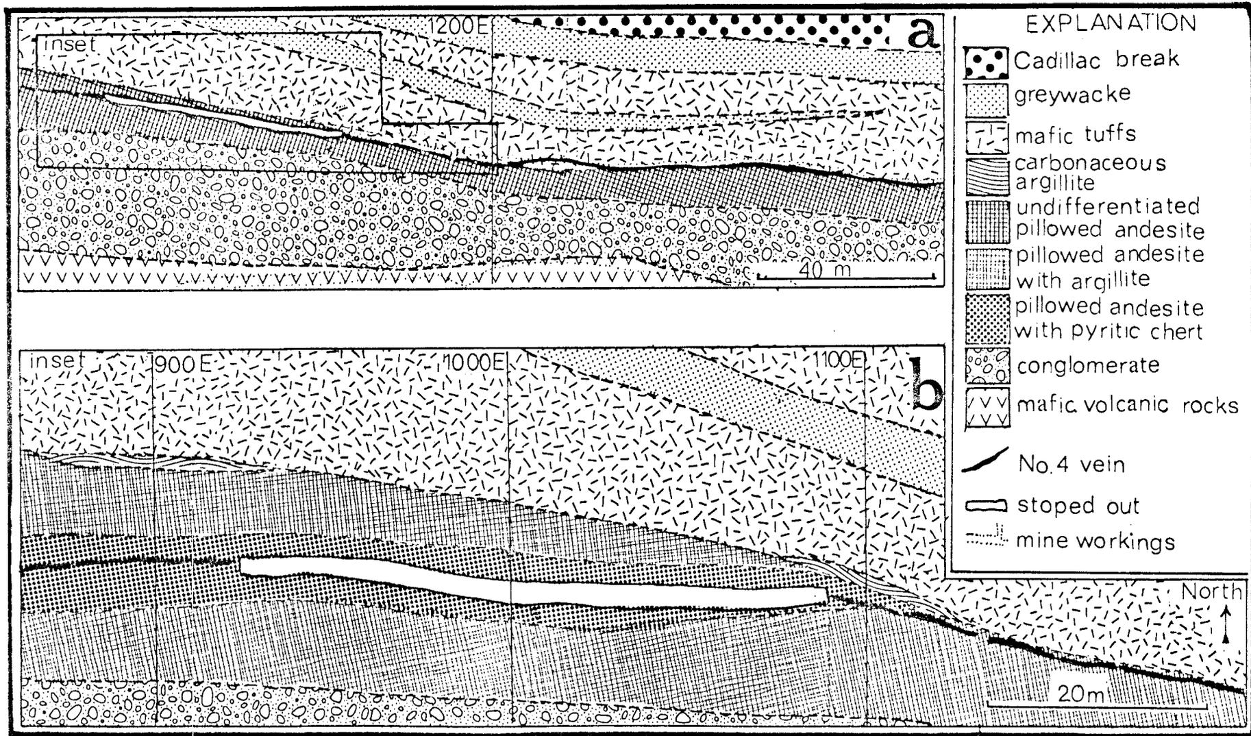
FIGURE 15 PLAN OF NO. 4 VEIN ON 500' LEVEL
