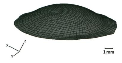
Figure 2.4: Sample FE model of a contact lens.
