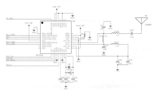
Figure 3-17 nRF24Z1 Schematic in Transmitter
