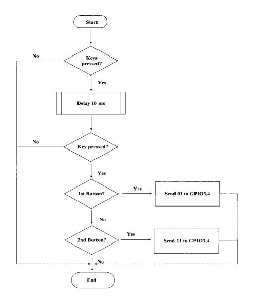
Figure 4-6 Flowchart of Detecting and Sending Button Status
