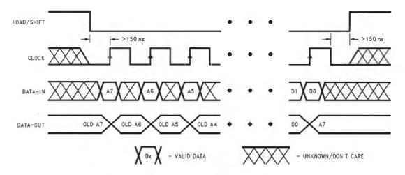
Figure 3-10 LM1973 Control Timing [25]
