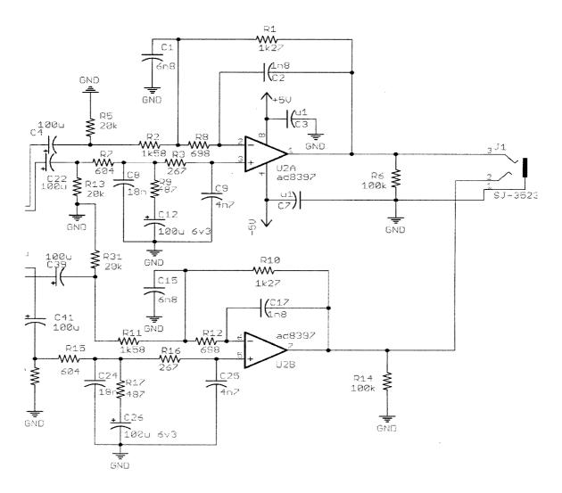
Figure 3-22 AD8397 Schematic
