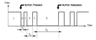
Figure 4-5 Waveform of Button Bounce
