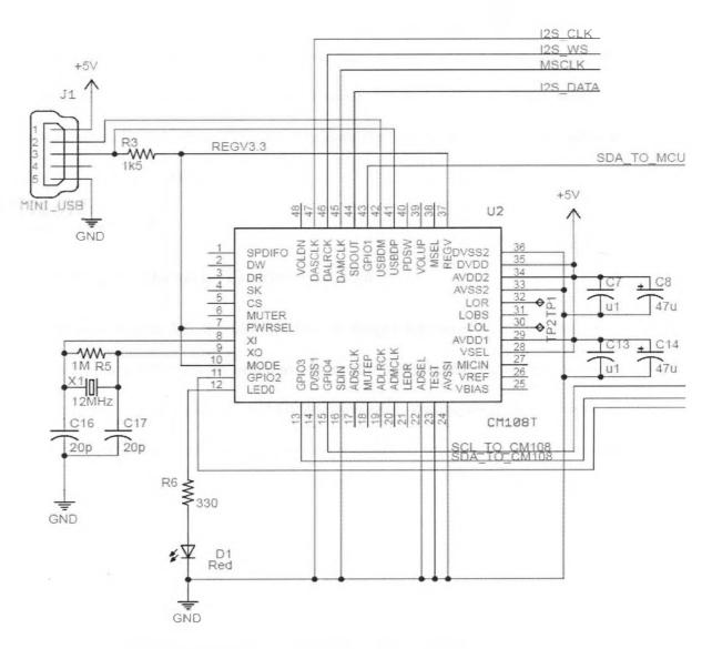
Figure 3-5 CM108 schematic in Wireless Transmitter
