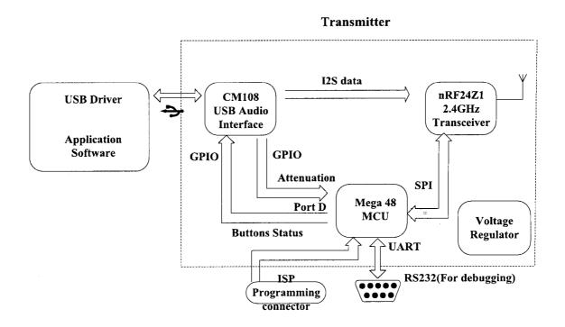
Figure 3-2 Transmitter Block Diagram
