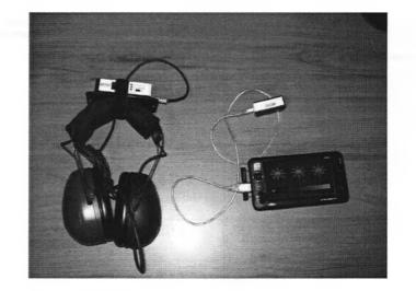
Figure 5-2 Headphones with Receiver and a Handheld PC Running Psychoacoustic Test Software
