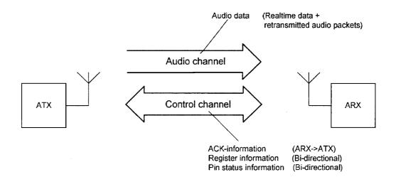
Figure 3-14 nRF24Z1 Communication Channel Principle [29]
