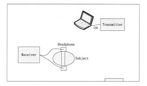
Figure 5-10 Experimental Set-up for Subjective Evaluation
