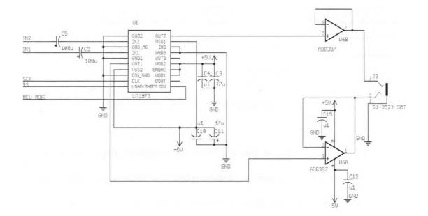
Figure 3-9 LM1973 and Unity-gain Buffer Schematic
