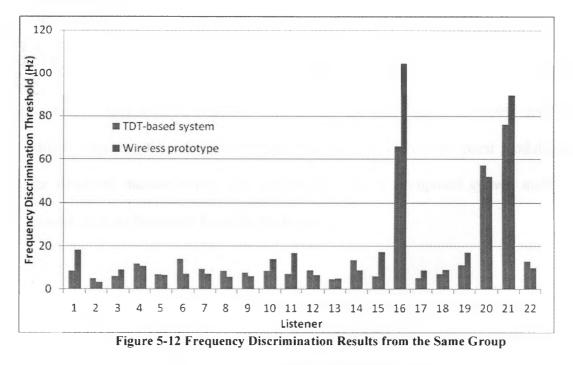
of Listeners with the TDT and the Wireless Prototype
