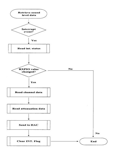
Figure 4-13 Flowchart of Retrieving and Sending Attenuation Data
