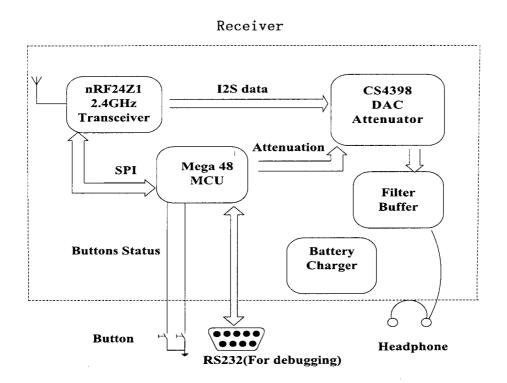
Figure 3-3 Receiver Block Diagram
