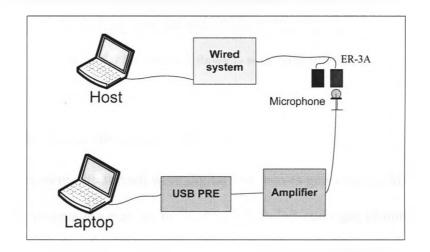
Figure 5-6 Experimental Set-up of Wired System
