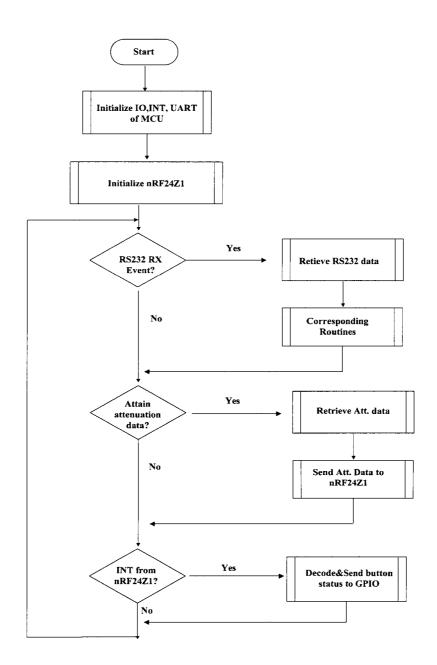
Figure 4-7 Main Flowchart of Transmitter
