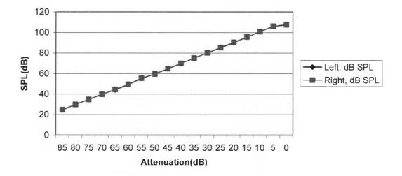
Figure 5-9 SPLs from 1 kHz Tone with Different Attenuation
