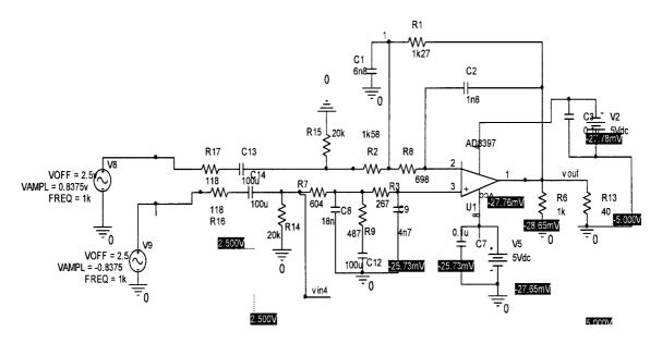
Figure 3-23 Schematic of DAC Output Amplifier for Simulation
