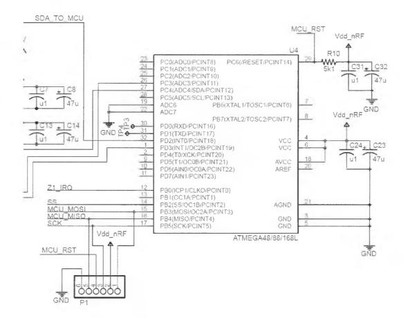
Figure 3-7 Mega48 Schematic in Transmitter
