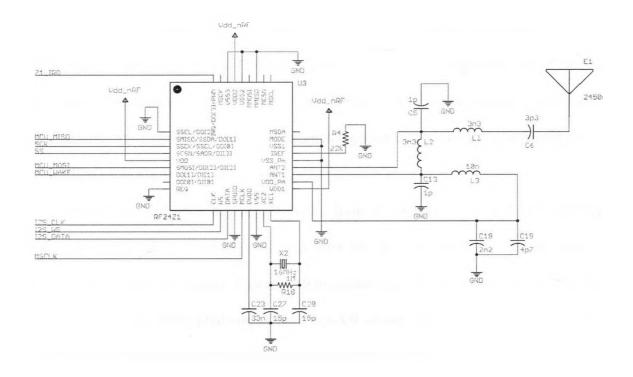
Figure 3-18 nRF24Z1 Schematic in Receiver
