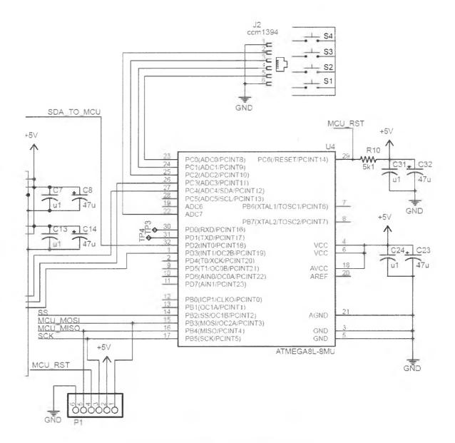
Figure 3-6 Mega8 Schematic in Wired System
