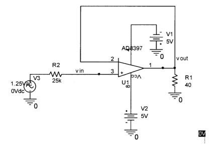
Figure 3-11 Schematic of AD8397 for Simulation (Assuming Vrms is 1.25v)
