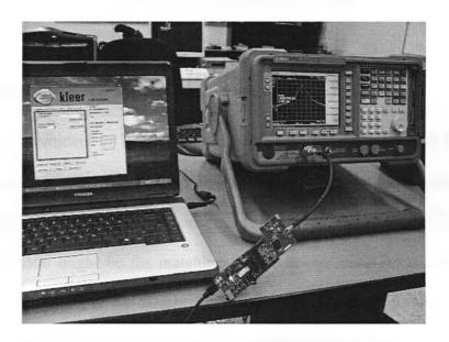
Figure 5-5 Measurement Set-up of Kleer Wireless Audio System
