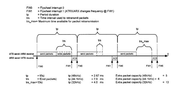
Figure 3-15 nRF24Z1 Data Streaming Principle [29]
