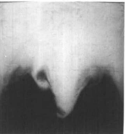
Figure 7. Spread of dyed source fluid in a fully spun-up flow, for both southwestern (left) and northwestern (right) sources. The top photographs correspond to 143 rotations, the center to 430 rotations and the bottom to 783 rotations after the source was dyed. The conditions of the experiment are listed in Table 1.
