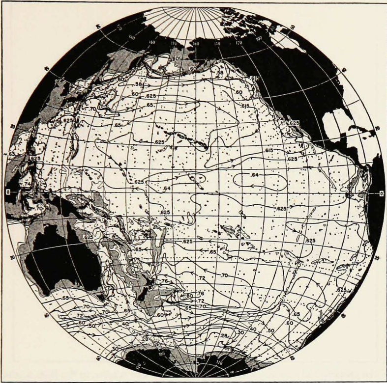
Figure 2. The geopotential anomaly at the 1000-decibar surface relative to the 2000-decibar surface, in dynamic meters ( 10 \text{ m}^2/\text{sec}^2 or 10 \text{ J/kg} ). In the shaded areas the ocean depth is less than 2000 m, and the light line is the 3000-m depth contour.
