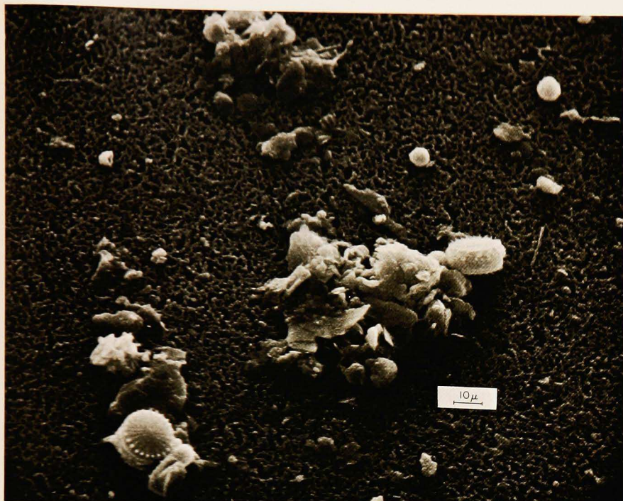
Figure 2. Scanning electron micrographs of samples of suspended matter collected in the upper Chesapeake Bay with the sampler. All samples were collected, freeze-dried, and photographed on silver-membrane filters. Note the good preservation of weakly bound composite particles (agglomerates) and fragile organisms. See also Fig. 3.
