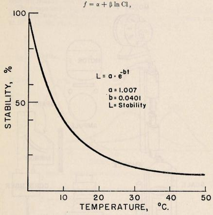
Figure 2. The relation between stability and temperature.
