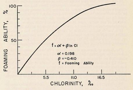
Figure 1. The relation between foaming and chlorinity.
