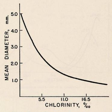
Figure 5. The relation between a mean diameter and chlorinity.
