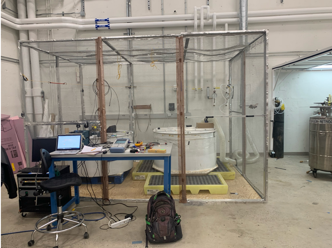
Figure 4.6: A custom Faraday cage built around the Y-factor measurement system. The cage was constructed for RFI mitigation, and demonstrations show it provides 20dB of attenuation for unwanted signals. The system is built from T-slot material and contains two doors, one on the side of filling and the other at the front for personnel access. The personnel door is embedded within a larger door, sized to enable the cylinders to be removed. The cage additionally serves as an extra safety barrier between the nitrogen bath and spectators in the lab, and the structure provides a convenient way to support cables and relieve cable strain.
