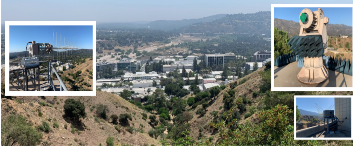
Figure 3.5: The Mesa Antenna Range at Jet Propulsion Laboratory in Pasadena, CA. The background photograph is the canyon which sits beneath the signal path, and the outlined photographs are the transmitter yagi antenna (left), the range mount and antenna under test (upper right), and the reference antenna (lower right).
