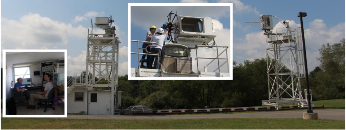
Figure 3.7: An antenna range at Green Bank Radio Observatory. Inlaid photos include (1) the measurement control room and (2) mounting the antenna under test, in this case a biconical antenna attached to a drone.
