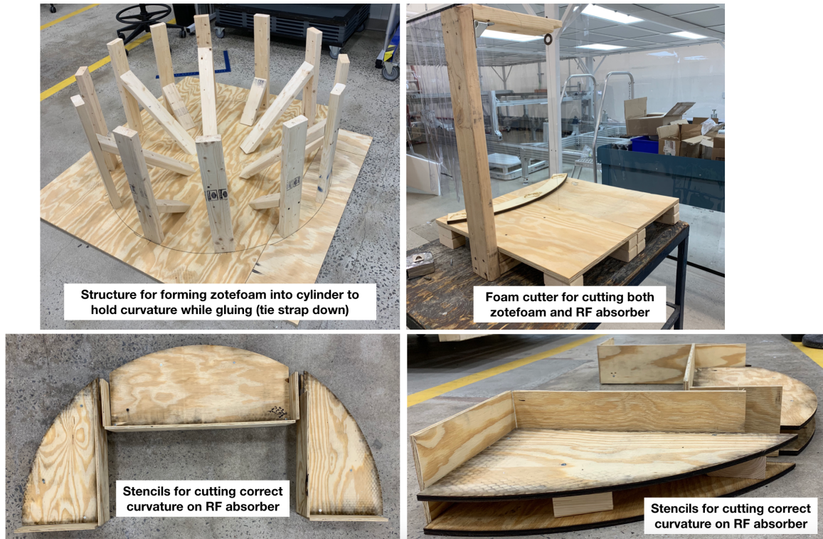
Figure 4.4: Various woodworking projects aid with the construction of the y-factor measurement system.
