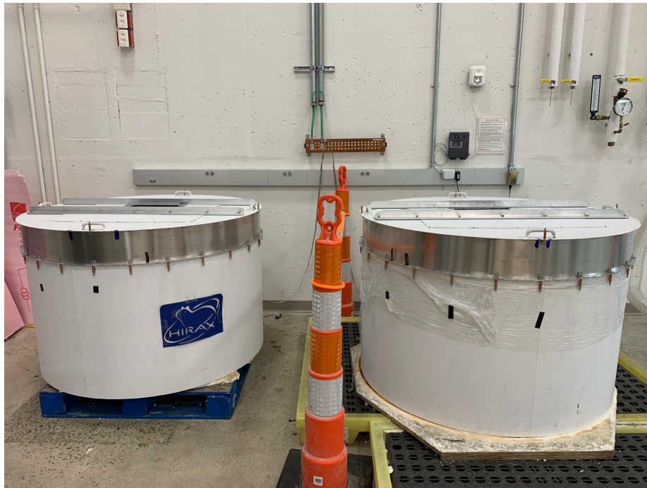
Figure 4.23: Cavity extenders of 6inches in length were constructed for the Y-factor system, in order to evaluate the impact of reflections and provide the capability to measure larger antennas.
