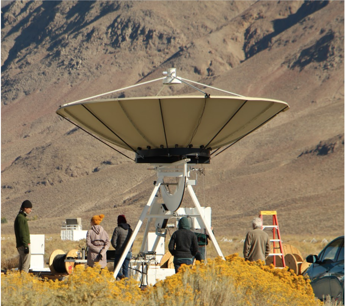
Figure 6.2: Photo of the DSA-110 dish mapped by the drone calibrator.
