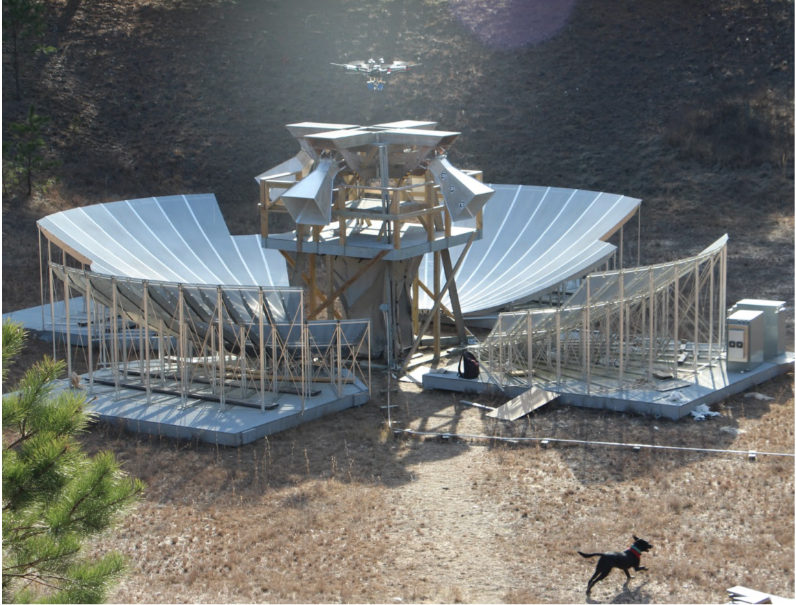
Figure 6.6: The Baryon Mapping eXperiment (BMX). BMX is comprised of four 4m off-axis dishes, and operates in a frequency range 1100-1500MHz. The drone system made 2D beam maps of the four BMX dishes in March 2020.
