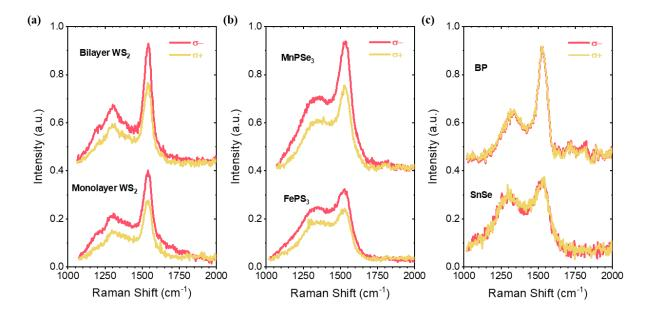
**Fig 2.1.14** Helicity-resolved Raman spectra of strong-coupled (a) monolayer  $WS_2/SiO_2$  and bilayer  $WS_2/SiO_2$  heterostructures, (b)  $FePS_3/SiO_2$  and  $MnPSe_3/SiO_2$  heterostructures, and (c)  $SnSe/SiO_2$  and  $BP/SiO_2$  heterostructures under  $\sigma$ + excitation with photon energy of 2.33 eV. All panels: from ref. (126).
