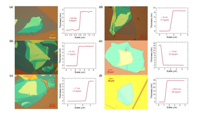
**Fig 3.1.12** Optical image and detailed AFM analysis of BP with different layer number of (a) 8 layers, (b) 11 layers, (c) 13 layers, (d) 17 layers, (e) 33 layers, (f) 58 layers. All panels: from ref. (129).
