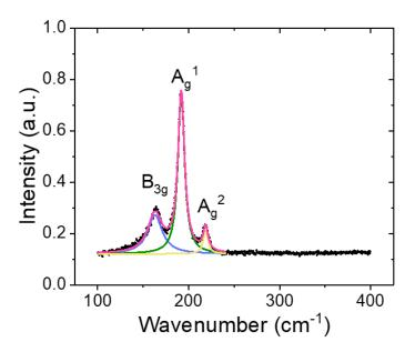
**Fig 2.3.3** Raman scattering spectra of the SnS sample. The Lorentz fitting curves of  $B_{3g}$ ,  $A_{g1}$  and  $A_{g2}$  mode are shown by blue, green and yellow lines, respectively. All panels: from ref. (128).
