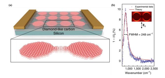
**Fig 1.6** (a) The schematic image of the graphene-disk plasmonic resonator device. The graphene nanodisks are connected by quasi-1D graphene nanoribbons. Adapted with permission from ref. (99) Copyright 2018, Springer Nature. (b) Infrared extinction spectrum of the graphene-disk plasmonic resonator with excitation polarization perpendicular to nanoribbons. Adapted with permission from ref. (99) Copyright 2018, Springer Nature.
