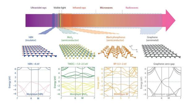
**Fig 1.1** Electromagnetic spectrum from ultraviolet rays to radiowaves covered by representative 2D materials (hBN, TMDs, BP and graphene) with their atomic structure, bandgap and band structure. Adapted with permission from ref. (19) Copyright 2014, Springer Nature.
