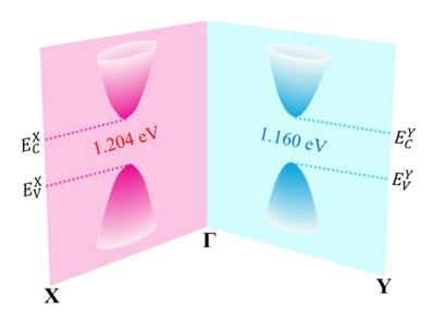
Fig 2.3.6 Schematic illustration of the band structure of layered SnS. All panels: from ref. (128).
