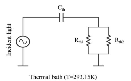
Fig 3.2.14 The schematic of thermal speed calculation. All panels: from ref. (131).
