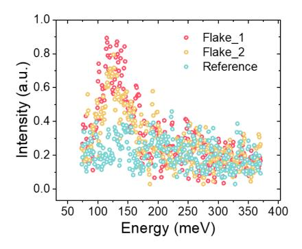
Fig 4.2.8 PL spectra from the Te flake and SiO<sub>2</sub>/Si substrate .
