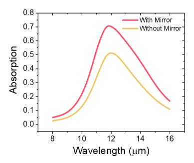
Fig 3.2.20 The simulated absorption spectrum of the bolometer with/without the gold back mirror.
