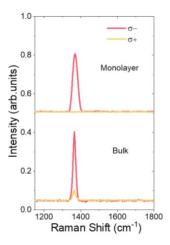
**Fig 2.2.10** Helicity-resolved Raman spectra of monolayer and bulk hBN under  $\sigma$ + excitation with photon energy of 2.33 eV. All panels: from ref. (127).
