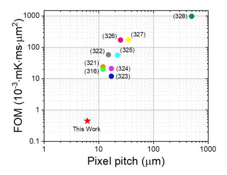
**Fig 3.2.19** The FOM of our bolometer device in comparison with the values reported in previous literatures. Here, the NETD has been normalized with the noise bandwidth of 1 Hz. All panels: from ref. (131).
