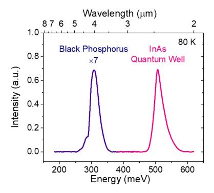
**Fig 3.1.9** The PL emission spectra of thin-film BP and the InAs quantum well (The PL intensity of BP is multiplied by a factor of 7). All panels: from ref. (129).
