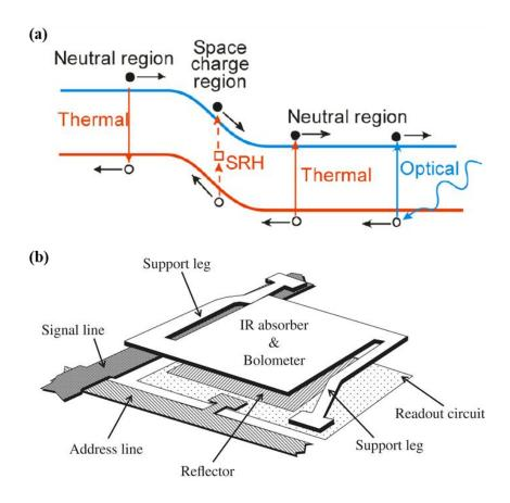
**Fig 1.8 (a)** The schematic illustration of the working mechanism of a p-n photodiode. Adapted with permission from ref. (116) Copyright 2016, IOP Publishing Ltd. (b) The schematic image of a typical microbolometer structure. Adapted with permission from ref. (123) Copyright 2017, Institute of Electrical Engineers of Japan. Published by John Wiley & Sons, Inc.
