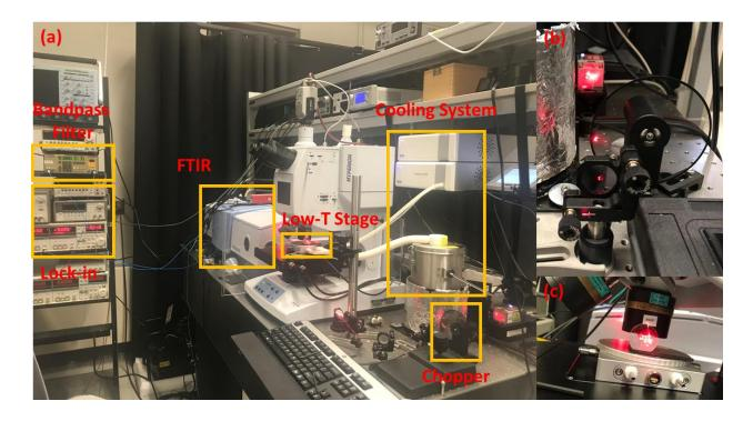
**Fig 3.1.1 (a)** An overall photo of the low-temperature mid-infrared PL measurement setup. **(b)** A close-up of the set-up at the mechanical chopper side. **(c)** A close-up of the set-up at the low-temperature sample stage side.
