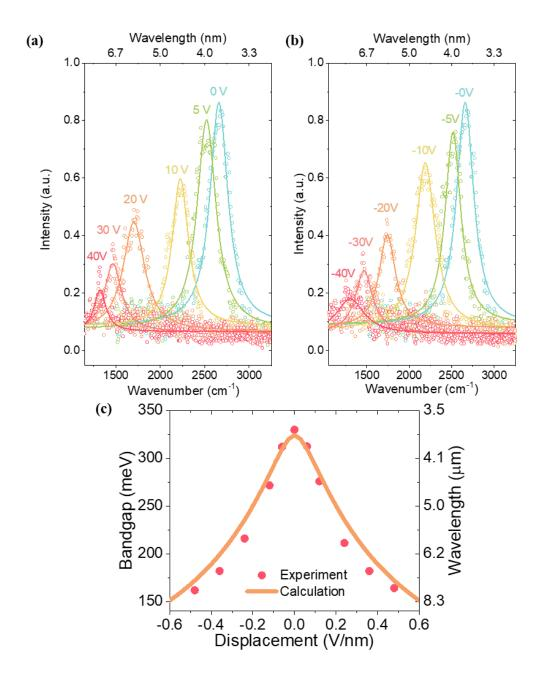
**Fig 3.1.15** The measured (dots) and fitted (lines) tunable PL spectra of the 20-layer BP device under different displacement fields (a) from 0 to 0.48 V/nm (b) from 0 to 0.48 V/nm. (c) The bandgap/wavelength tuning of the 20-layer BP extracted from PL spectra (dots) and first-principle based model calculations (line). All panels: from ref. (130).
