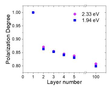
**Fig 2.2.7** Layer number dependence of polarization degree of Raman G mode in graphene flakes at excitation photon energy of 2.33 eV and 1.94 eV. All panels: from ref. (127).
