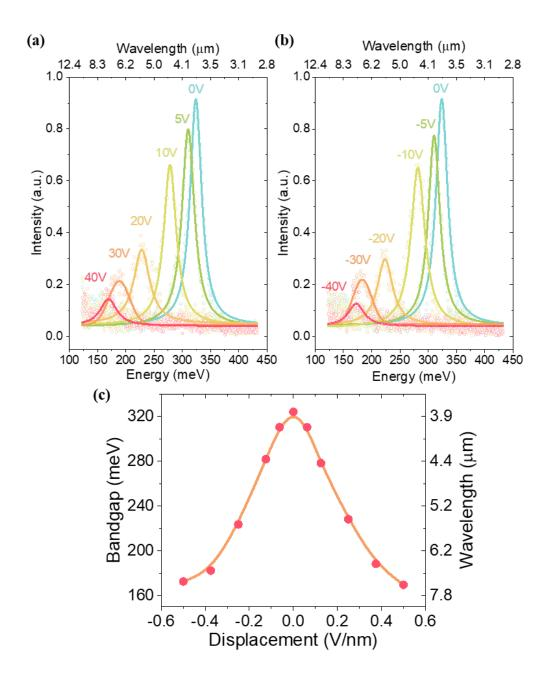
**Fig 3.1.16** The measured (dots) and fitted (lines) tunable PL spectra of the 23-layer BP device under different displacement fields (a) from 0 to 0.48 V/nm (b) from 0 to 0.48 V/nm. (c) The bandgap/wavelength tuning of the 20-layer BP extracted from PL spectra.
