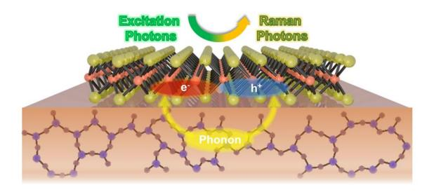
**Fig 2.1.12** Schematic of electron-phonon interaction and activation of optically-silent Raman modes in the 2D material/SiO<sub>2</sub> heterostructures. All panels: from ref. (126).
