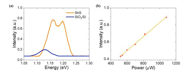
**Fig 2.3.5** (a) PL spectra from the SnS sample and SiO<sub>2</sub>/Si substrate. (b) Excitation power dependence of the SnS PL intensity. All panels: from ref. (128).
