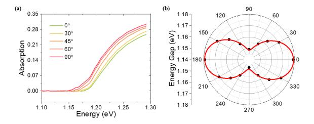
**Fig 2.3.12** (a) Absorption spectra of SnS at 77K under different illumination polarization. (b) Angular-resolved energy gap extracted from the absorption spectra. All panels: from ref. (128).
