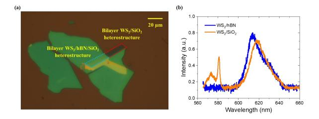
**Fig 2.1.10** (a) Optical micrograph of monolayer WS<sub>2</sub>/hBN/SiO<sub>2</sub> heterostructure. (b) Unpolarized emission spectra of bilayer WS<sub>2</sub>/hBN/SiO<sub>2</sub> heterostructure and bilayer WS<sub>2</sub>/SiO<sub>2</sub> heterostructure after 30 minutes annealing. All panels: from ref. (126).
