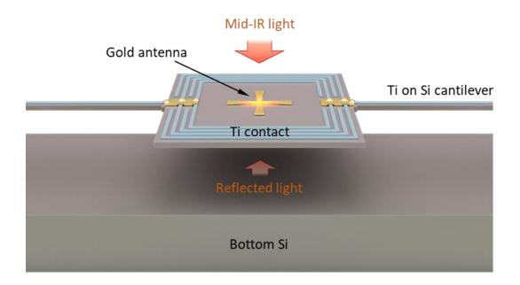
**Fig 3.2.1** The schematic of the silicon nanomembrane microbolometer device. All panels: from ref. (131).
