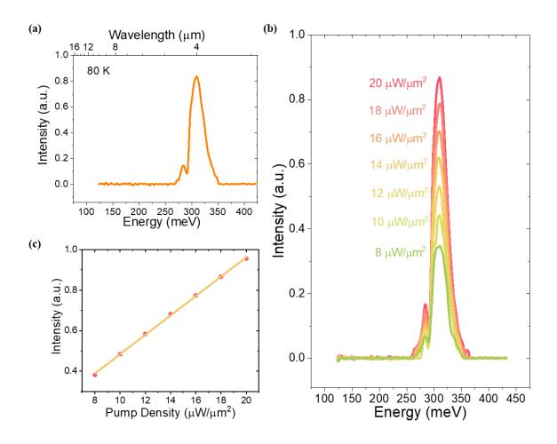
**Fig 3.1.7** (a) Mid-infrared PL spectrum of the 46-nm thick BP at 80 K. (b) Excitation power dependence of the PL spectrum of the 46-nm thick BP. (c) The measured (dots) and fitted (line) power dependence of the BP PL peak intensity. All panels: from ref. (129).
