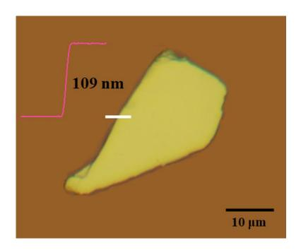
Fig 2.3.2 Optical micrograph of a typical SnS flake on 285 nm  $SiO_2/Si$ . Insert: The atomic force microscopy scan performed on the SnS flake. Its thickness is determined to be 109 nm. All panels: from ref. (128).
