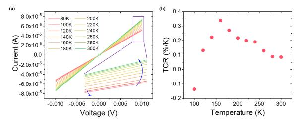
**Fig 4.2.5** (a) The temperature dependent I-V characteristics of the graphite nanoribbon array device. The insert: detailed I-V characteristics at bias voltage near 0.01 V. (b) The calculated temperature dependence of TCR.
