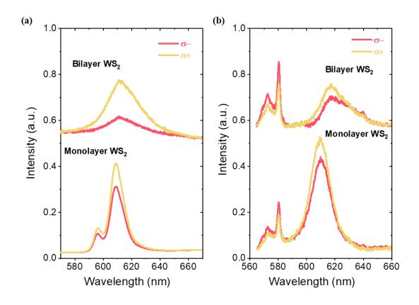
**Fig 2.1.18** The helicity-resolved emission spectra from monolayer  $WS_2/SiO_2$  and bilayer  $WS_2/SiO_2$  heterostructures (a) before and (b) after 30 min annealing process under  $\sigma$ + excitation with photon energy of 2.33 eV. All panels: from ref. (126).
