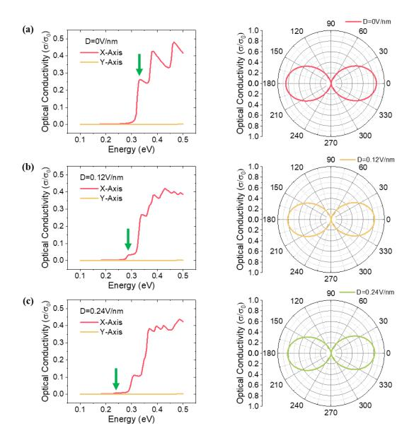
**Fig 3.1.22** The anisotropic low-energy optical conductivity spectrum (left) and angular-resolved optical conductivity at the first peak (See the green arrows in the left panel) of the spectrum (right) of the 20-layer BP under the displacement field of (a) 0, (b) 0.12 and (c) 0.24 V/nm. All panels: from ref. (130).
