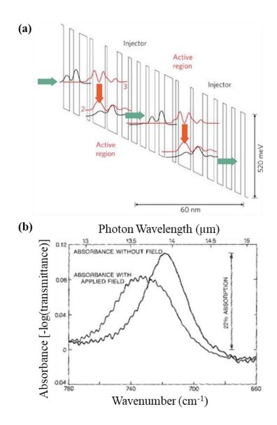
**Fig 1.7** (a) The schematic image of intersubband laser transition in the conduction band of a typical MQW structure. Adapted with permission from ref. (111) Copyright 2012, Springer Nature. (b) Infrared absorbance spectrum of a GaAs QW structure with/without an external electric field of 36 kV/cm. Adapted with permission from ref. (115) Copyright 1987, AIP Publishing.
