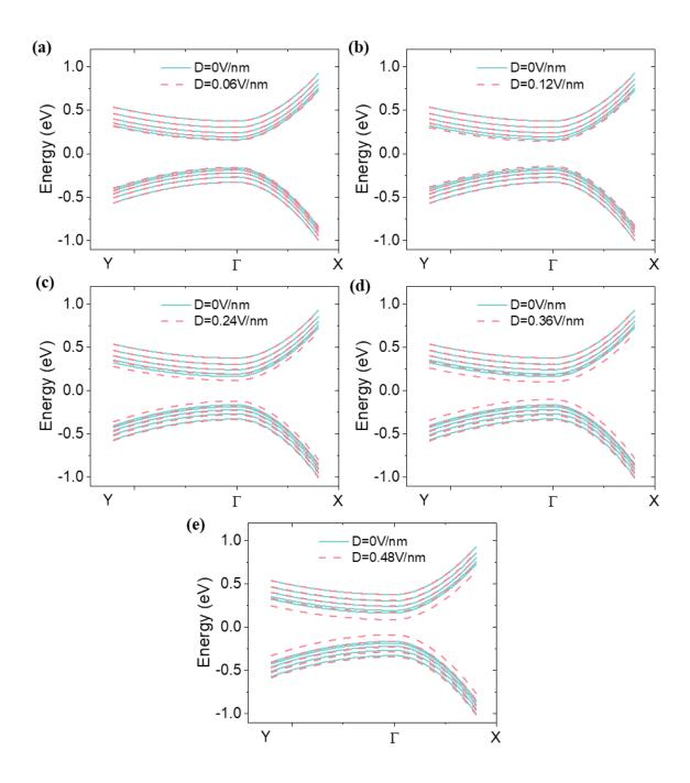
**Fig 3.1.17** The bands of the 20-layer BP near the  $\Gamma$  point at displacement field of (a) 0.06V/nm, (b) 0.12 V/nm, (c) 0.24 V/nm, (d) 0.36 V/nm, (e) 0.48 V/nm, in comparison with those of the intrinsic 20-layer BP. Only 5 highest valance and 5 lowest conduction bands are plotted for simplicity. All panels: from ref. (130).
