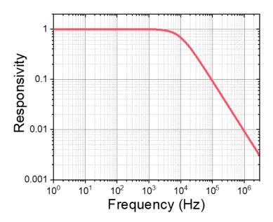
**Fig 3.2.15** Calculated modulation frequency dependence of the responsivity. All panels: from ref. (131).
