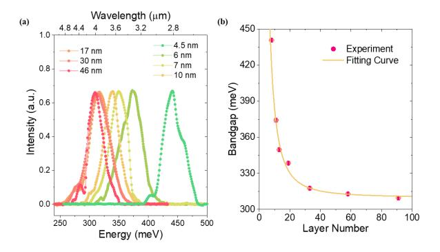
**Fig 3.1.13** (a) Thickness dependence of the PL spectra of BP. (b) Thickness dependence of BP bandgap in mid-infrared. An error bar of  $\pm 1$  layer is added to the layer number axis. All panels: from ref. (129).
