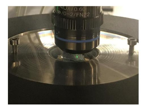
Fig 2.1.7 A photo of the sample mounted in Janis ST-500 Microscopy Cryostat.
