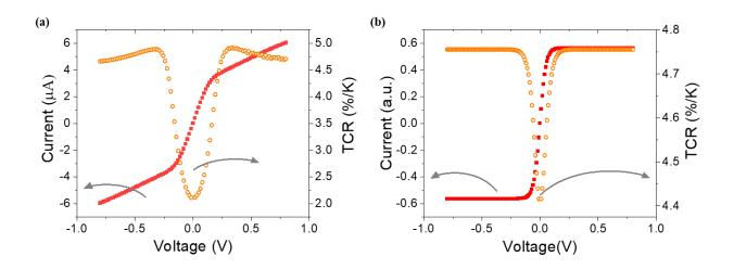
**Fig 3.2.8** The **(a)** measured and **(b)** calculated I-V characteristics and TCR of the bolometer device as a function of the bias voltage. All panels: from ref. (131).
