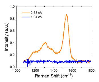
**Fig 2.1.11** Unpolarized Raman spectra of monolayer WS<sub>2</sub>/SiO<sub>2</sub> heterostructure under excitation photon energy of 2.33 eV and 1.94 eV. All panels: from ref. (126).
