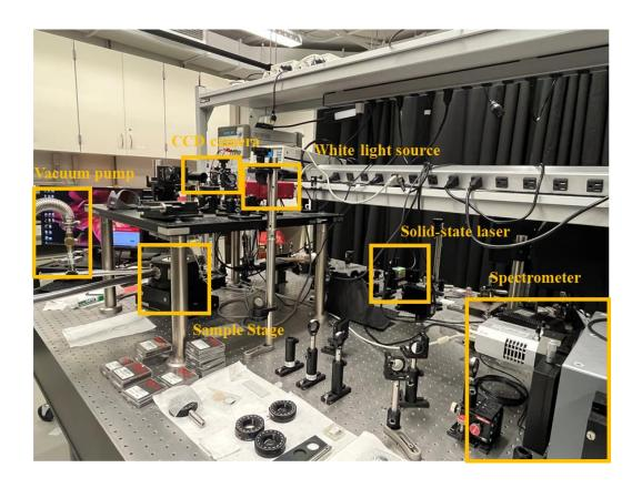
Fig 2.1.3 A photo of the home-made low-temperature micro-Raman/PL measurement system.
