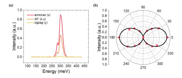
**Fig 3.1.10 (a)** Polarization-resolved PL spectra of 46-nm thick BP along x- (red), x-y (orange, 45 degrees to x and y) and y- (yellow) directions. **(b)** The measured (dots) and fitted (line) angular-resolved PL peak intensity of BP. All panels: from ref. (129).
