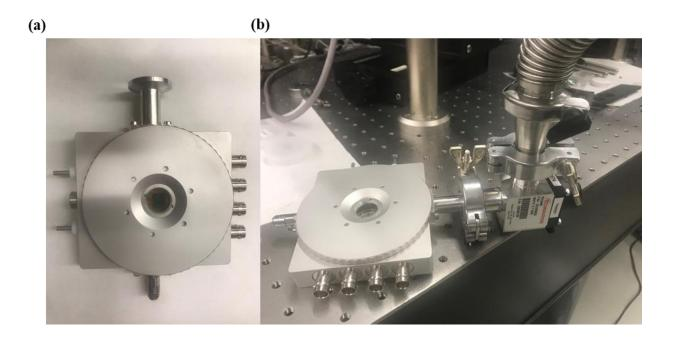
Fig 3.2.9 (a) A photo of vacuum chamber sample stage. (b) A photo of vacuum pumping system.
