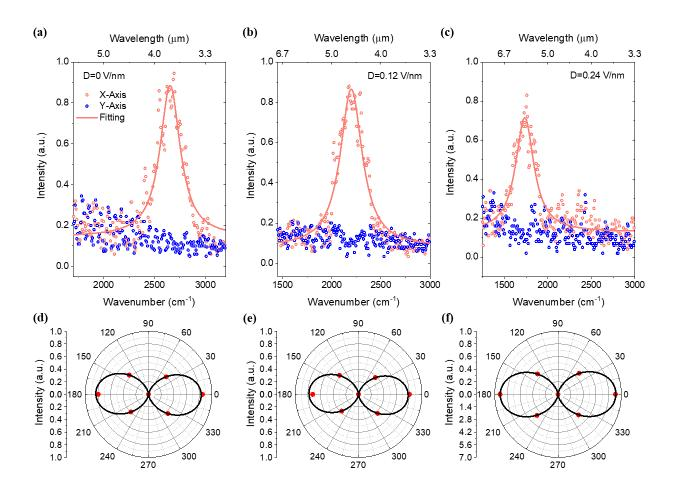
**Fig 3.1.21 Upper panel:** The PL spectra of the 20-layer BP measured along x- and y-directions of the crystal at the displacement field of (a) 0 V/nm, (b) 0.12 V/nm, (c) 0.24 V/nm. **Lower Panel:** The measured (dots) and fitted (line) angular-resolved PL intensity of the 20-layer BP at the displacement field of (d) 0 V/nm, (e) 0.12 V/nm, (f) 0.24 V/nm. All panels: from ref. (130).
