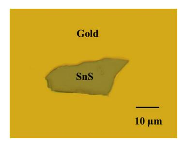
**Fig 2.3.10** Optical micrograph of SnS flake exfoliated on gold film/SiO<sub>2</sub>/Si substrate. All panels: from ref. (128).
