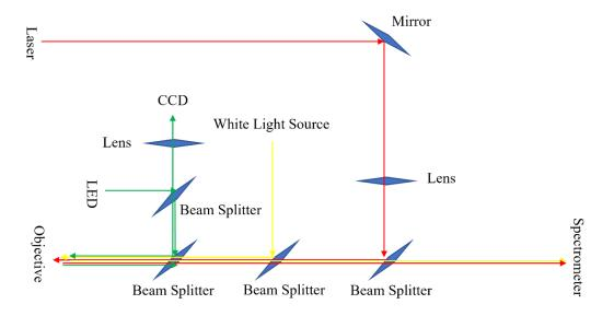
**Fig 2.1.4** Schematic illustration of the optical measurement system. Red line: Optical path for Raman and PL measurement. Yellow line: Optical path for absorption measurement. Green line: Optical path for sample illumination and imaging.
