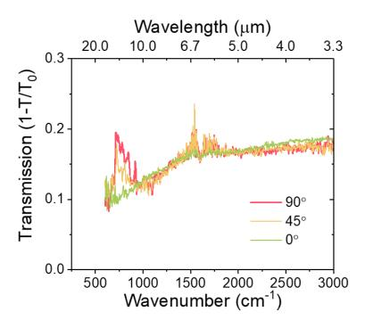
**Fig 4.2.2** The linearly-polarized infrared extinction spectra of the graphite nanoribbon array. The red (green) curve shows the spectra for incident light polarization perpendicular (parallel) to graphite nanoribbon direction.
