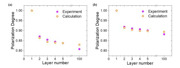
**Fig 2.2.9** The layer number dependent polarization degree of graphene Raman G mode from Raman tensor calculation compared with the experimental results (**a**) at room temperature and (**b**) at 77K. All panels: from ref. (127).
