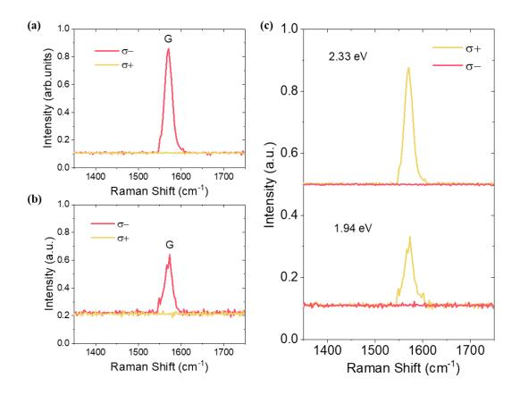
**Fig 2.2.3** Helicity-resolved Raman spectra of Raman G mode in monolayer graphene under (a)  $\sigma$ + excitation with photon energy of 2.33 eV (b)  $\sigma$ + excitation with photon energy of 1.94 eV (c)  $\sigma$ - excitation. All panels: from ref. (127).
