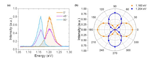
**Fig 2.3.8** (a) PL spectra of SnS under different detection polarization. (b) Angular-resolved PL intensity of the 1.204 eV (yellow) and 1.160 eV (blue) emission peaks under different detection polarization. The fitting curves for PL emissions from Γ-X and Γ-Y valley are indicated by yellow and blue lines, respectively. All panels: from ref. (128).
