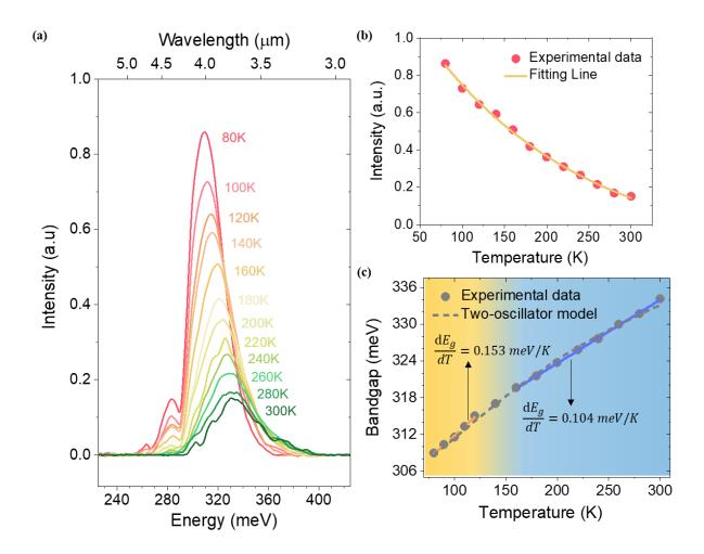
**Fig 3.1.11** (a) Temperature dependence of the PL spectrum of the 46-nm thick BP. (b) Temperature dependence of the BP PL peak intensity. (c) Temperature-dependent bandgap of BP extracted from the PL peak position. All panels: from ref. (129).
