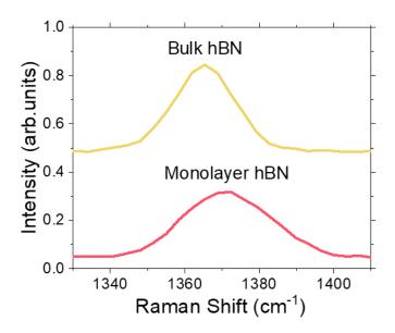
Fig 2.2.2 Unpolarized Raman spectra of monolayer and bulk hBN. All panels: from ref. (127).
