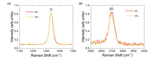
Fig 2.2.4 Helicity-resolved Raman spectra of Raman (a) D and (b) 2D modes in monolayer graphene under  $\sigma$ + excitation with photon energy of 2.33 eV. All panels: from ref. (127).
