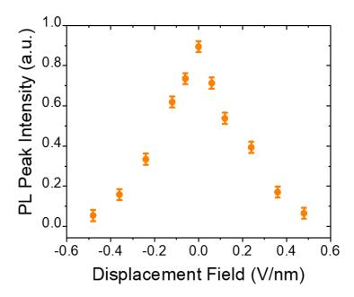
**Fig 3.1.18** The PL intensity extracted from PL spectra as the function of displacement field. All panels: from ref. (130).
