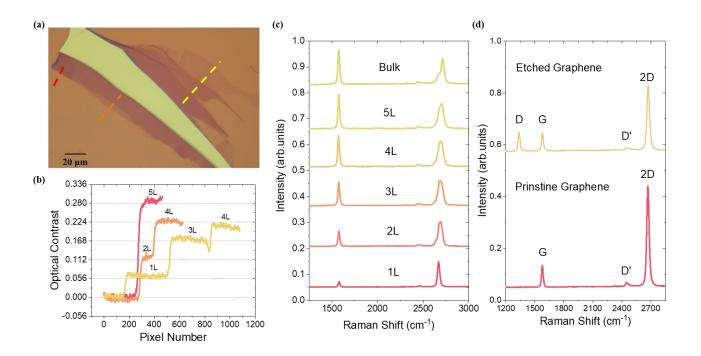
**Fig 2.2.1** (a) Optical micrograph of graphene flakes. (b) Optical contrast of graphene flakes measured along the lines in (a). (c) Unpolarized Raman spectra of few-layer (1L to 5L) and thin-film (>100L) graphite. (d) Unpolarized Raman spectra of etched monolayer graphene and pristine monolayer graphene. All panels: from ref. (127).
