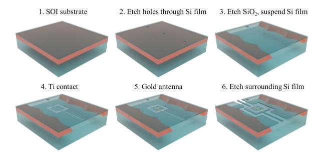
Fig 3.2.6 The schematic of process flow of the device fabrication. All panels: from ref. (131).
