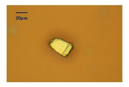
Fig 4.2.6 Optical image of a Te flake on a 285-nm SiO<sub>2</sub>/Si substrate.
