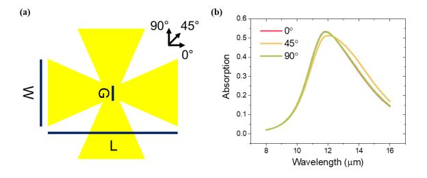
**Fig 3.2.2** (a) The schematic of the cross-diabolo antenna. (b) The simulated absorption spectrum of the bolometer under different excitation polarizations. All panels: from ref. (131).
