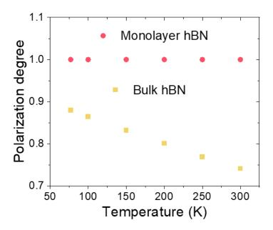
**Fig 2.2.11** Temperature dependence of polarization degree of Raman  $E_{2g}$  mode in monolayer and bulk hBN. All panels: from ref. (127).
