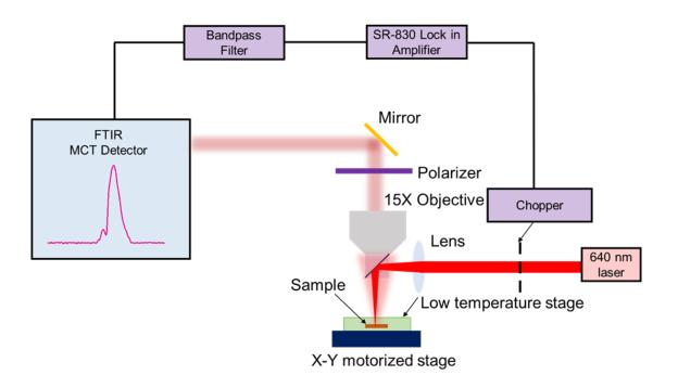
Fig 3.1.2 Schematic illustration of the mid-infrared PL measurement setup. All panels: from ref. (129).
