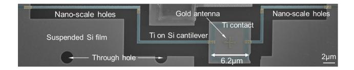
**Fig 3.2.17** A SEM (false color) micrograph of the bolometer device with nano-scale holes fabricated on its cantilevers. All panels: from ref. (131).
