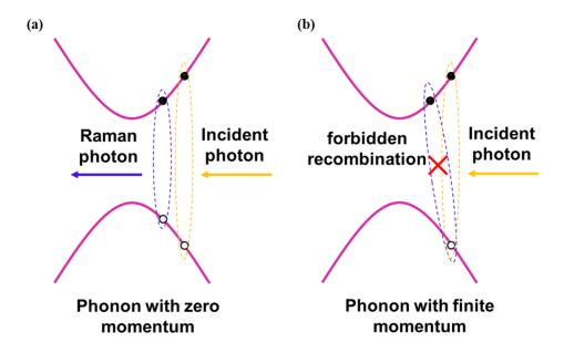
**Fig 2.1.13** Schematic of **(a)** allowed and **(b)** forbidden pathways for recombination of phonon coupled electron-hole pair. All panels: from ref. (126).
