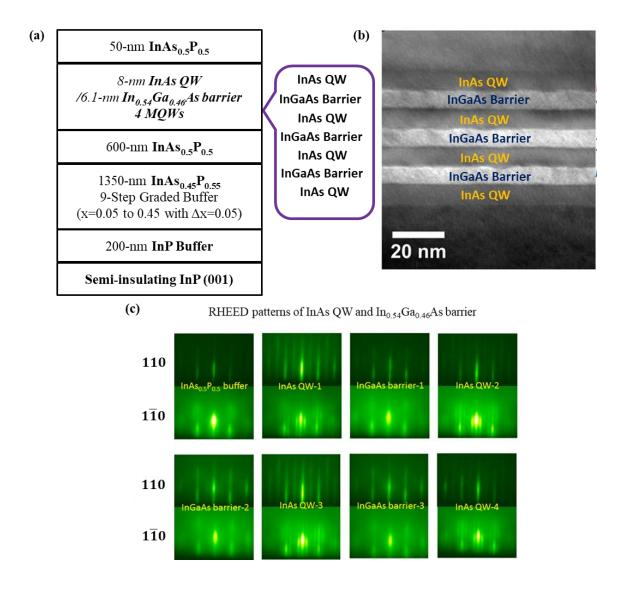
**Fig 3.1.8 (a)** Schematic structure of InAs MQW grown on indium phosphide (InP) substrate. **(b)** Cross-sectional transmission electron microscopy (X-TEM) of InAs QW/In<sub>0.54</sub>Ga<sub>0.46</sub>As barriers. **(c)** The Reflection high-energy electron diffraction (RHEED) patterns taken during the growth process. All panels: from ref. *(129)*.
