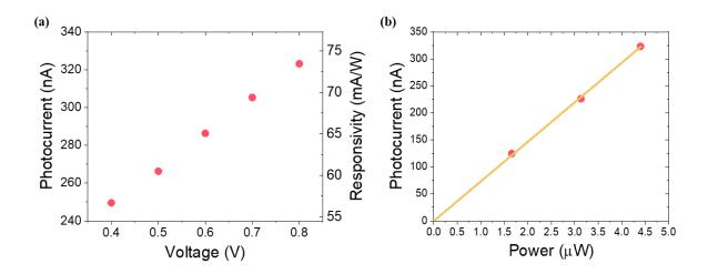
**Fig 3.2.10** (a) The measured photocurrent and corresponding responsivity of the bolometer device against the bias voltage. (b) Incident power dependence of the photocurrent. All panels: from ref. (131).
