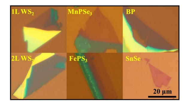
**Fig 2.1.2** Optical images of strong-coupled 2D materials/ $SiO_2$  heterostructures. Monolayer  $WS_2$ , bilayer  $WS_2$ , few-layer  $MnPSe_3$ ,  $FePS_3$ , BP and SnSe were used to construct heterostructures. All panels: from ref. (126).
