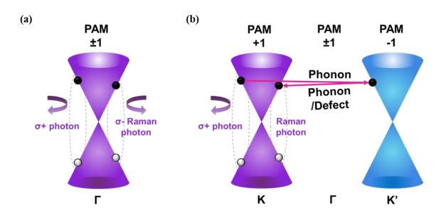
**Fig 2.2.5** Schematic illustration of the valley phonon scattering processes and corresponding variation of PAM for Raman (a) G, (b) D and 2D modes in monolayer graphene. All panels: from ref. (127).
