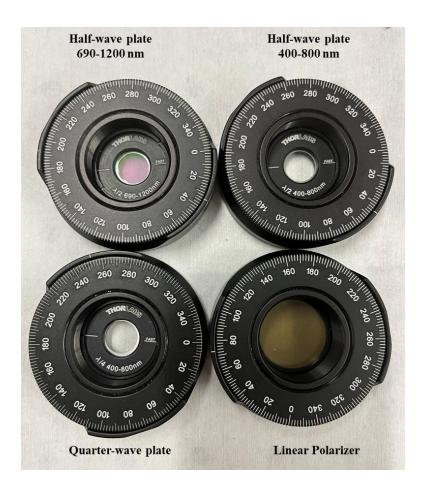
**Fig 2.1.5** A photo of broadband wave-plates and linear polarizers for polarization-resolved optical measurements.
