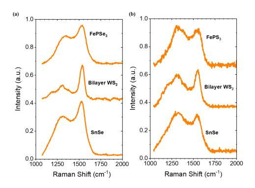
**Fig 2.1.8** Unpolarized Raman spectra of strong-coupled 2D material/ $SiO_2$  heterostructures with FePS<sub>3</sub>, bilayer WS<sub>2</sub> and SnSe as the 2D materials in heterostructures under excitation photon energy of (a) 2.33 and (b) 1.94 eV, respectively. All panels: from ref. (126).
