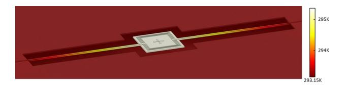
Fig 3.2.12 Simulated temperature elevation across the bolometer device. All panels: from ref. (131).
