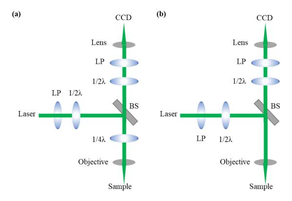
Fig 2.1.6 Schematic illustration of the (a) circularly and (b) linearly polarized optical measurements.
