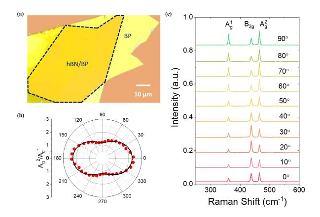
**Fig 3.1.4 (a)** Optical image of the hBN covered 46-nm thick BP flake on a 285-nm  $SiO_2/Si$  substrate. **(b)** Polarization-resolved Raman spectrum of the 46-nm thick BP. **(c)** The measured (dotes) and fitted (line) angular-resolved Raman intensity ratio of  $A_g^2$  and  $A_g^1$  mode. All panels: from ref. (129).
