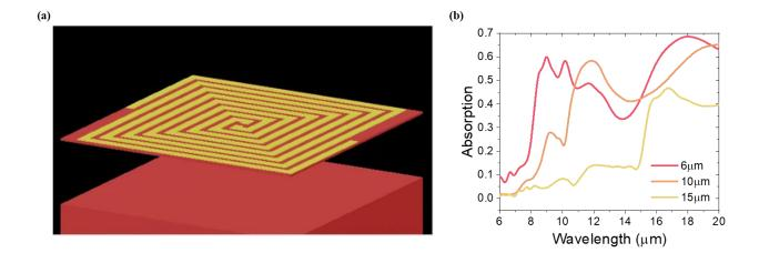
Fig 3.2.4 (a) The schematic of the spiral antenna. (b) The simulated absorption spectrum of the bolometer under different simulation period.
