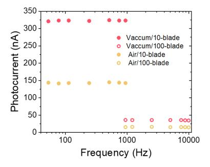
**Fig 3.2.16** Modulation frequency dependence of the photocurrent of the same device measured in air compared with that measured in vacuum from 50 Hz to 10 kHz.
