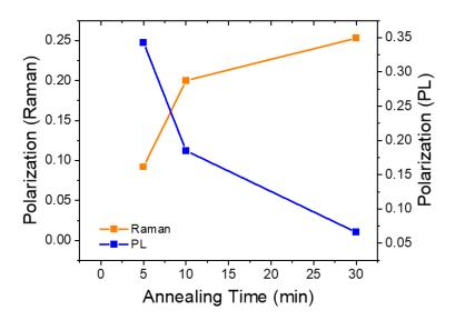
Fig 2.1.22 The polarization degree of Raman modes and PL in monolayer  $WS_2/SiO_2$  heterostructure versus the annealing time. All panels: from ref. (126).
