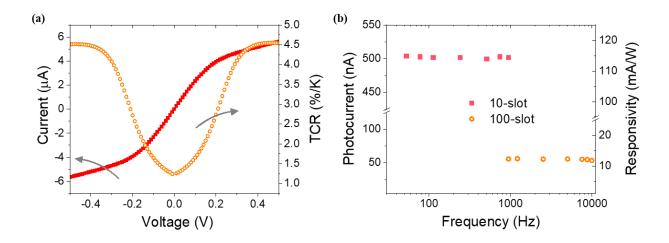
**Fig 3.2.18** (a) The I-V characteristics and the TCR of the bolometer device as a function of the bias voltage. (b) The measured photocurrent and corresponding responsivity as a function of the modulation frequency. All panels: from ref. (131).
