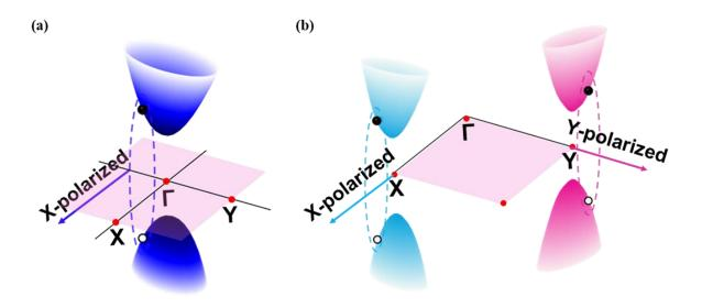
**Fig 2.1.17** Schematic illustration of band structure and corresponding optical selection rule in (a) BP and (b) SnSe. All panels: from ref. (126).
