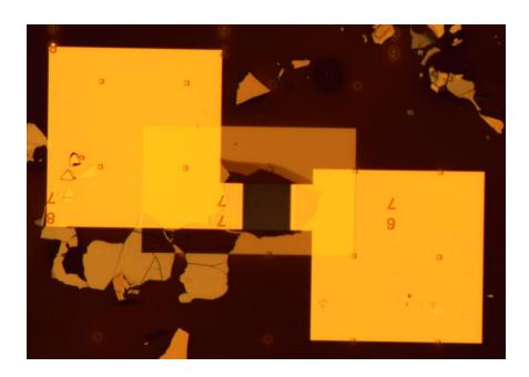
Fig 4.2.3 The optical image of the graphite nanoribbon array device for transport measurements.
