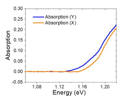
**Fig 2.3.13** Anisotropic absorption spectra of SnS along x- and y-polarization at room temperature. All panels: from ref. (128).
