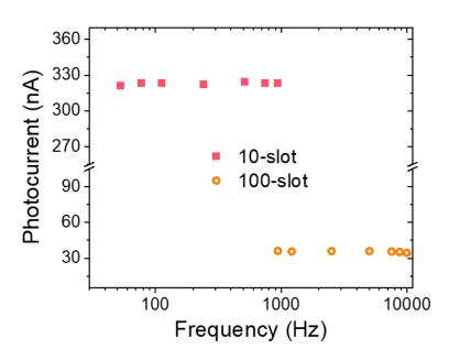
**Fig 3.2.13** Modulation frequency dependence of the photocurrent from 50 Hz to 10 kHz. All panels: from ref. (131).
