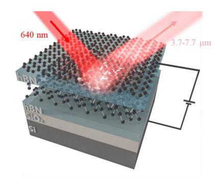
Fig 3.1.5 The schematic illustration of the dual-gate hBN/BP/hBN device. All panels: from ref. (130).
