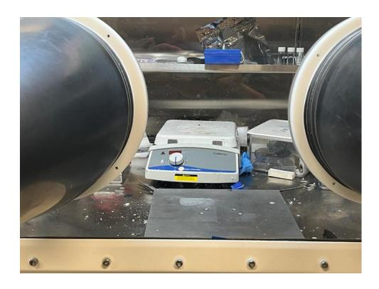
Fig 2.1.1 A photo of the hotplate in the glove box for sample annealing.
