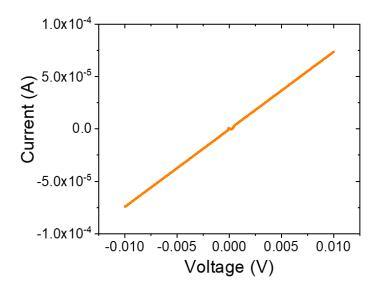
Fig 4.2.4 The I-V characteristics of the graphite nanoribbon array device at room temperature.
