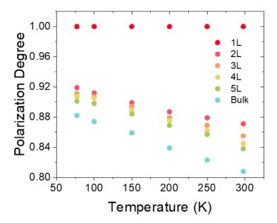
**Fig 2.2.8** Temperature dependence of polarization degree for Raman G mode in 1L-5L graphene and thin-film graphite. All panels: from ref. (127).
