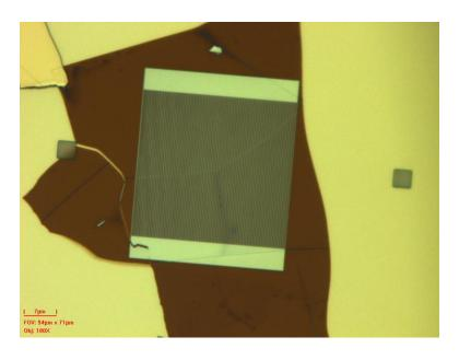
Fig 4.2.1 The optical image of the graphite nanoribbon array for infrared spectra measurements.
