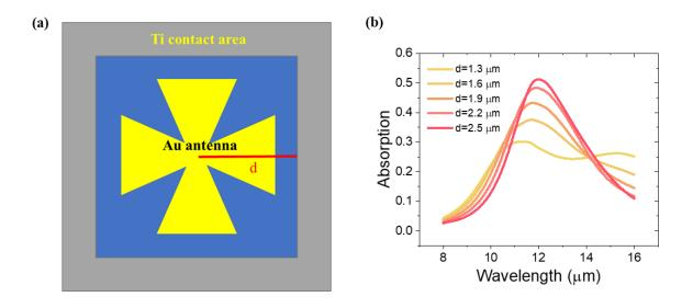
**Fig 3.2.5** (a) Schematic illustration of the distance between the center of the antenna to the boundary of the Ti contact, represented by d. (b) The dependence of the simulated absorption spectrum on distance d. All panels: from ref. (131).
