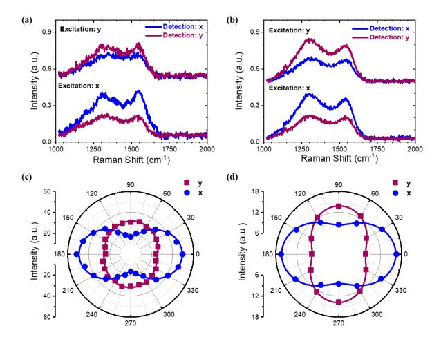
**Fig 2.1.16 Upper Panel:** The linearly polarized Raman spectra of strong-coupled (**a**) BP/SiO<sub>2</sub> and (**b**) SnSe/SiO<sub>2</sub> heterostructures under x-polarized and y-polarized excitation. **Lower Panel:** The angular resolved Raman intensity of strong-coupled (**c**) BP/SiO<sub>2</sub> and (**d**) SnSe/SiO<sub>2</sub> heterostructures under x-polarized and y-polarized excitations. All panels: from ref. (126).
