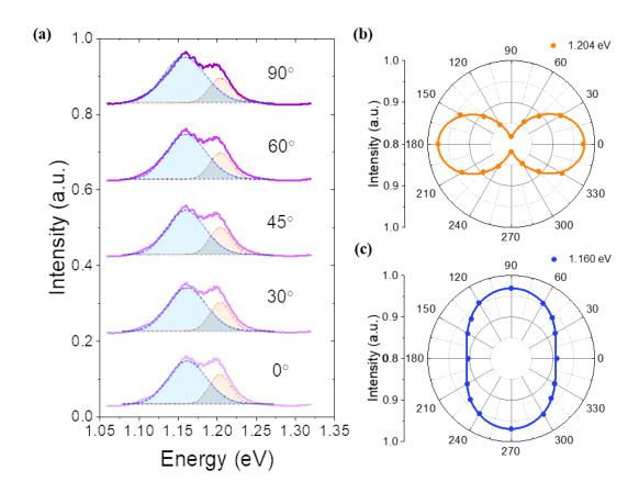
**Fig 2.3.7 (a)** PL spectra of SnS under different excitation polarization. **(b)** Angular-resolved PL intensity of the 1.204 eV (yellow) and 1.160 eV (blue) emission peaks under different excitation polarization. The fitting curves for PL emissions from Γ-X and Γ-Y valley are indicated by yellow and blue lines, respectively. All panels: from ref. (128).
