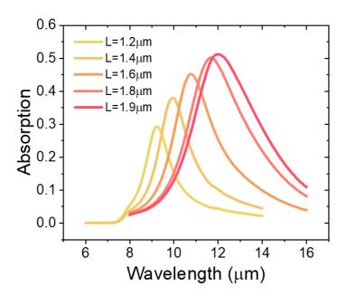
Fig 3.2.21 The simulated wavelength-tunable absorption spectrum of the bolometer with various antenna length.
