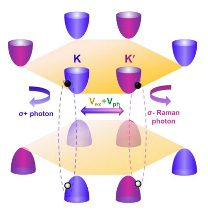
**Fig 2.1.20** Schematic of optical transition process for phonon-assisted excitonic intervalley scattering and the reversed helicity of Raman photons under broken  $C_3$  symmetry. All panels: from ref. (126).
