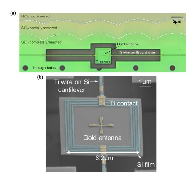
**Fig 3.2.7** (a) An optical micrograph of a fabricated bolometer device. (b) Scanning electron micrograph (false color) of the device's central area. All panels: from ref. (131).
