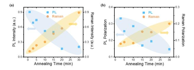
Fig 2.1.21 The (a) intensity and (b) polarization degree of the Raman modes and the PL in bilayer WS<sub>2</sub>/SiO<sub>2</sub> heterostructures versus the annealing time. All panels: from ref. (126).
