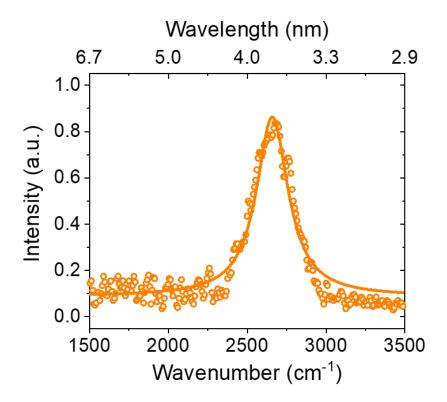
**Fig 3.1.14** The measured (dotted) and fitted (solid) PL spectrum of the 20-layer BP device at 83 Kelvin. All panels: from ref. (130).
