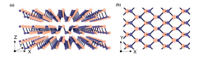
**Fig 2.3.1** Schematic illustration of the crystal structure of layered SnS. (left panel: front view of the x-z plane; right panel: top view of the x-y plane). All panels: from ref. (128).
