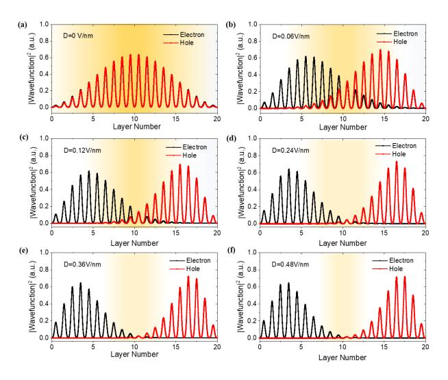
**Fig 3.1.19** The wavefunction distributions of the electron and hole states at  $\Gamma$  point of the 20-layer BP at displacements field of (a) 0V/nm, (b) 0.06 V/nm, (c) 0.12 V/nm, (d) 0.24 V/nm, (e) 0.36 V/nm, (f) 0.48 V/nm. The wavefunction overlapping is illustrated by background color, whose transparency increases as the overlapping decreases. All panels: from ref. (130).
