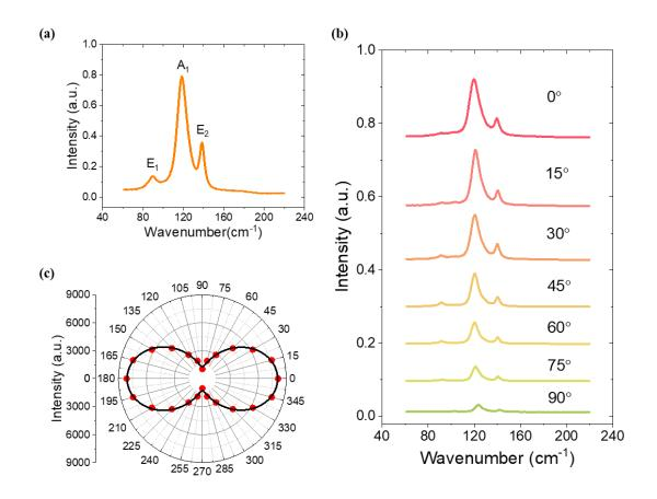
**Fig 4.2.7** (a) Raman scattering spectra of the Te flake. (b) Polarization-resolved Raman spectrum of the Te flake. (c) The measured (dotes) and fitted (line) angular-resolved Raman intensity of  $A_1$  mode.
