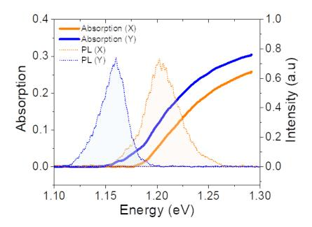
Fig 2.3.11 Anisotropic absorption spectra of SnS along x- and y-polarized illumination at 77K and its comparison with PL spectra. All panels: from ref. (128).
