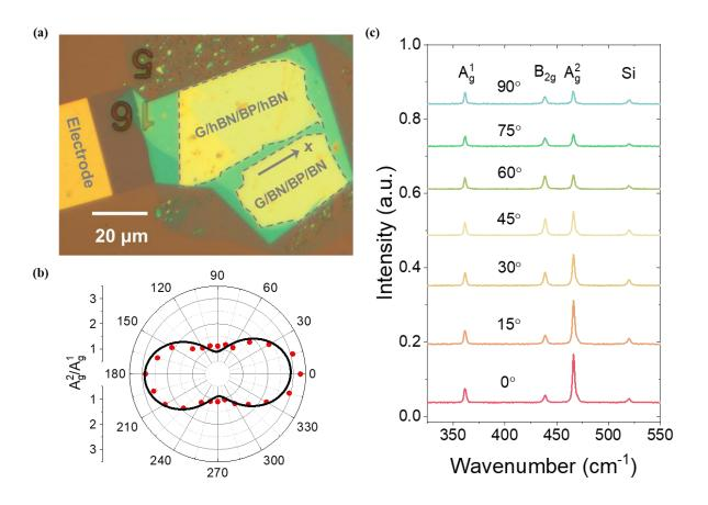
**Fig 3.1.6** (a) Optical micrograph of the dual-gate hBN/BP/hBN device with CVD graphene as the top-gate. (b) Polarization-resolved Raman spectrum of the 10.5-nm thick BP. (c) The measured (dots) and fitted (line) angular-resolved Raman intensity ratio of  $A_g^2$  and  $A_g^1$  mode. All panels: from ref. (130).
