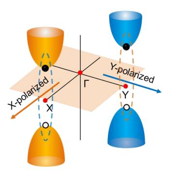
**Fig 2.3.9** Schematic illustration of the optical selective rule of the band edge emission. All panels: from ref. (128).
