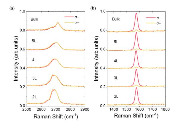
**Fig 2.2.6** Helicity-resolved Raman spectra of Raman (a) 2D and (b) G modes in 2L-5L graphene and thin-film (>100L) graphite under  $\sigma$ + excitation with photon energy of 2.33 eV. All panels: from ref. (127).
