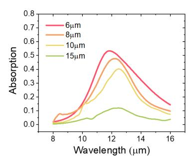
Fig 3.2.3 The simulated absorption spectrum of the bolometer under different simulation period.
