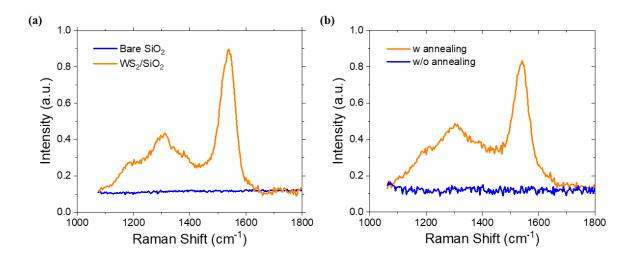
**Fig 2.1.9** (a) Unpolarized Raman spectrum of isolated SiO<sub>2</sub>/Si substrate and monolayer WS<sub>2</sub>/SiO<sub>2</sub>/Si heterostructure after annealing. (b) Unpolarized Raman spectrum of bilayer WS<sub>2</sub>/SiO<sub>2</sub> heterostructure before and after thermal annealing process. All panels: from ref. (126).
