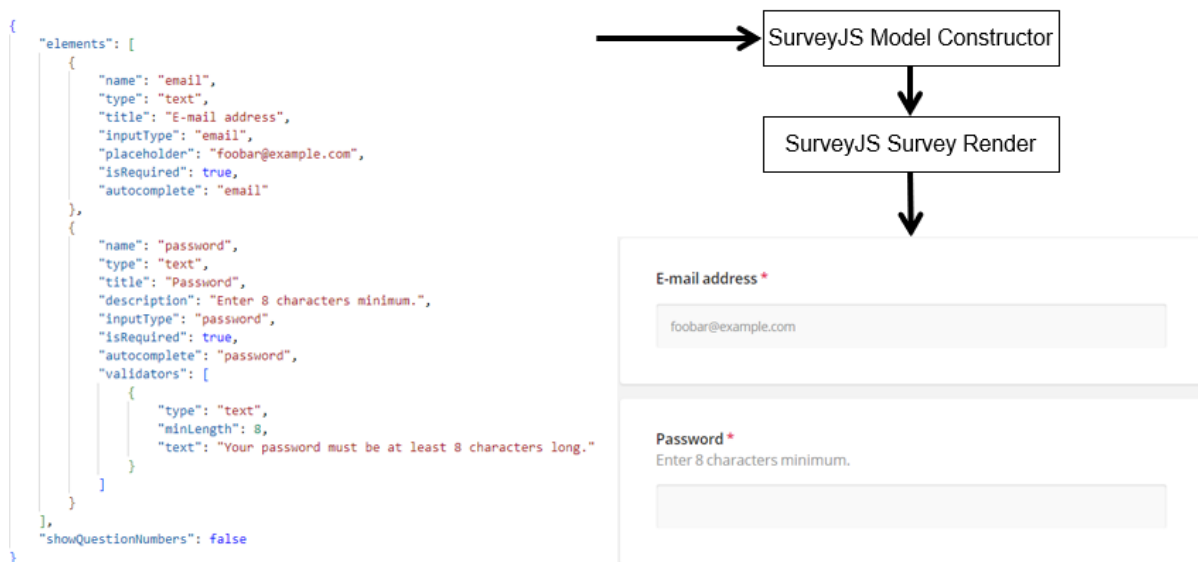
Figure 4: High-level depiction of how a form is created from a JSON model Source: Own Illustration
