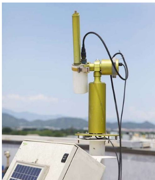
Figure 2.1: A typical CIMEL Electronics CE-318 sun photometer used in the AERONET mission. (Image credit: Dong, 2020)
