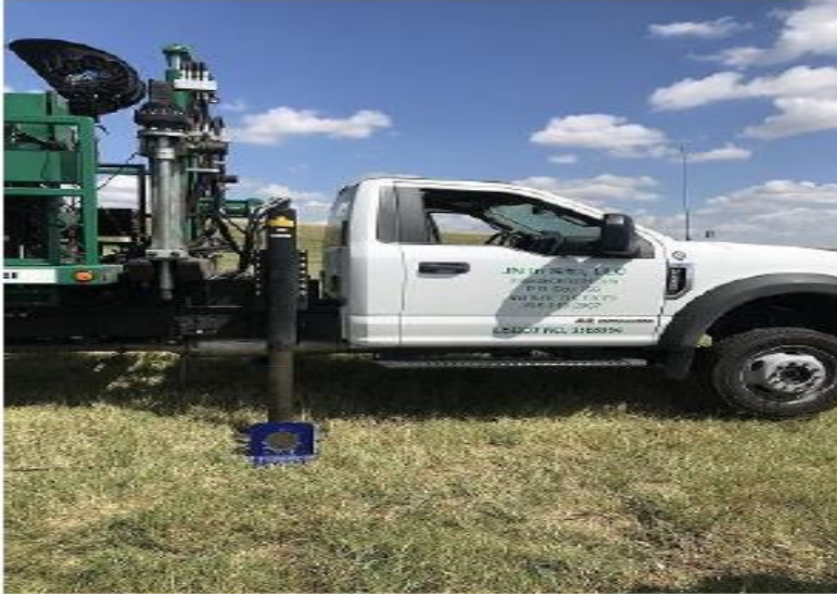
Figure 2.2: SCPT equipment used for data collection
