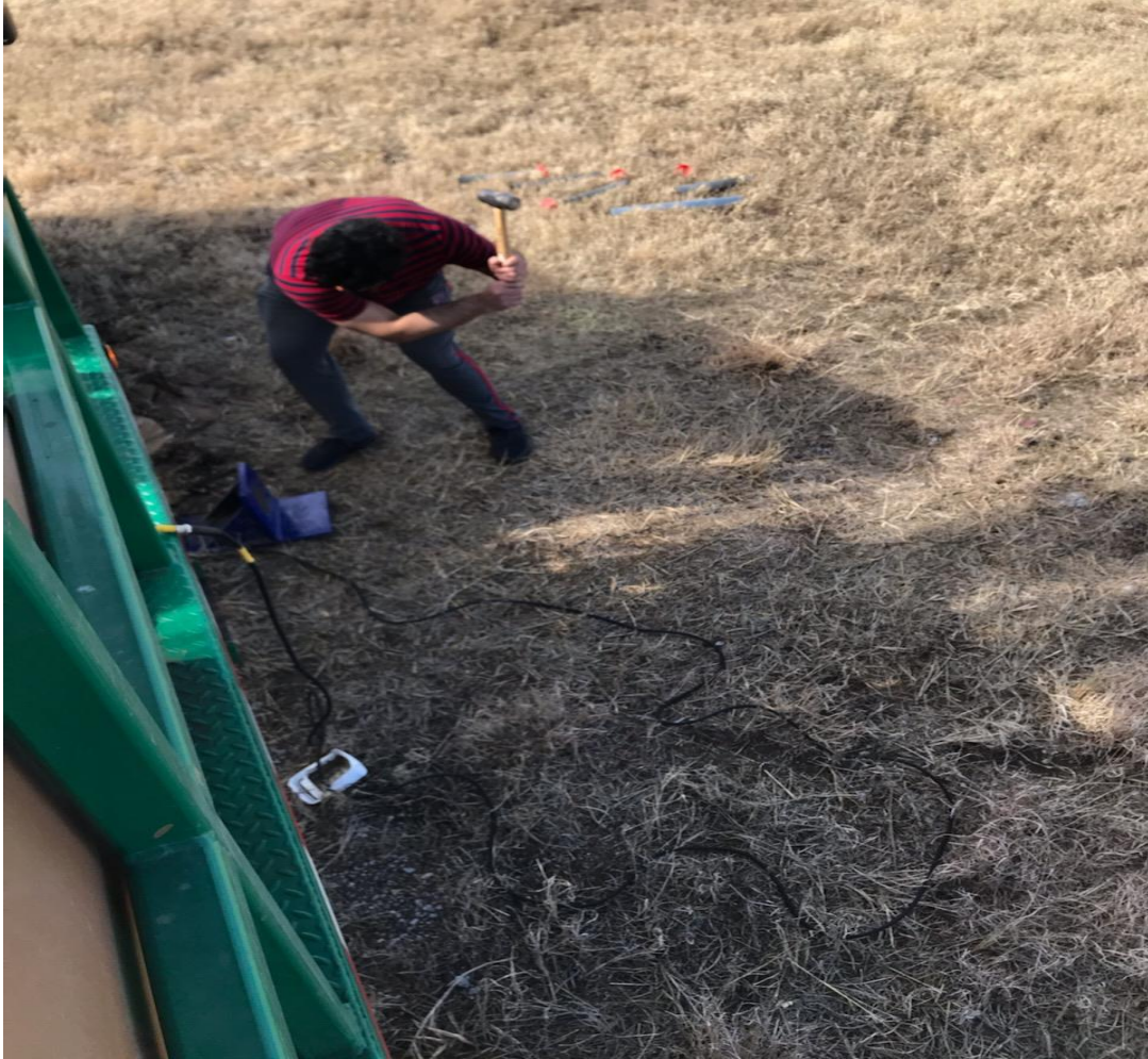
Figure C.3: A student about to stroke the shear beam to trigger seismic waves for the SCPT data collection process
