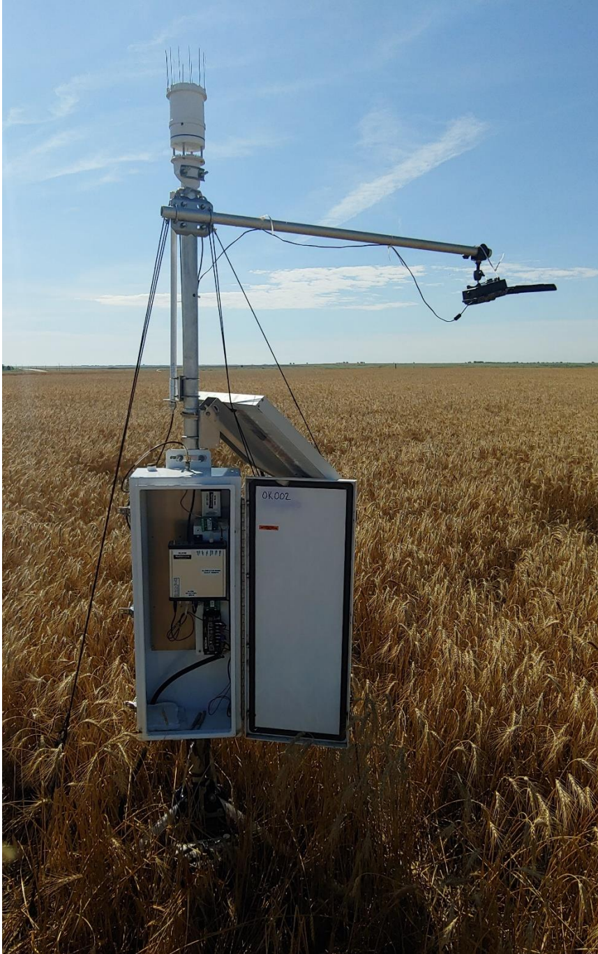
Figure 2. Photograph of CRONOS station 2 located in Tillman County, Oklahoma near the town of Chattanooga. This station is equipped with an all-in-one weather station (top), digital camera (arm), and cosmic ray neutron detector (box) which is located behind the data logger (box).
