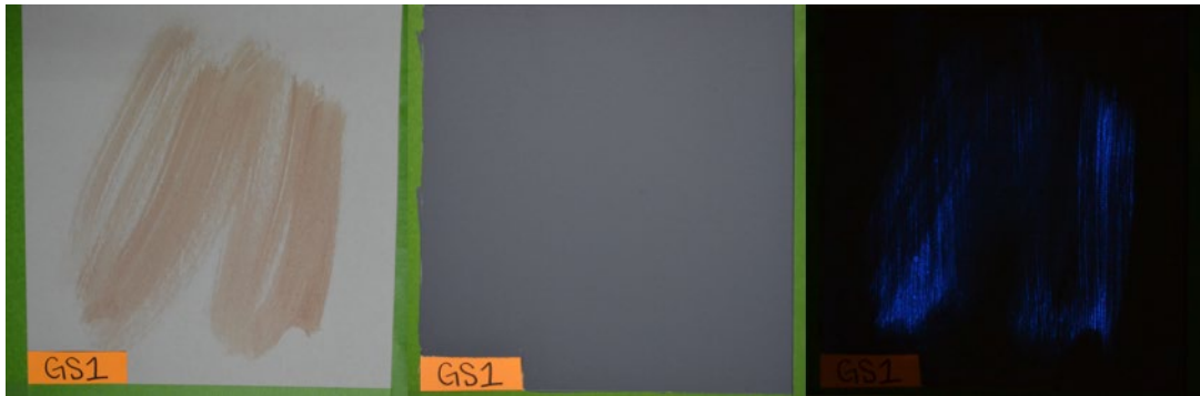
Figure 66. Swipe, Grey Colour, Sherwin Williams Paint and Primer, 1 Layer of Paint
