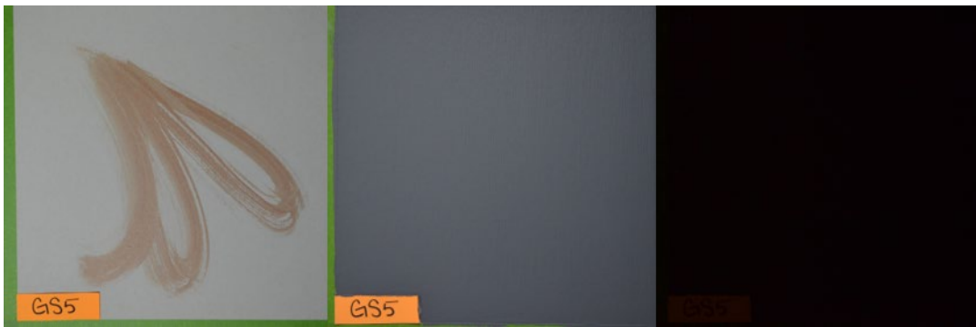
Figure 68. Swipe, Grey Colour, Sherwin Williams Paint and Primer, 5 Layers of Paint
