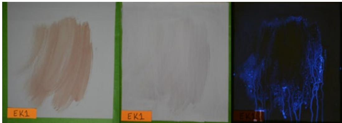
Figure 58. Swipe, Grey Colour, Kilz Primer, 1 Layer of Paint
