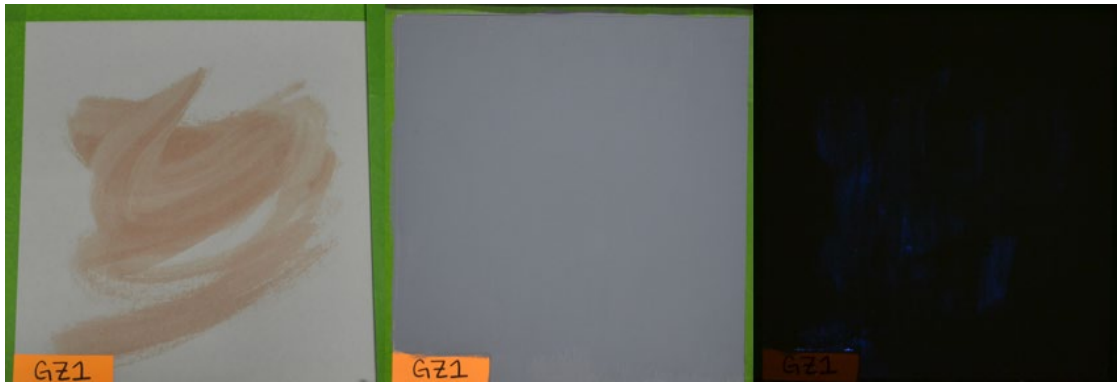
Figure 78. Swipe, Grey Colour, Zinsser Primer, 1 Layer of Paint
