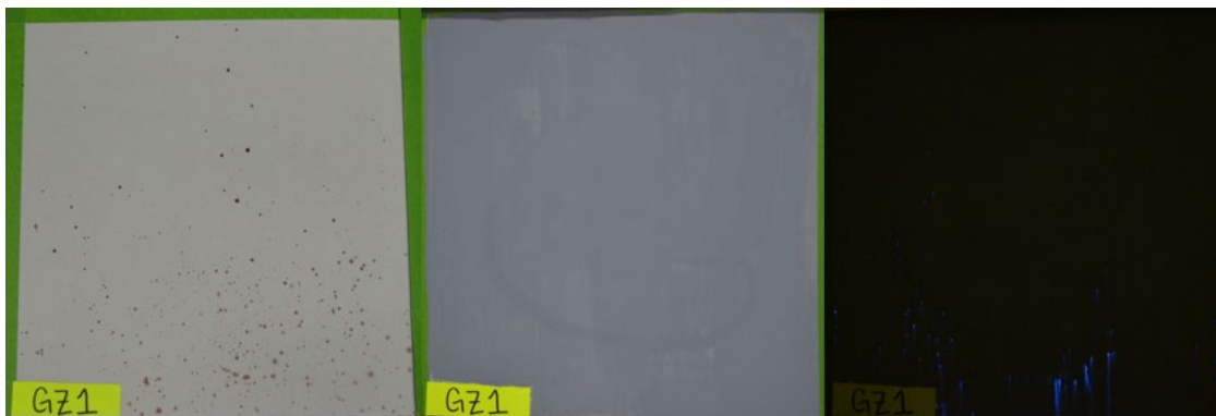
Figure 46. Spatter, Grey Colour, Zinsser Primer, 1 Layer of Paint
