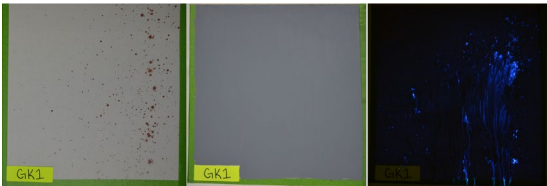
Figure 42. Spatter, Grey Colour, Kilz Primer, 1 Layer of Paint
