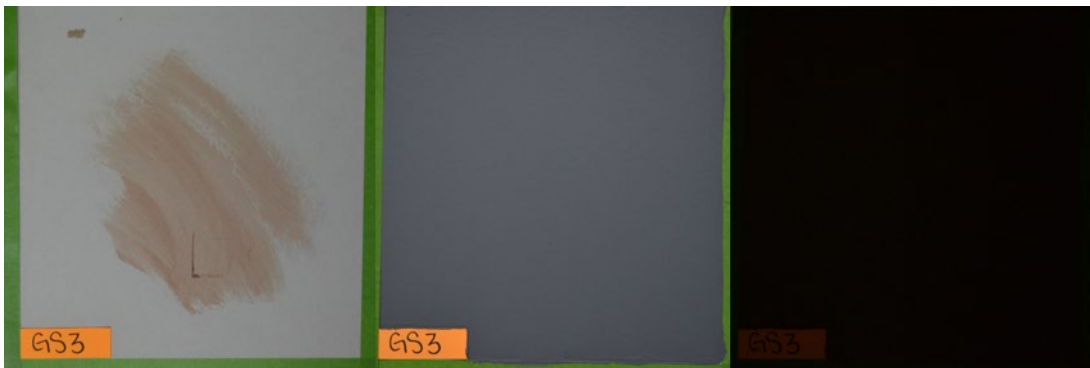
Figure 67. Swipe, Grey Colour, Sherwin Williams Paint and Primer, 3 Layers of Paint
