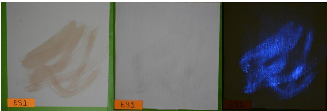
Figure 50. Swipe, Grey Colour, Sherwin Williams Paint and Primer, 1 Layer of Paint
