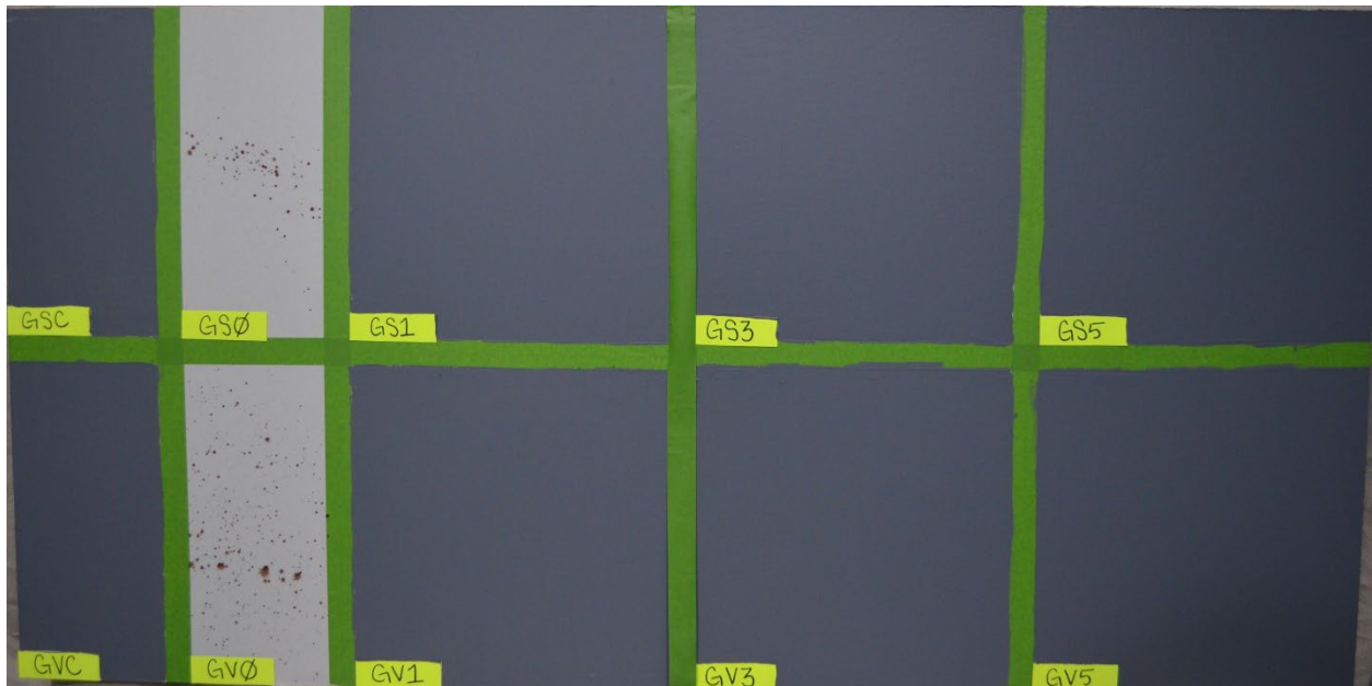
Figure 11. Spatter, Grey Colour, Sherwin Williams & Valspar Paint and Primer
