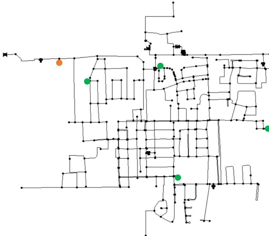
Figure 16. Locations of fire flow simulations.
