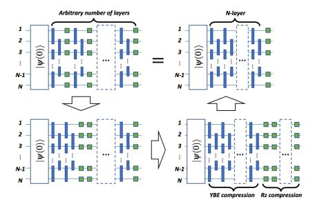
FIG. 9. Circuit compression for XX+Z model. Two-qubit gates for XX interaction are denoted by blue blocks, and single qubit Rz gates are denoted by green blocks. Note that blue and green blocks commute<sup>3</sup>.
