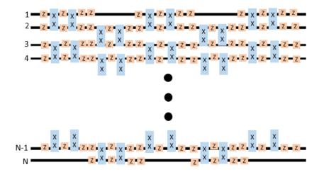
FIG. 13. The XY+Z QTD circuit for N qubits after substituting in  $e^{i\frac{\pi}{4}Z_i}e^{i\frac{\pi}{4}Z_{i+1}}X_iX_{i+1}e^{-i\frac{\pi}{4}Z_i}e^{-i\frac{\pi}{4}Z_{i+1}}$  for every  $Y_iY_{i+1}$  block.
