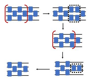
FIG. 8. Compression scheme for 4 qubits. Reflection symmetry exists with two layers of alternative gates. Addition of a third layer can be absorbed into the two layers by recursive usage of reflection symmetry (red bracket) via the YBE and merge identity (black dotted box)<sup>3</sup>.
