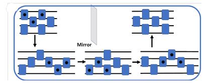
FIG. 7. Reflection symmetry is achieved by using the YBE four times on four qubits (action of YBE on which triplets is shown by black dots)<sup>3</sup>.
