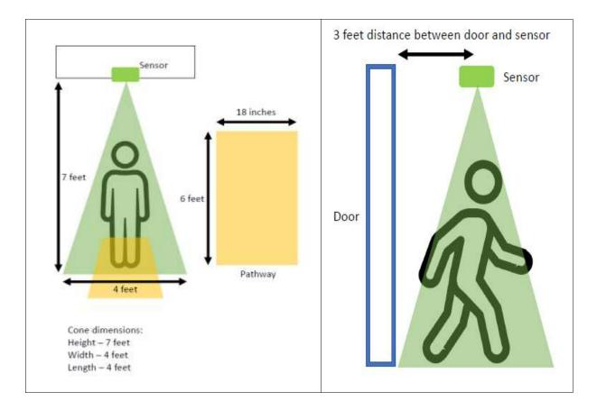
FIGURE 21: SENSOR PLACEMENT
