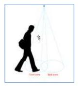
FIGURE 22: SENSOR FIELD VIEW
