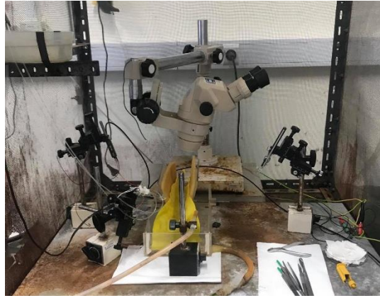
Figure 2.1 EOG experiments were conducted in a Faraday cage to block electromagnetic fields.
