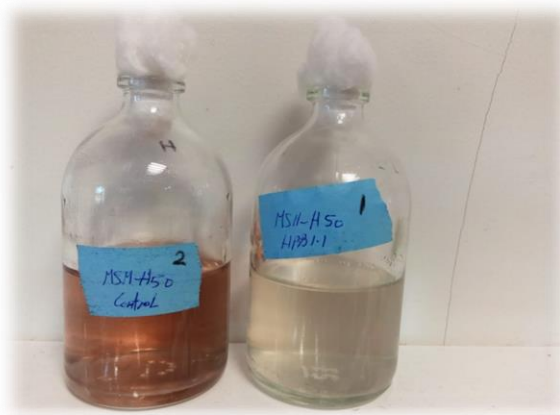
Figure 3.31. MSM-HQ (50 mgL -1 ) culture of Mycolicibacterium sp. (HPB1.1) (on the right) after seven days, showing no color change compared with the brownish coloration of the negative control medium (on the left).
