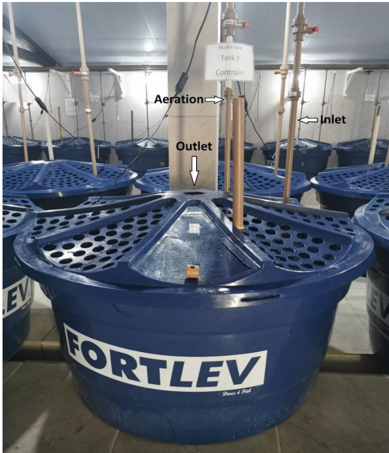
Figure 3.2: Individual tank design used in the experiment. All 20 tanks had the same design with the inlet next to the wall and outlet and aeration in the middle of the tank.
