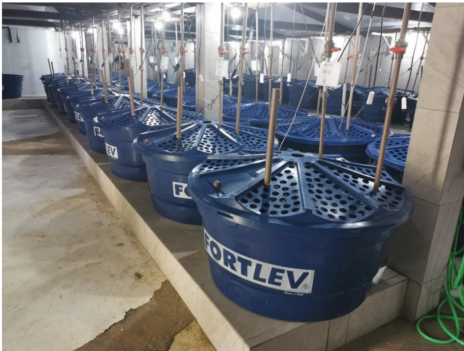
Figure 3.3: Experimental set up with 20 tanks of 400 liter ( n = 4 for each experimental diet).
