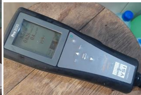
Figure 3.5: YSI Pro 20 probe was used to keep the temperature at 10.9 \pm 0.1 \text{ }^{\circ}\text{C} .
