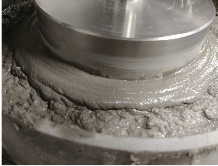
Fig. 2.4. Shear-induced volumetric change of an assembly of particles: compaction from loosely-packed to closely-packed arrangement, pushing out the suspending matrix from the voids [28-30].
