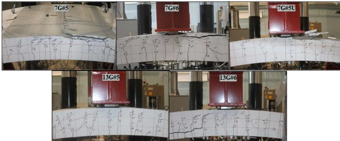
Figure 7.4 Failure mode of the tested specimens.
