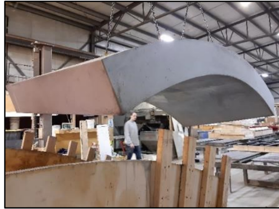
Figure 5.1 (a) Geometry of tunnel segment specimens (dimensions in mm); (b) fabricated cage inside formwork (13G#5H); (c) specimen demolding.
