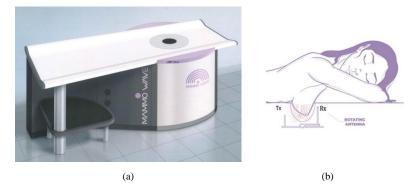
**Figure 2.** MammoWave system (**a**) and sketch of the breast imaging configuration showing a woman's breast inside the cup and the transmitting and receiving rotating antennas (**b**).
