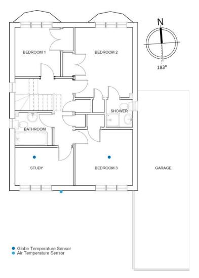
Figure 14. Sensor Layout for Case Study 2
