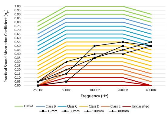
Figure 125. Practical Sound Absorption Coefficient ( $\alpha_{pi}$ ) for Sample E at 15, 30, 100 and 300 mm mounting distances.
