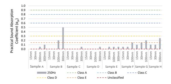
Figure 129. Practical Sound Absorption Coefficient ( $\alpha_{pi}$ ) for all samples tested at all mounting distances at 250 Hz.
