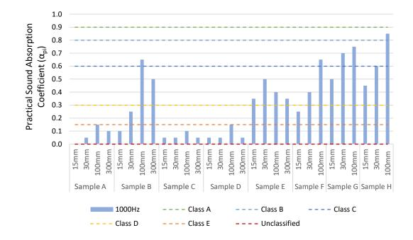
Figure 131. Practical Sound Absorption Coefficient ( $\alpha_{pi}$ ) for all samples tested at all mounting distances at 1000 Hz.
