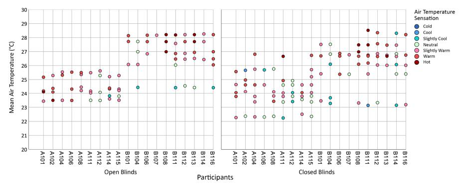
Figure 99. Mean Air Temperature (°C) and Air Temperature Sensation response in the open and closed blind conditions for each participant (Open Blind N = 80, Closed Blind N = 97)
