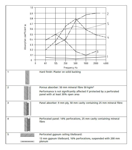
Figure 5. Typical Acoustic Coeffcients for (1) Hard Finish, (2) Porous Absorber, (3) Panel Absorber, (4) Perforated / Cavity Absorber and (5) Perforated Ceiling Tile (BSI, 2014).
