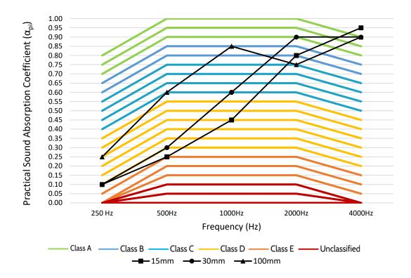
Figure 128. Practical Sound Absorption Coefficient ( $\alpha_{pi}$ ) for Sample H at 15, 30 and 100 mm mounting distances.
