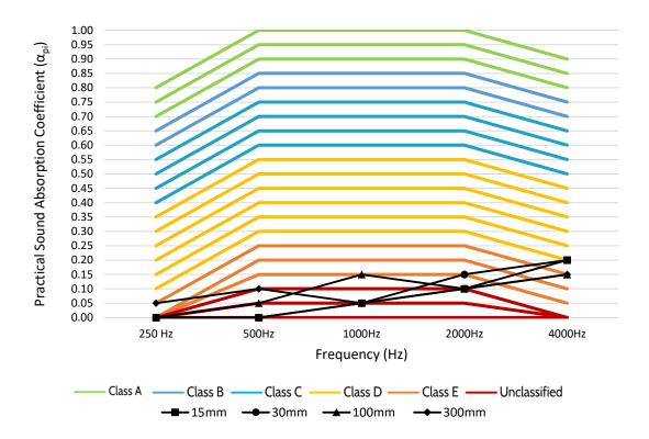
Figure 124. Practical Sound Absorption Coefficient ( $\alpha_{pi}$ ) for Sample D at 15, 30, 100 and 300 mm mounting distances.
