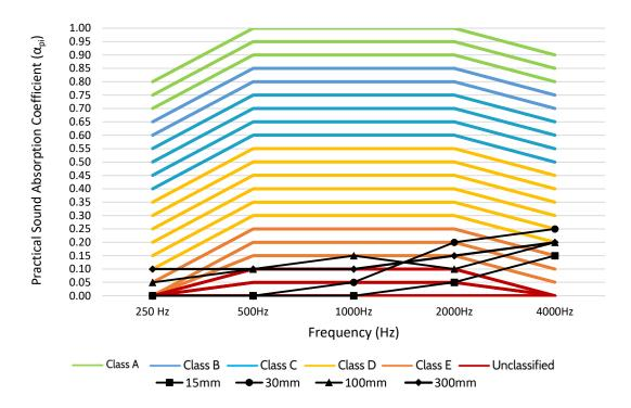
Figure 121.Practical Sound Absorption Coefficient ( $\alpha_{pi}$ ) for Sample A at 15, 30, 100 and 300 mm mounting distances.
