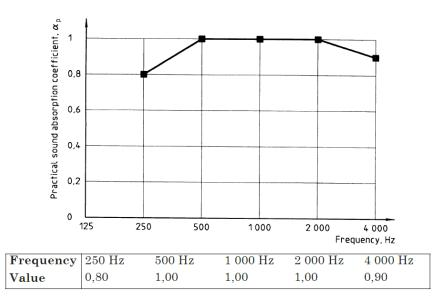
Figure 114. Reference curve for evaluation of Weighted Sound Absorption Coefficient,  $\alpha_w$  as per BS EN ISO 11654 (BSI, 1997).
