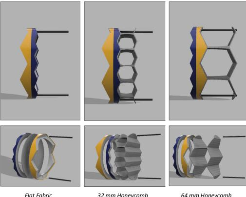
Flat Fabric32 mm Honeycomb64 mm HoneycombFigure 110. Side and exploded view of 100 mm sample holder with test samples.
