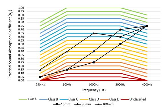
Figure 126. Practical Sound Absorption Coefficient ( $\alpha_{pi}$ ) for Sample F at 15, 30 and 100 mm mounting distances.
