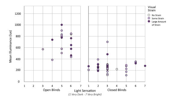
Figure 104. Lighting sensation and visual strain scatter plot of the blind closed (N = 97) and blind open (N = 80) responses.
