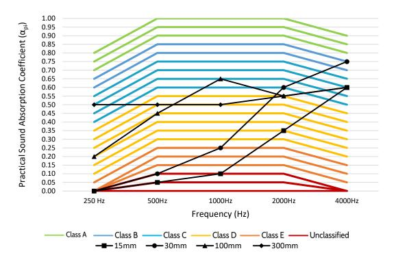
Figure 122. Practical Sound Absorption Coefficient ( $\alpha_{pi}$ ) for Sample B at 15, 30, 100 and 300 mm mounting distances.
