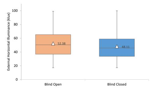
Figure 78. Test Session Mean External Horizontal Illuminance (klux) between the blind open (N = 80) and closed (N = 111) conditions for each participant ( $\Delta$  = Mean).
