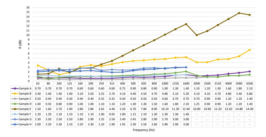
Figure 113. Sound Reduction, R, (dB) for all samples and frequencies measured (Flat Fabrics, Samples A - H, measured across 63 - 6300 Hz and Structured Fabrics, Samples F - H, measured across 63 - 1600 Hz). Frequencies between 250 Hz and 5000 Hz affect speech (Peters et al.,
