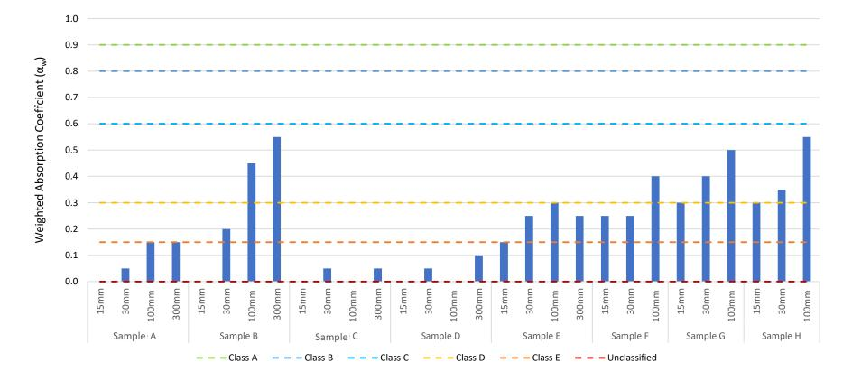
Figure 134. Weighted Sound Absorption ( $\alpha_w$ ) of each sample at differing mounting distances.
