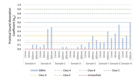
Figure 130. Practical Sound Absorption Coefficient ( $\alpha_{pi}$ ) for all samples tested at all mounting distances at 500 Hz.
