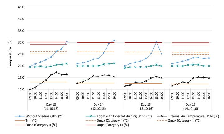
Figure 20. Daily temperature profiles comparing the measured hourly average external air temperature (O), internal operative temperature for rooms with (\*) and without external shading (•), the exponentially weighted running mean air temperature (T<sub>rm</sub>), the internal maximum acceptable operative temperature (Θ<sub>max</sub>) and the absolute maximum operative temperature (Θ<sub>upp</sub>) for the days monitored in October 2016 (Graph 2 of 2)
