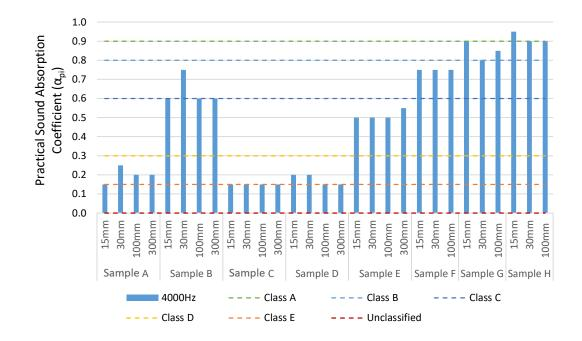
Figure 133. Practical Sound Absorption Coefficient ( $\alpha_{pi}$ ) for all samples tested at all mounting distances at 4000 Hz.
