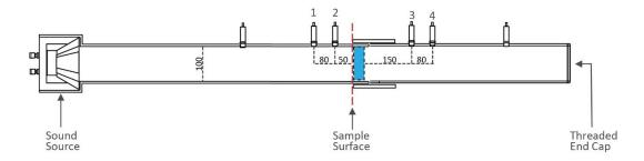
Figure 108.SW-422 100 mm Impedance Tube to measure 63Hz – 1600 Hz sound frequencies. (Items 1,2, 3 and 4 identify the microphone positions and all dimensions are in mm)
