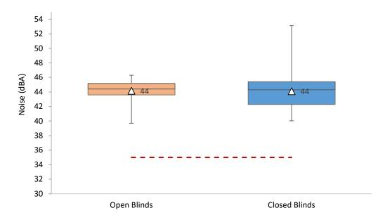
Figure 84. Test Session Mean Noise Level (dBA) between the open (N = 74) and closed (N = 111) blind conditions for each participant (dashed line = comfort threshold,  $\Delta$  = Mean).
