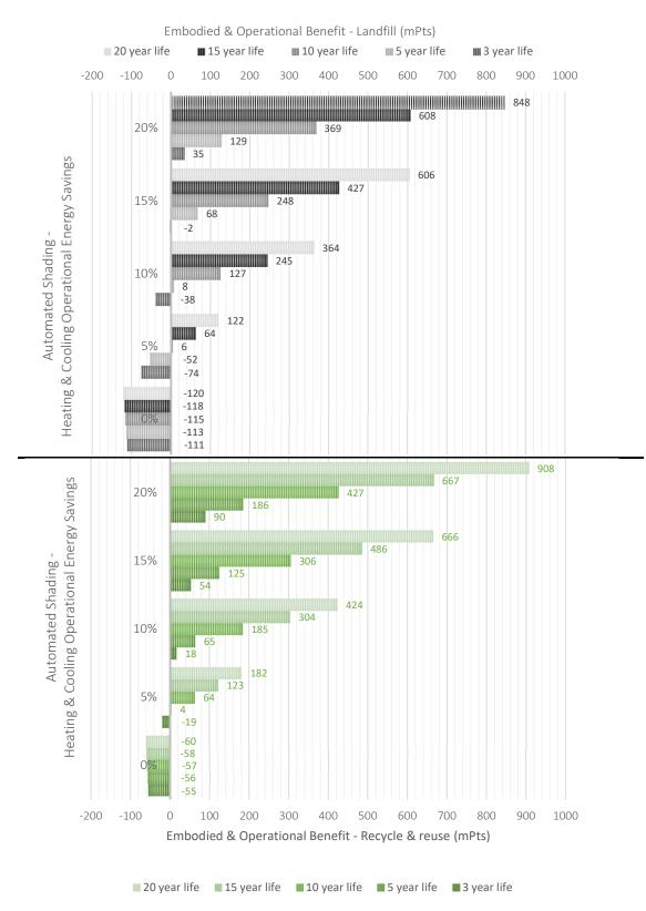
Figure 142. Operational & Embodied Impact of Manual, Motorised and Automated Shading Systems when sent to Landfill or Recycled and reused (Heating & Cooling model)
