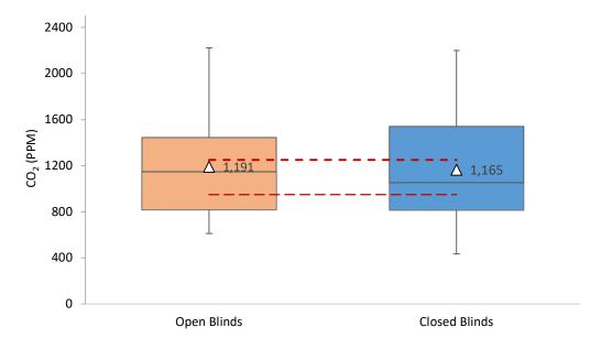
Figure 82. Test Session Mean CO<sub>2</sub> Levels (PPM) between the open (N = 62) and closed (N = 103) blind conditions for each participant (dashed line = comfort threshold,  $\Delta$  = Mean).
