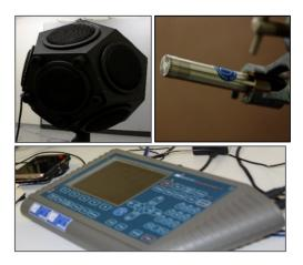
Figure 117.Loudspeaker (Top Left), Microphone (Top Right) and Norsonic Nor121 Environmental Analyser (Bottom)
