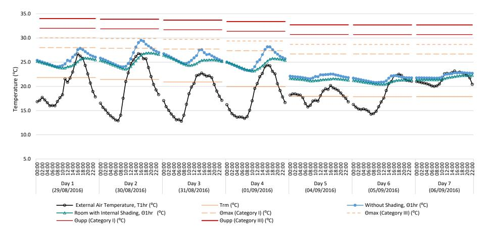
Figure 25. Daily temperature profiles comparing the measured hourly average external air temperature (O), internal operative temperature for rooms with ( $\Delta$ ) and without internal shading (•), the exponentially weighted running mean air temperature ( $T_{rm}$ ), the internal maximum acceptable operative temperature ( $\Theta_{max}$ ) and absolute maximum operative temperature ( $\Theta_{upp}$ ) for the days monitored in August and September 2016 (Graph 1 of 4).
