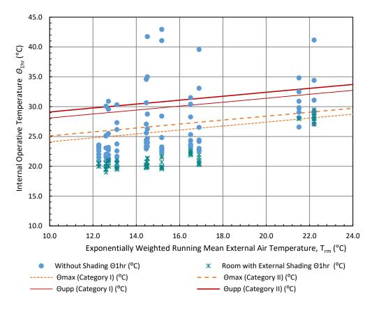
Figure 18. Scatter plot of hourly average indoor operative temperature (O<sub>1hr</sub>) plotted against the exponentially weighted running mean external air temperature (T<sub>rm</sub>) with plots relating to rooms with no shading (●) and rooms with external shading (\*) (80 monitored readings).
