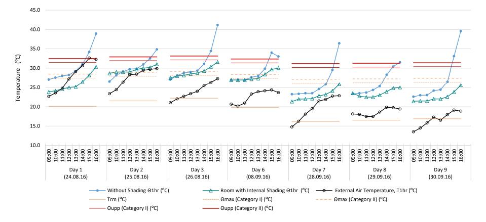
Figure 16. Daily temperature profiles comparing the measured hourly average external air temperature (O), internal operative temperature for rooms with ( $\Delta$ ) and without internal shading (•), the exponentially weighted running mean air temperature ( $T_{rm}$ ), the internal maximum acceptable operative temperature ( $\Theta_{max}$ ) and the absolute maximum operative temperature ( $\Theta_{upp}$ ) for the days monitored in August and September 2016 (Graph 1 of 2).
