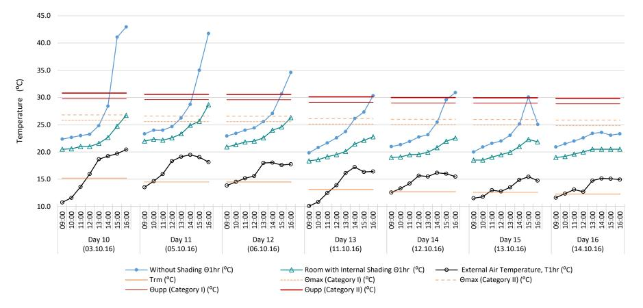
Figure 17. Daily temperature profiles comparing the measured hourly average external air temperature (O), internal operative temperature for rooms with ( $\Delta$ ) and without internal shading (•), the exponentially weighted running mean air temperature ( $T_{rm}$ ), the internal maximum acceptable operative temperature ( $\Theta_{max}$ ) and the absolute maximum operative temperature ( $\Theta_{upp}$ ) for the days monitored in October 2016 (Graph 2 of 2).
