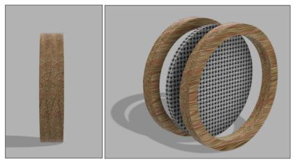
Figure 111.Side and exploded view of 30mm sample holder setup for flat fabrics.
