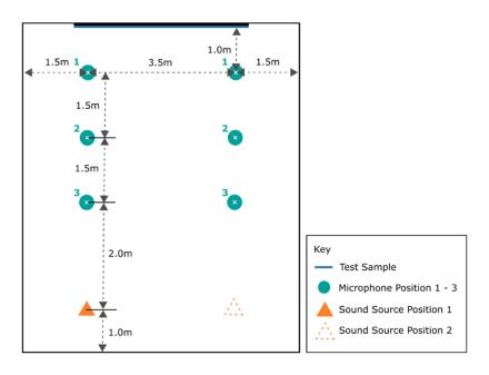
Figure 116. Layout of the equipment within the reverberation room
