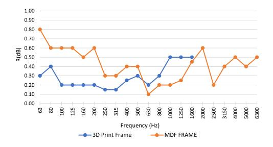
Figure 112. Sound Reduction Index, R (dB) for 3D printed and MDF sample holder.
