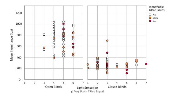
Figure 105. Lighting sensation and identifiable glare issues scatter plot for the blind closed (N = 97) and blind open (N = 80) responses.
