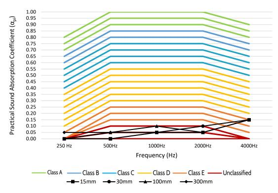
Figure 123. Practical Sound Absorption Coefficient ( $\alpha_{pi}$ ) for Sample C at 15, 30, 100 and 300 mm mounting distances.
