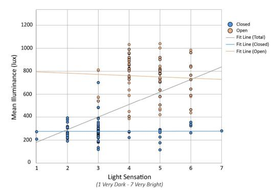
Figure 100. Relationship between mean illuminance (lux) and light sensation responses in the blind closed (•) and blind open (•) conditions (blind closed = 97, blind open N = 80) with lines of best fit.
