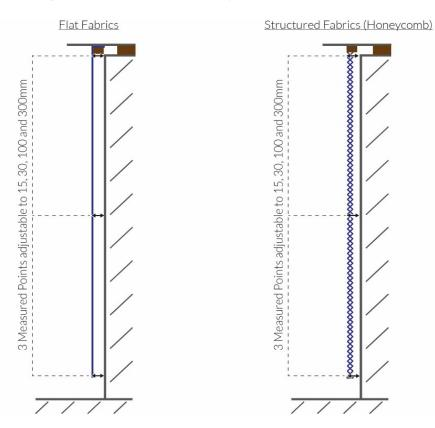
Figure 120. Mounting of shading fabrics within the reverberation room
