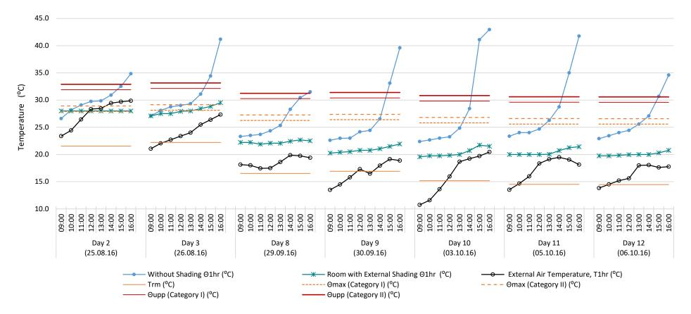
Figure 19. Daily temperature profiles comparing the measured hourly average external air temperature (O), internal operative temperature for rooms with (\*) and without external shading (•), the exponentially weighted running mean air temperature (T<sub>rm</sub>), the internal maximum acceptable operative temperature (Θ<sub>max</sub>) and the absolute maximum operative temperature (Θ<sub>upp</sub>) for the days monitored in August, September and October 2016 (Graph 1 of 2).
