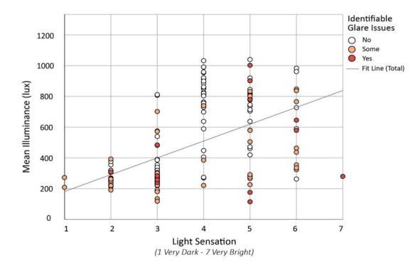
Figure 101. Relationship between mean illuminance (lux), light sensation, and identifiable glare issues with the line of best fit (N = 171).
