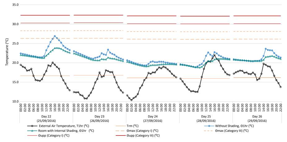
Figure 28. Daily temperature profiles comparing the measured hourly average external air temperature (O), internal operative temperature for rooms with ( $\Delta$ ) and without internal shading (•), the exponentially weighted running mean air temperature ( $T_{rm}$ ), the internal maximum acceptable operative temperature ( $\Theta_{max}$ ) and the absolute maximum operative temperature ( $\Theta_{upp}$ ) for the days monitored in September 2016 (Graph 4 of 4).
