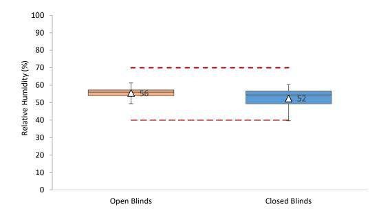
Figure 83. Test Session Mean Relative Humidity between the open (N = 74) and closed (N = 111) blind conditions for each participant (dashed line = comfort threshold,  $\Delta$  = Mean).
