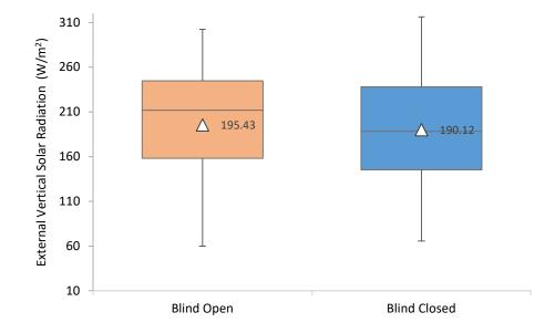
Figure 79. Test Session Mean External Vertical Solar Radiation (w/m<sup>2</sup>) during the test sessions between the blind open (N = 80) and closed (N = 111) conditions for each participant ( $\Delta$  = Mean).
