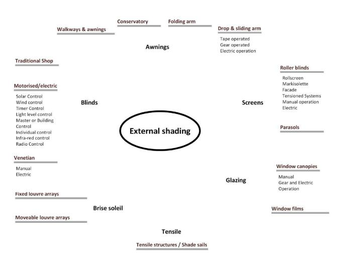
Figure 2. Product Dissemination of External Shading Products (Seguro and Palmer, 2016)
