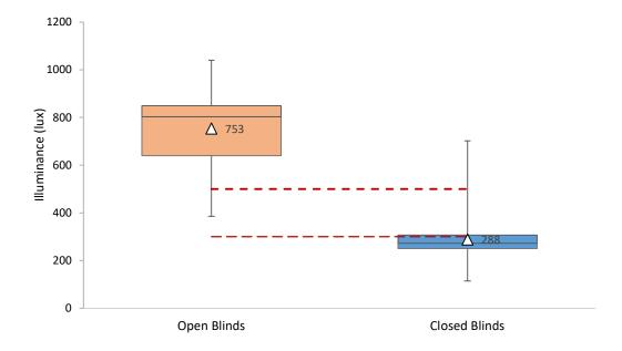
Figure 85. Test Session Mean Illuminance between the open (N = 74) and closed blind (N = 111) conditions for each participant (dashed line = comfort threshold,  $\Delta$  = Mean).
