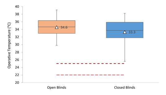
Figure 80. Test Session Mean Operative Temperature between the open (N = 66) and closed (N = 102) blind conditions for each participant (dashed line = comfort threshold,  $\Delta$  = Mean).
