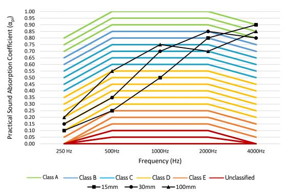
Figure 127. Practical Sound Absorption Coefficient ( $\alpha_{pi}$ ) for Sample G at 15, 30 and 100 mm mounting distances.
