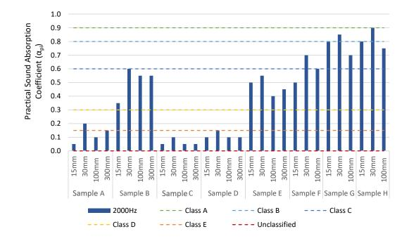
Figure 132. Practical Sound Absorption Coefficient ( $\alpha_{pi}$ ) for all samples tested at all mounting distances at 2000 Hz.
