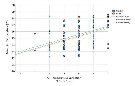
Figure 98. Mean Air Temperature (°C) and Air Temperature Sensation responses in the blind closed (•) and blind open (•) conditions (Blind Closed = 97, Blind Open N = 80) with lines of best fit.
