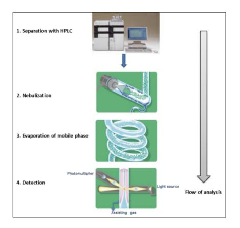
Figure 2.7: Principle of HPLC-ELSD detection of compounds during analysis (Campos et al., 2016).
