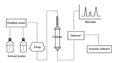
Figure 2.6: The main components of a medium pressure liquid chromatography system (Claeson et al., 1993).
