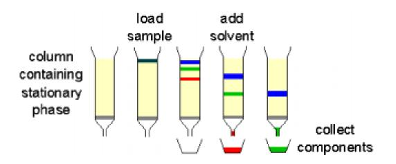
Figure 2.5: Liquid chromatography (LC) separation procedure
