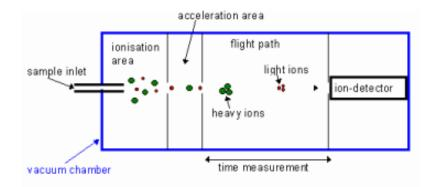
Figure 2.11: Time-of-Flight mass analyser
