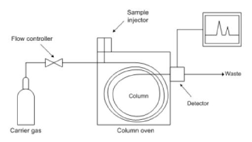
Figure 2.4: Diagram of a gas chromatography mass spectrometer (GC-MS)
