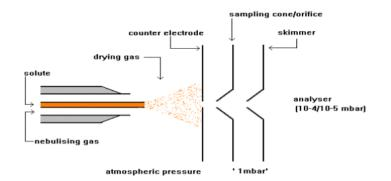
Figure 2.8: Basic diagram of an electrospray ionisation (ESI)
