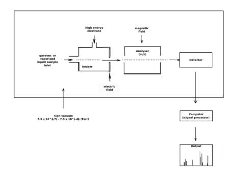
Figure 2.3: Schematic of the main components of a mass spectrometer (Prelorendjos, 2014).
