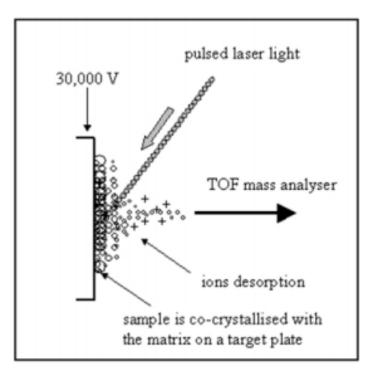
Figure 2.9: Basic diagram of a matrix assisted laser desorption ionisation (MALDI)
