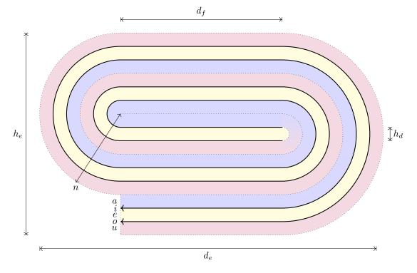
Figure 6.4: A concentric element with 3 dielectric layers
