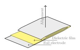
Figure 2.2: A simple winding
