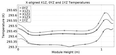
(c) Temperature along X1Z, 0YZ, and 1YZ cut lines for heat on a tab connector  $$X$-aligned XY0 and XY1 Temperatures}$
