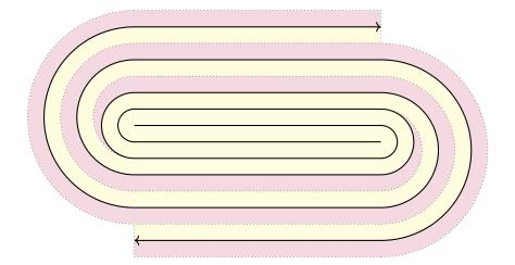
Figure 6.13: A graded counterroll element with 3 dielectric layers
