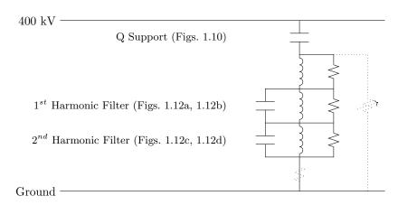
Figure 1.5: A filter bay line diagram (p108, [9])
