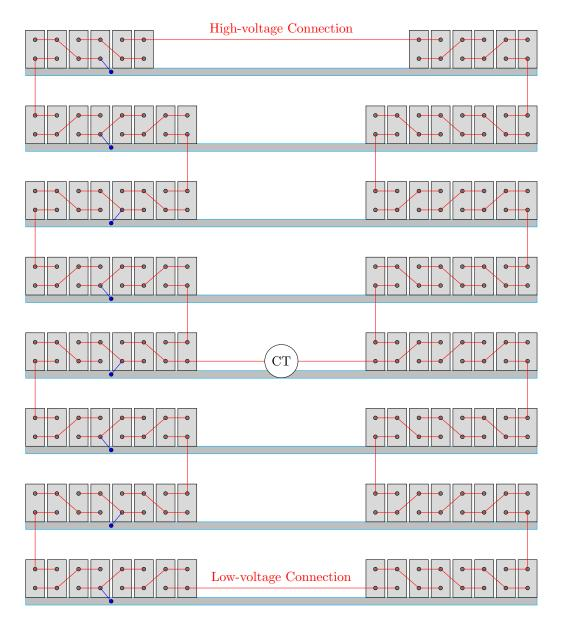
Figure 1.11: Jumper (red), rack tie (blue), and CT connections for both sides of a large bank
