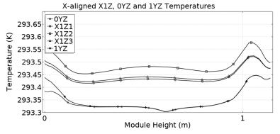
(c) Temperature along X1Z, 0YZ, and 1YZ cut lines for a central heat source  $% \left( {{\mathbf{x}_{i}}} \right)$
