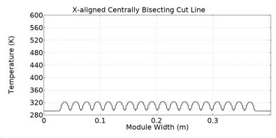
(a) Temperature along a centrally bisecting cut line for heat on a tab connector X-aligned X0Z, 0YZ and 1YZ Temperatures
