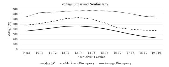
Figure 4.4: Voltage stresses between foils and deviation from a straight line
