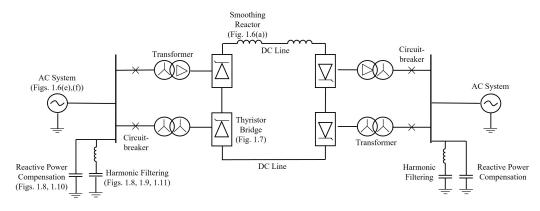
Figure 1.3: Line diagram of an LCC HVDC link [8]
