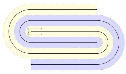
Figure 6.7: A counterroll element with 2 dielectric layers
