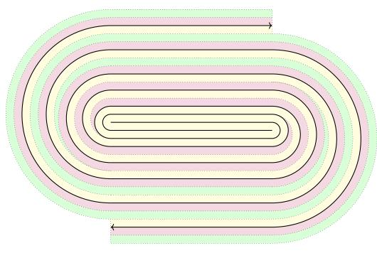
Figure 6.15: A graded counterroll element with 5 dielectric layers
