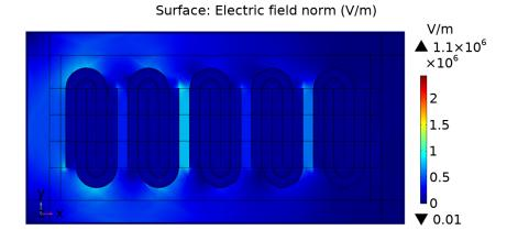
(a) A cut plane in XY at Z2 showing electric field effects at the centre of 5 elements Surface: Electric field norm (V/m)
