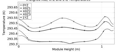
(b) Temperature along X0Z, 0YZ, and 1YZ cut lines for a penultimate foil heat source
