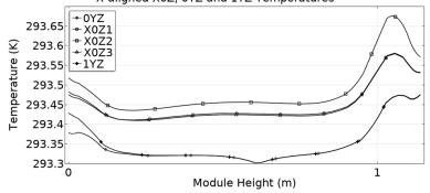
(b) Temperature along X0Z, 0YZ, and 1YZ cut lines for heat on a tab connector
