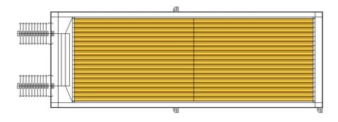
Figure 5.1: A capacitor model with foils aligned to the X-axis
