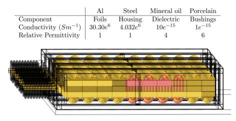
Figure 4.20: Foils in a capacitor unit with 5 series groups of 2 elements each
