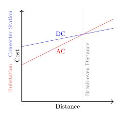
Figure 1.4: Cost-distance relationship for AC and DC connections (p320, [10])
