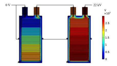
Figure 4.22: Voltage shared by units connected to a rack (left) and to 22 kV (right)
