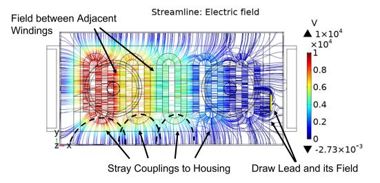
Figure 4.13: A streamline of electric field shows the nature of stray effects
