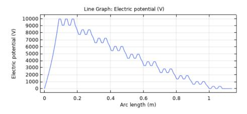
Figure 4.2: Voltage over a cross-section and cut line of a simple unit
