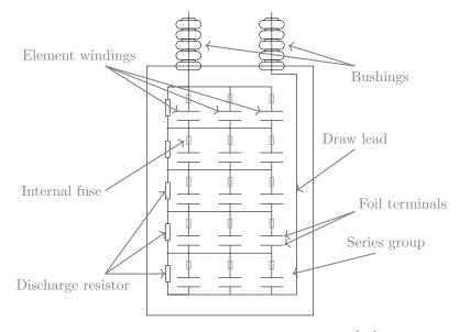
Figure 2.1: A capacitor unit line diagram [28]
