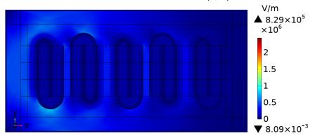
(b) A cut plane in XY at Z2.5 showing electric field at element margins Surface: Electric field norm (V/m)  $\,$
