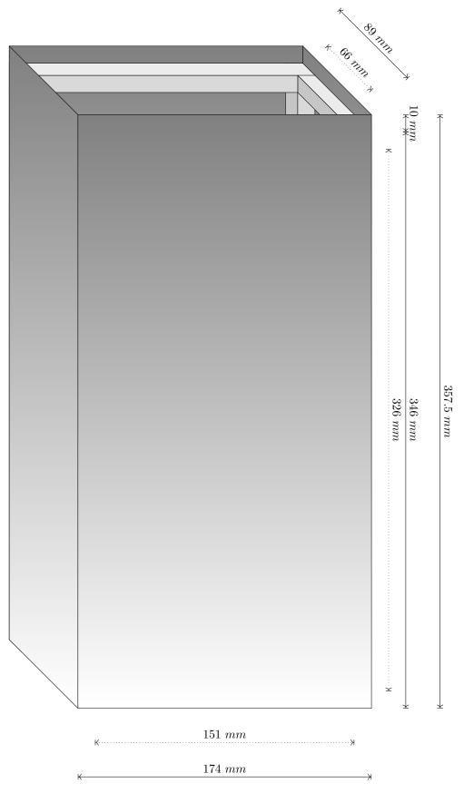
Figure 6.2: Scale model frame with enclosed sides
