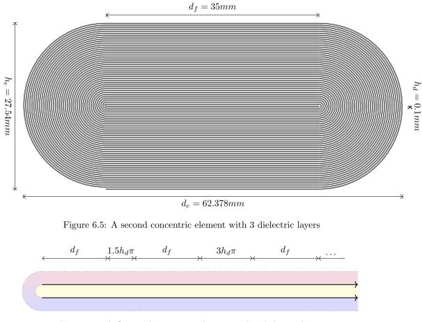
Figure 6.6: A flattened concentric element with 3 dielectric layers
