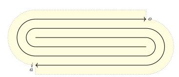
Figure 6.9: A counterroll element with 1 dielectric layer
