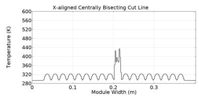
(a) Temperature along a centrally bisecting cut line for a penultimate foil heat source X-aligned X0Z, 0YZ and 1YZ Temperatures
