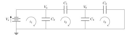
Figure 4.5: A simplified equivalent circuit with stray capacitances  $C_3$  and  $C_4$
