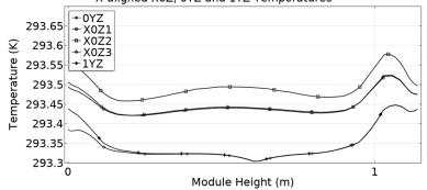
(b) Temperature along X0Z, 0YZ, and 1YZ cut lines for a central heat source
