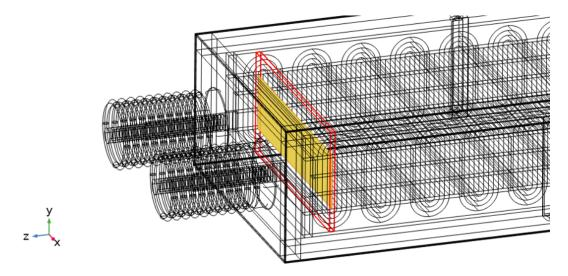
Figure 3.7: A single boundary selected from the specified settings
