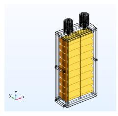
Figure 5.12: A 9-winding, 40-turn model
