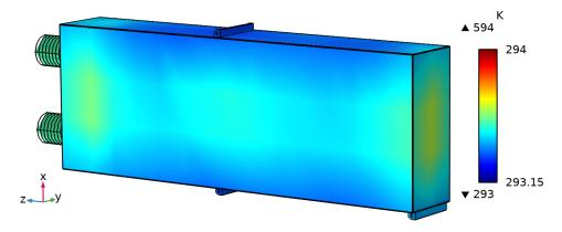
Figure 5.6: Point heat source on a penultimate foil
