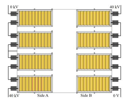
Figure 4.21: Foils in a capacitor rack of 8 units
