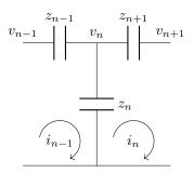
Figure 4.8: Stray capacitance in the general case
