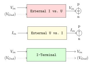
Figure 3.5: Nodes to couple geometrical (left) to Electric Circuit (right) physics
