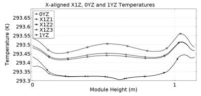
(c) Temperature along X1Z, 0YZ, and 1YZ cut lines for a penultimate foil heat source  $% \left( {{\mathbf{x}_{1}}} \right)$
