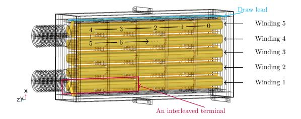
Figure 4.11: A unit with interleaved foil windings in yellow and numbered elements
