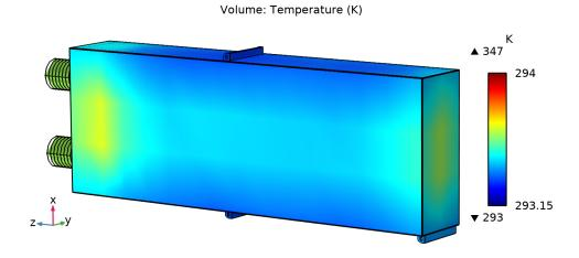
Figure 5.7: Point heat source on a tab connector
