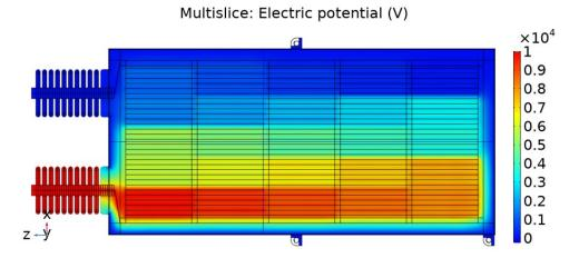
Figure 4.14: A cut plane shows voltage to increase within each interleaved winding
