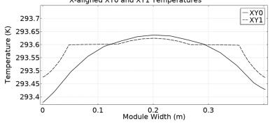
(d) Temperature along XY0 and XY1 cut lines for heat on a tab connector
