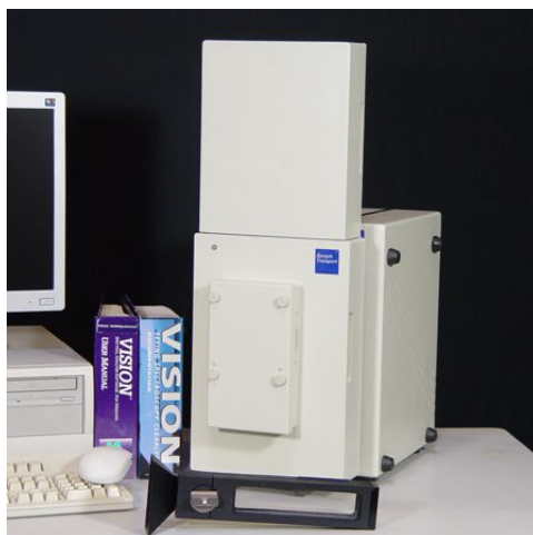
Figure 3.3: At-line instrument used: 6500 NIR (FOSS NIRSystems, Inc., USA) with sample transport module.
