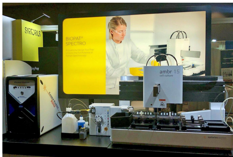
Figure 6.1: The Ambr ® system with BioPat Spectro using Raman from Kaiser Optical Systems
