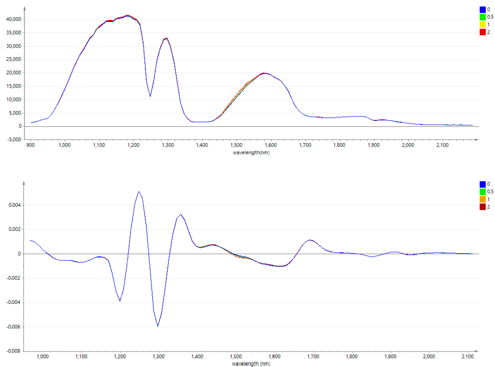
Figure 4.10: Raw spectra of pure samples of lactate (0, 0.5, 1.0 and 2.0 M) (top plot) and pretreated with SNV, second derivative and Savitzky-Golay filter (bottom plot).
