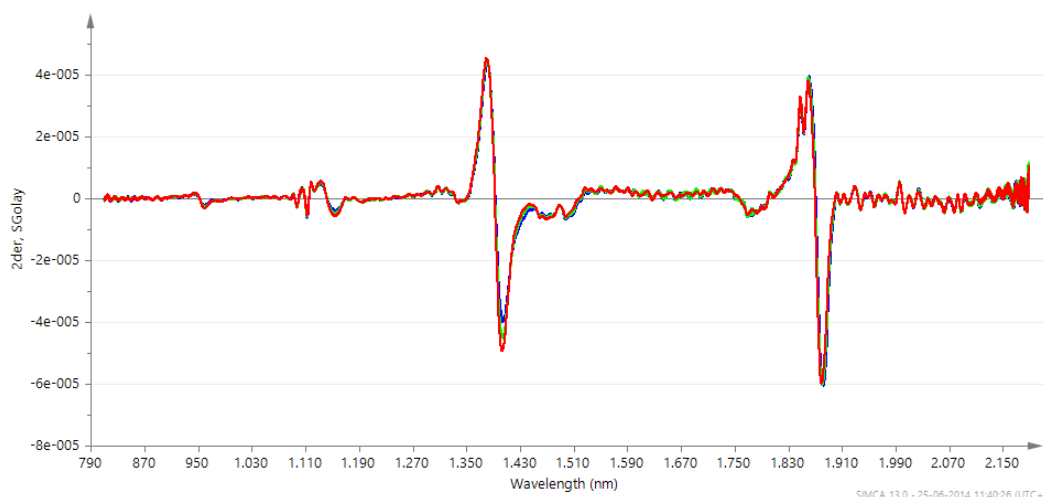
Figure 3.32: Second derivative of the online spectra of 2.5 g/L glucose solution at three different temperatures: 10°C (in blue), 20°C (in green) and 30°C (in red).
