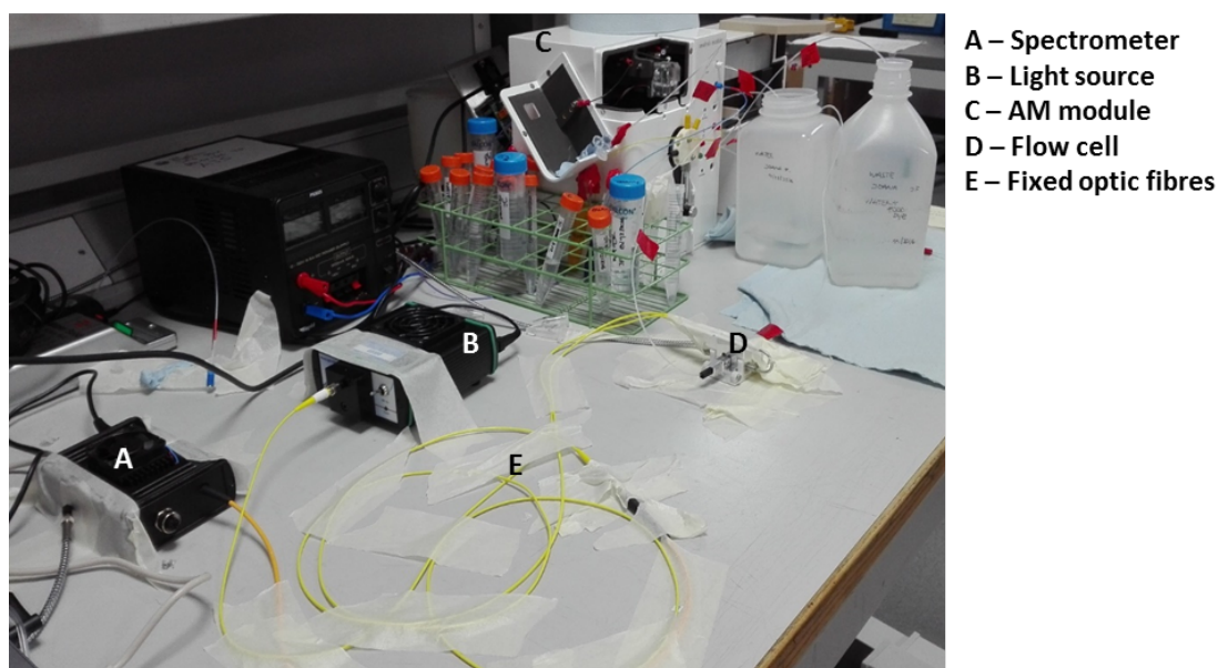
Figure 4.1: Hardware set-up for sample preparation and near infrared spectra collection. Legend in the picture describes the elements seen: A - NIR detector; B - light source, C - Analysis Module used for sample preparation (AM); D - flow-cell; E - fibre optics.
