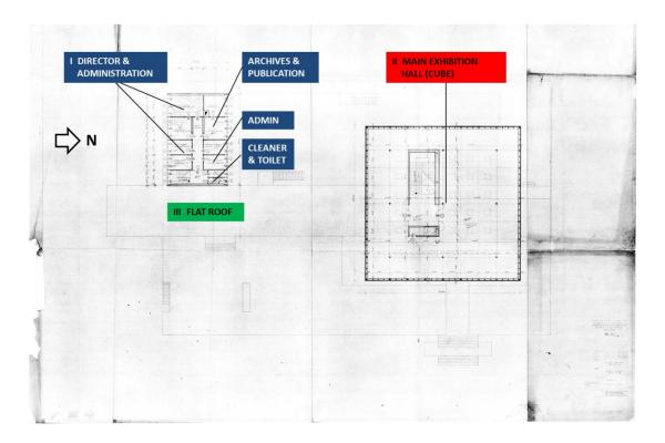
Fig.5.14 Museum of Revolution First floor plan; Annotated by Selma Harrington on the scanned copy of the archival working drawing (AF Sarajevo, courtesy of Dr Aida Idrizbegović Zgonić).
