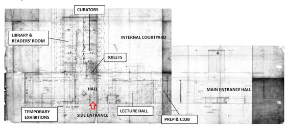
Fig.5.13 Museum of Revolution: Ground floor plan; Annotated by Selma Harrington on the scanned copy of the archival working drawing (AF Sarajevo, courtesy of Dr Aida Idrizbegović Zgonić).
