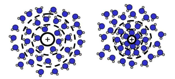
**Figure 1.17. Schematic of the hydration shell around a large and small cation**. Small ions have a larger charge density and hence water molecules will pack more tightly, whereas larger ions will have a lower charge density and water molecules will be more weakly associated with the ion. Adapted from Tansel *et al.*, 2006.
