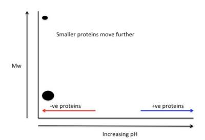
**Figure 3.2. Schematic of a 2D-gel.** In the 1st dimension (X-axis) proteins are separated based on their isoelectric point (IEP), which is the pH at which the protein will stop moving in an electric field, i.e. it becomes overall neutral. The proteins are then separated based on their molecular weight (Y-axis), with smaller proteins migrating faster and further than larger proteins.
