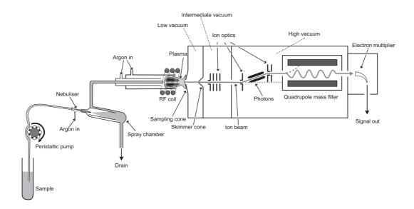
**Figure 5.1. Schematic of an ICP-MS instrument.** The sample is introduced into the instrument via the nebuliser (as an aerosol), where it is desolvated and converted to a gas, before it is ionised by the plasma (argon in this case). The ions are then passed onto the mass spectrometer, where they are separated by their mass to charge ratio (m/z), and the concentration of each ion calculated. Adapted from Linge, 2009.
