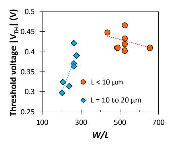
**Figure 4.6:** Threshold voltage as a function of W/L for narrow-gate OTFTs with interdigitated source/drain contacts and  $L < 10 \ \mu m$  (circles) or  $L = 10 \ to \ 20 \ \mu m$  (diamonds).
