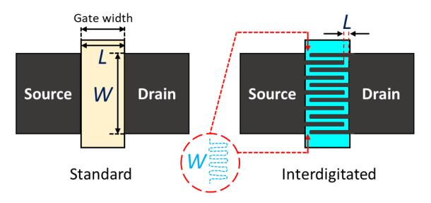
Figure 4.1: Standard rectangular and interdigitated source/drain contacts.
