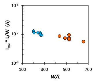
**Figure 4 8:** Normalised on-state drain current as a function of W/L for narrow-gate OTFTs with interdigitated source/drain contacts and  $L < 10 \, \mu m$  (circles) and  $L = 10 \, \text{to } 20 \, \mu m$  (diamonds).
