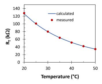
**Figure 6.3:** Temperature response of a thermistor having a nominal resistance of 100  $k\Omega$  at 25°C.
