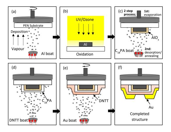
**Figure 3.2:** Flow diagram of MIM structure and OTFT fabrication stages. Note, DNTT (stage d) is omitted during MIM structure fabrication.
