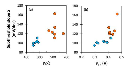
**Figure 4.11:** Subthreshold slope as a function of W/L (a) and  $V_{\rm TH}$  (b) for narrow-gate OTFTs with interdigitated source/drain contacts and  $L < 10~\mu m$  (circles) or L = 10 to  $20~\mu m$  (diamonds).
