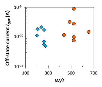
**Figure 4.9:** Off-state drain current as a function of W/L for narrow-gate OTFTs with interdigitated source/drain contacts and  $L < 10 \, \mu m$  (circles) or L = 10 to  $20 \, \mu m$  (diamonds).
