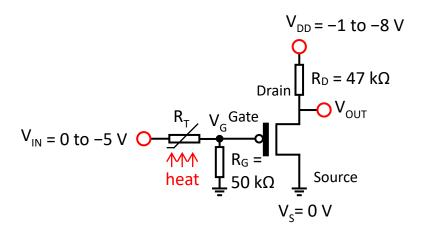
**Figure 6.1:** OTFT based temperature sensor.  $V_{\rm IN} = 0$  to -5 V,  $V_{\rm DD} = -1$  to -8 V,  $V_{\rm S} = 0$  V.  $R_{\rm T}$  has nominal resistance of 100 k $\Omega$  at 25° C and  $R_{\rm D} = 47$  k $\Omega$ .
