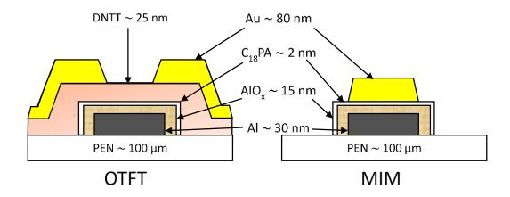
Figure 3.1: OTFT and MIM structure cross-sectional view.
