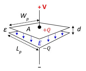
Figure 2.1: Schematic diagram of MIM structure.
