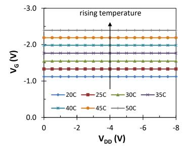
**Figure 6.6:**  $V_{\rm G}$  as a function of  $V_{\rm DD}$  for temperatures between 20 and 50°C,  $R_{\rm G} = 50$  k $\Omega$ ,  $R_{\rm D} = 47$  k $\Omega$  and  $V_{\rm IN} = -4$ V.  $V_{\rm G}$  is referenced to ground.
