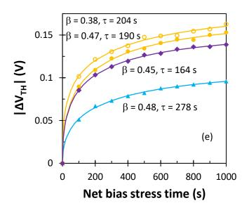
**Figure 5.9:** Threshold voltage shift of 5-6 months aged OTFTs as a function of net bias stress time. The legend of Fig. 5.8 applies.
