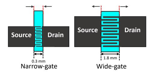
**Figure 4.2:** Schematic of narrow gate and wide-gate OTFTs.
