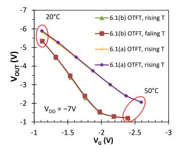
**Figure 6.9:** Repeated measurements of  $V_{\rm OUT}$  as a function of  $V_{\rm G}$  for  $V_{\rm IN} = -4$  V,  $V_{\rm DD} = -7$  V,  $R_{\rm D} = 47$  kΩ,  $R_{\rm G} = 50$  kΩ and OTFTs of Figure 6.2(a) and (b). Rising and falling T represent ramping temperature from 20 to 50°C and from 50 to 20°C respectively.
