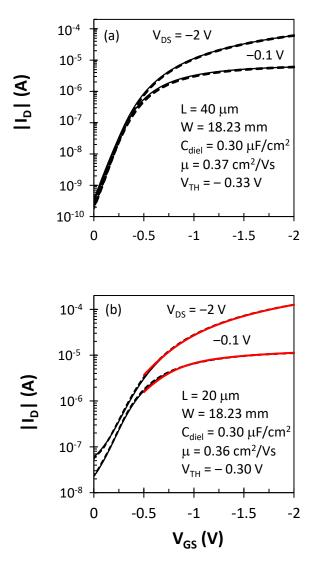
**Figure 6.2:** Transfer characteristics of OTFTs used in the temperature sensor and verification model. Solid black lines and dotted lines represent hysteresis for  $V_{\rm GS}$  ramped in forward direction (0 to -2 V) and reverse (-2 to 0 V) respectively. Solid red lines represents the transistor model.
