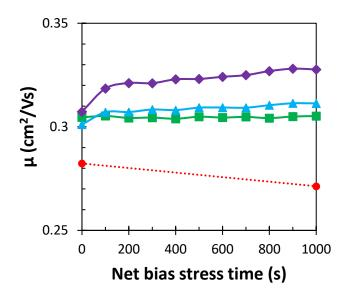
**Figure 5.4:** Field-effect mobility  $\mu$  as a function of net bias stress time. The legend of Fig. 5.2 applies.
