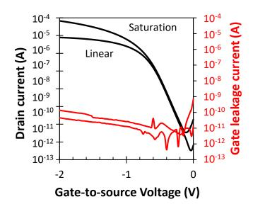
Figure 3.6: Transfer characteristics in linear ( $V_{DS} = -0.1 \text{ V}$ ) and saturation regime ( $V_{DS} = -2 \text{ V}$ ) for  $V_{GS}$  sweep from 0 to -2 V.
