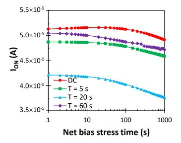
**Figure 5.2:** On-state drain current  $I_{ON}$  as a function of net bias stress time for DC (circles), and AC pulse periods with 1 s on-time and periods; T = 5 s (square), 20 s (triangles) and 60 s (diamonds).
