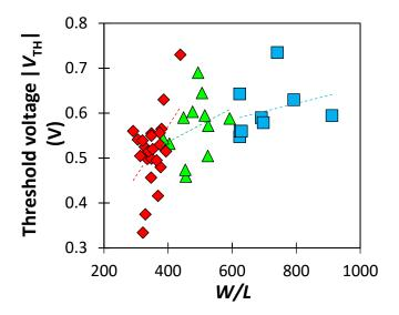
**Figure 4.15:** Threshold voltage as a function of W/L for wide-gate OTFTs with interdigitated source/drain contacts and L=20 to 30  $\mu$ m (square), L=30 to 40  $\mu$ m (triangles), or L=40 to 50  $\mu$ m (diamonds).
