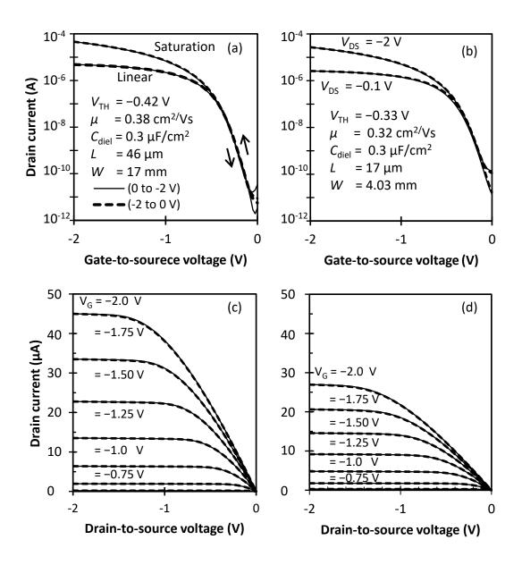
**Figure 4.4:** Transfer (a, b) and output (c, d) characteristics for wide-gate (a, c) and narrow-gate (b, d) OTFTs on PEN. Each curve shows hysteresis measurement from 0 to -2 V (solid line) and back (dash lines).
