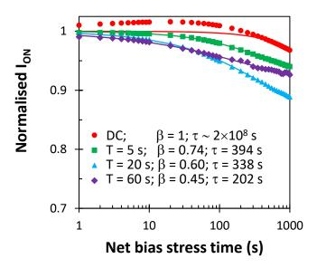
**Figure 5.5:** Normalised on-state drain current of freshly fabricated OTFTs as a function of net bias stress time. Points (symbols) represent measured data and lines are the stretched exponential fits with fitting parameters of  $\beta$  and  $\tau$ .
