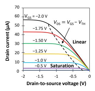
**Figure 3.9:** Output characteristics, plot of drain current as a function of drain-to-source voltage from 0 to -2 V and gate-to-source voltage at -0.25 V increments. Dashed line divides the linear and saturation regimes.
