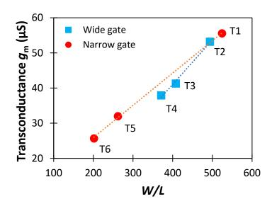
**Figure 4.21:** AC transconductance  $g_m$  as a function of W/L for narrow-gate (circles) and wide-gate (squares) OTFTs.
