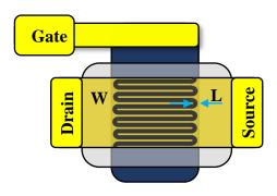
**Figure 3.12:** Top view of an organic thin-film transistor with interdigitated source/drain contacts.
