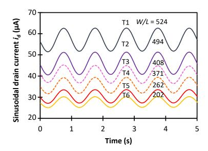
**Figure 4.20:** Sinusoidal drain current as a function of time (for  $v_{gs}$  of  $-0.2V_{pp}$ , and  $V_{DS}$  and  $V_{S}$  of -2 V and 0 V respectively. The solid and dashed lines correspond to narrow- and wide-gate transistors, respectively.
