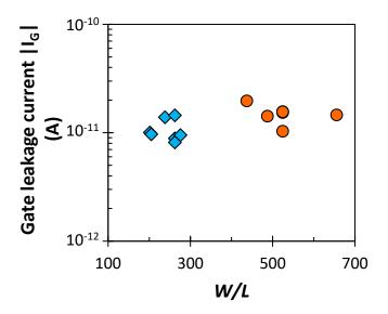
**Figure 4.12:** Gate leakage current as a function of W/L for narrow-gate OTFTs with interdigitated source/drain contacts and  $L < 10 \mu m$  (circles) or L = 10 to  $20 \mu m$  (diamonds).
