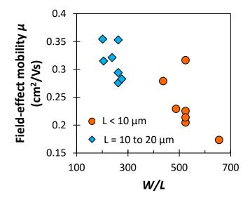
**Figure 4.5:** Field-effect mobility as a function of W/L for narrow-gate OTFTs with interdigitated source/drain contacts and  $L < 10 \ \mu m$  (circles) or  $L = 10 \ to \ 20 \ \mu m$  (diamonds).
