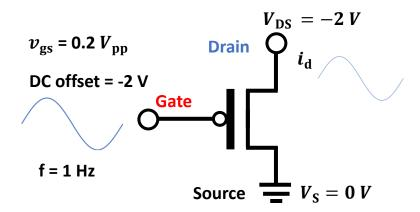
Figure 3.11: AC transconductance measurement setup.
