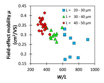
**Figure 4.14:** Field-effect mobility as a function of W/L for wide-gate OTFTs with interdigitated source/drain contacts and L=20 to 30  $\mu$ m (square), L=30 to 40  $\mu$ m (triangles), or L=40 to 50  $\mu$ m (diamonds).
