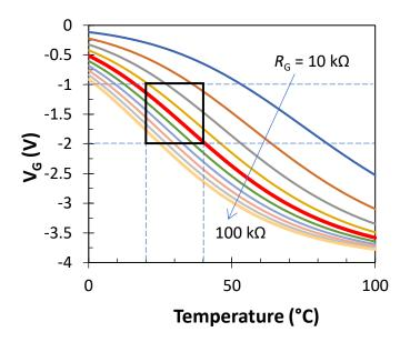
Figure 6.4: Effects of resistor  $R_G$  (10 k to 100 kΩ) on  $V_G$  as a function of temperature. The desirable temperature and voltage range for  $V_G$  are indicated by the black rectangle. The red thick curve corresponds to  $R_G = 50$  kΩ. The results correspond to  $V_{IN} = -4$  V.
