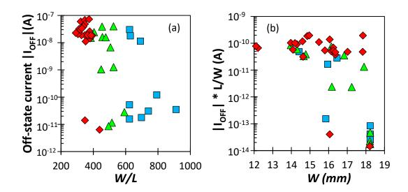
**Figure 4.17:** Off-state drain current (a) and normalised off-state drain current (b) as functions of W/L and width W respectively, for channel length L=20 to 30  $\mu$ m (squares), 30 to 40  $\mu$ m (triangles) and 40 to 50  $\mu$ m (diamonds).
