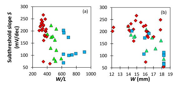
**Figure 4.18:** Subthreshold slope as a function of W/L (a) and W (b) for wide-gate OTFTs with interdigitated source/drain contacts and L = 20 to 30  $\mu$ m (square), L = 30 to 40  $\mu$ m (triangles), or L = 40 to 50  $\mu$ m (diamonds).
