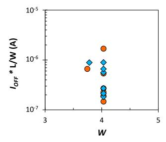
**Figure 4.10:** Normalised off-state drain current as a function of W for narrow-gate OTFTs with interdigitated source/drain contacts and  $L < 10 \, \mu m$  (circles) or L = 10 to  $20 \, \mu m$  (diamonds).
