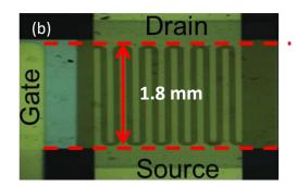
**Figure 4.13:** Gate width manipulation in wide-gate OTFTs resulting in reduced gate width of 1.4 mm and W = 15.40 mm (a) and full gate width of 1.8 mm and W = 18.23 mm (b). Dashed horizontal lines show the gate width boundaries.
