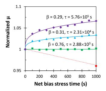
**Figure 5.7:** Normalised filed-effect mobility of freshly fabricated OTFTs as a function of net bias stress time. The legend of Fig. 5.5 applies.
