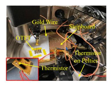
**Figure 3.15:** Temperature sensor measurement setup
