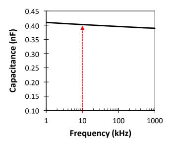
**Figure 3.4:** MIM capacitance as a function of AC frequency.
