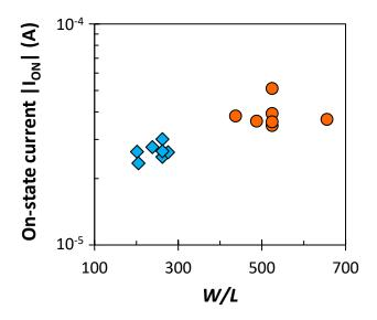
**Figure 4.7:** On-state drain current as a function of W/L for narrow-gate OTFTs with interdigitated source/drain contacts and  $L < 10 \, \mu m$  (circles) or L = 10 to 20  $\mu m$  (diamonds).
