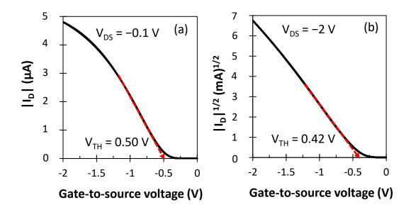
Figure 3.7: Threshold voltage extraction from slopes of  $I_D$  and  $\sqrt{I_D}$  as functions of  $V_{GS}$  in linear ( $V_{DS} = -0.1 \text{ V}$ ) (a) and saturation ( $V_{DS} = -2 \text{ V}$ ) (b) regimes.
