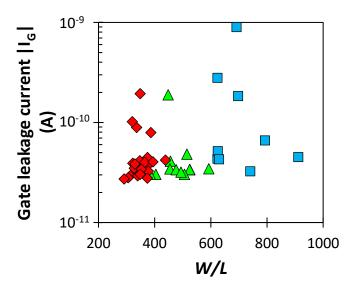
**Figure 4.19:** Gate leakage current as a function of W/L for wide-gate OTFTs with interdigitated source/drain contacts and L=20 to 30  $\mu$ m (square), L=30 to 40  $\mu$ m (triangles), or L=40 to 50  $\mu$ m (diamonds).
