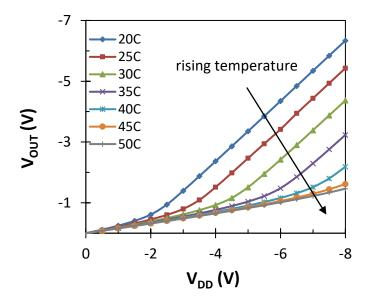
**Figure 6.7:**  $V_{\text{OUT}}$  as a function of  $V_{\text{DD}}$  for temperatures between 20 and 50°C,  $R_{\text{G}} = 50 \text{ k}\Omega$ ,  $R_{\text{D}} = 47 \text{ k}\Omega$  and  $V_{\text{IN}} = -4\text{V}$ .
