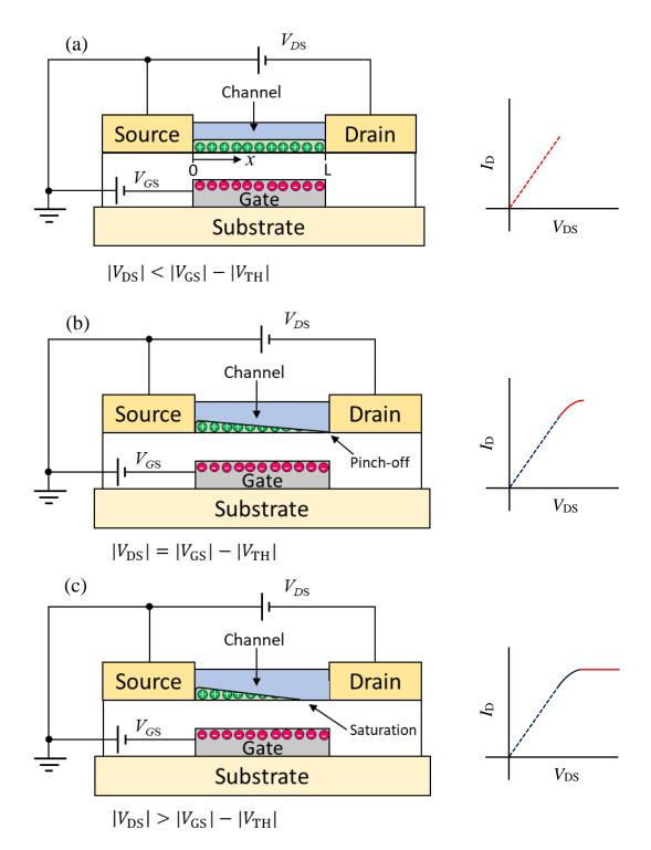
**Figure 2.3:** OTFT channel formation. Linear regime ( $|V_{DS}| < |V_{GS}| - |V_{TH}|$ ) (a), pinch-off ( $|V_{DS}| = |V_{GS}| - |V_{TH}|$ ) (b), and saturation regime ( $|V_{DS}| > |V_{GS}| - |V_{TH}|$ ) (c).
