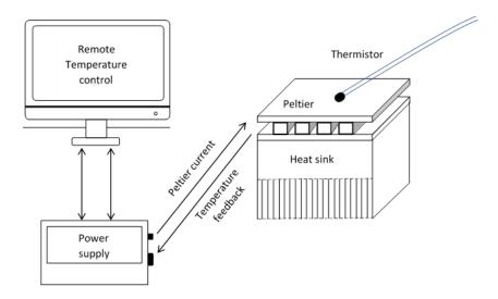
**Figure 3.16:** Thermistor temperature control system setup.
