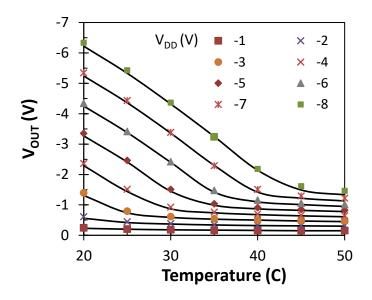
**Figure 6.8:**  $V_{\rm OUT}$  of temperature sensor as a function of temperature between 20 and 50°C for  $R_{\rm G} = 50$  kΩ,  $R_{\rm D} = 47$  kΩ, and  $V_{\rm IN} = -4$  V. The solid black lines in (c) correspond to the sensor model.
