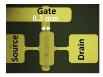
**Figure 4.3:** Top-view of narrow-gate width OTFT with  $L = 17 \mu m$  and W = 4.03 mm.
