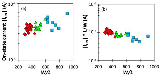
**Figure 4.16:** On-state drain current (a) and normalised on-state drain current (b) as functions of W/L and channel lengths L=20 to 30  $\mu$ m (squares), 30 to 40  $\mu$ m (triangles) and 40 to 50  $\mu$ m (diamonds).
