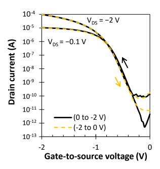
**Figure 3.10:** OTFT hysteresis measurement, forward ( $V_{\rm GS} = 0$  to -2 V) and reverse ( $V_{\rm GS} - 2$  to 0 V) sweep (arrows show the direction of sweep) in linear ( $V_{\rm DS} = -0.1$  V) and saturation ( $V_{\rm DS} = -2$  V) regimes.
