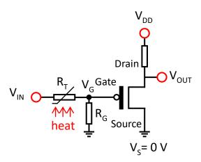
**Figure 3.14:** OTFT-based temperature sensor schematic.
