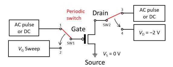
**Figure 3.13:** Bias stress setup. The same AC pulse or DC bias were applied to gate and drain (switch positions 1 and 3 respectively). Transfer characteristics were measurement by sweeping  $V_{GS}$  from 0 to -2 V and  $V_{DS} = -2$  V (saturation) and  $V_S = 0$  V (synchronised switch to positions 2 and 4 respectively).
