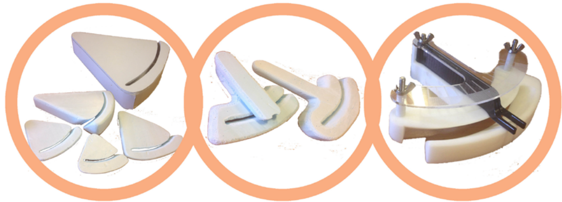
Figure 5-27 Prototypes (a) Kappa board and Foam (b) Alternate Form Models (c) FDM models
