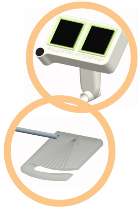
Figure 5-19 Concept Development: CAD of (a) Magnetic Compass (b) Positioning Guide
