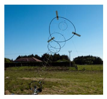
Figure 3.7: Image of a rigid rotor Daisy Kite prototype undergoing field tests (August 2019).
