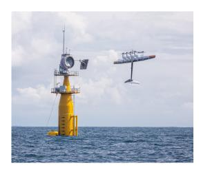
Figure 2.4: Makani's M600 being tested off the coast of Norway (August 2019) [4]
