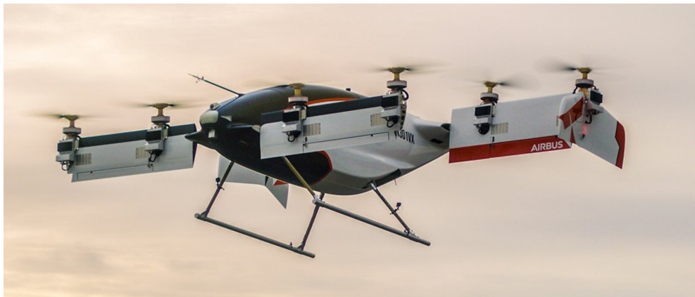
Figure 6.1: A 3 Vahana EVTOL during test flight [15]
