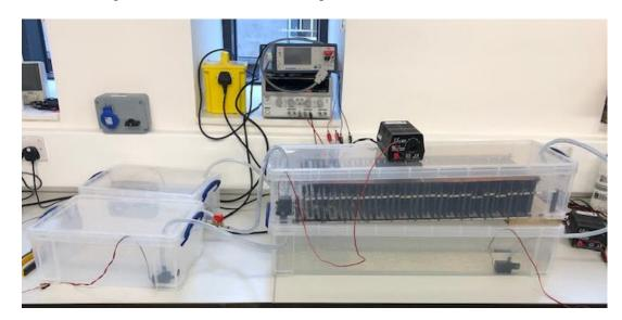
Fig. 6.15 Water desalination test rig
