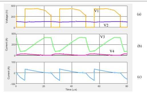
Fig. 2.22 DCDL snubber using  $20\mu$ F capacitor and  $10\mu$ H inductor to create clamp operation. (a)(V1) Q1 Switch Voltage (Vds), (a)(V2) Capacitor Voltage (Vcap), (b)(V3) Secondary (L2) inductor current, (b)(V4) Primary (L1) inductor current, (c) Snubber capacitor (C2) current
