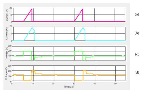
*Fig. 5.2 Simulated switching waveforms of the asymmetrical half-bridge coupled-inductor buck converter. (a) Q1 source current, (b) Primary (L1) inductor currnet, (c) D2 Voltage, (d) Q1 Switch Voltage (Vds)*
