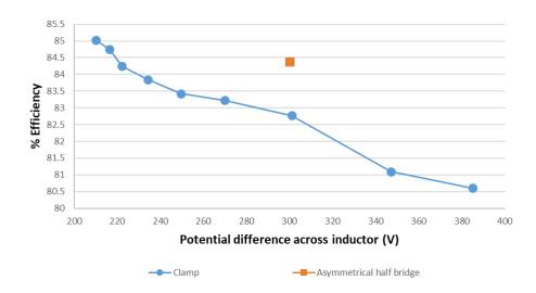
Voltage across Inductor vs Efficiency
