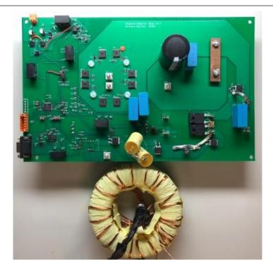
Fig. 4.5 Coupled-inductor circuit prototype
