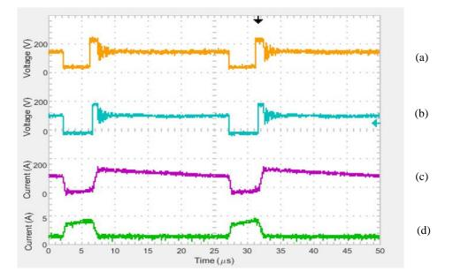
Fig. 6.25 Two full switching cycles for 1.8V super-capacitors. (a) Q1 Switch Voltage (Vds), (b) Q2 Switch Voltage (Vds), (c) Secondary (L2) inductor current, (d) Primary (L1) inductor current
