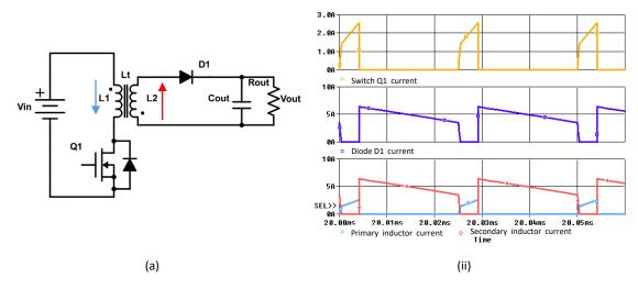
*Fig. 2.3 Single switch flyback converter: (i) schematic and (ii) simulation currents for switch Q1, diode D1 and the primary and secondary of Lt.*
