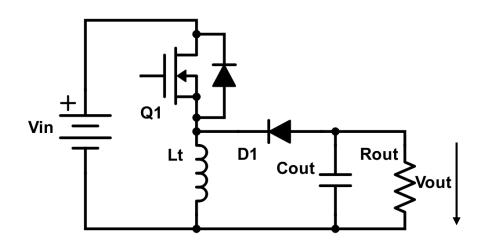
Fig. 2.2 Buck-boost converter
