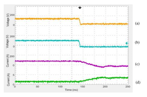
Fig. 6.23 Primary switch turn on for 1.8V super-capacitors. (a) Q1 Switch Voltage (Vds), (b) Q2 Switch Voltage (Vds), (c) Secondary (L2) inductor current, (d) Primary (L1) inductor current
