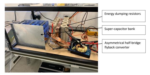
Fig. 6.16 Complete super-capacitor test setup
