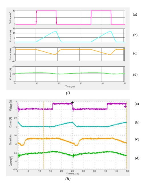
*Fig. 3.5 Flyback circuit waveforms with 2.65:1 turns ratio at a 36% duty cycle: (i) simulated and (ii) experimental. (a) Q1 Gate Signal (Vgs), (b) Primary (L1) inductor current, (c) Secondary (L2) inductor current, (d) Load Voltage R1*
