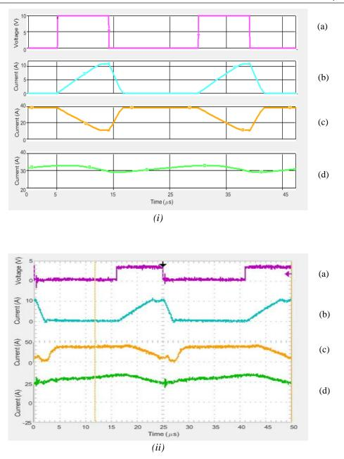
*Fig. 3.6 Coupled-inductor buck converter waveforms with a 2.65:1 turns ratio at a 36% duty cycle: (i) simulated and (ii) experimental. (a) Q1 Gate Signal (Vgs), (b) Primary (L1) inductor current, (c) Secondary (L2) inductor current, (d) Load Voltage R1*
