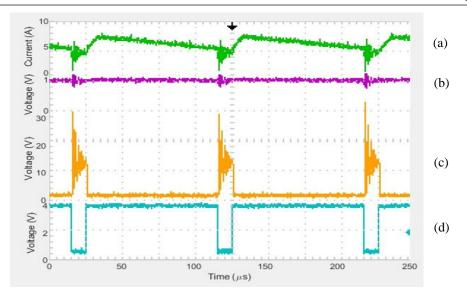
Fig. 4.6 Discontinuous operation with reverse current flow. (a) Secondary (L2) inductor current, (b) Load Voltage R1, (c) Q2 Switch voltage (Vds), (d) Q1 Gate Signal (Vgs)
