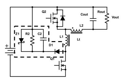
Fig. 2.33 ZRC snubber circuit
