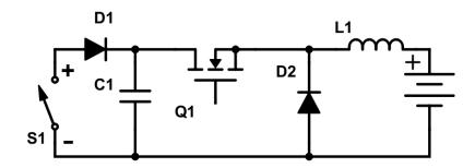
Fig. 4.10 SMPS regenerative snubber, using a buck-boost topology.
