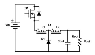
Fig. 2.13 Coupled-inductor buck converter, S5+/-
