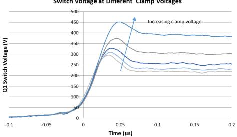
Switch Voltage at Different Clamp Voltages
