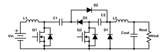
Fig. 2.5 Multi-stage Cuk converter.
