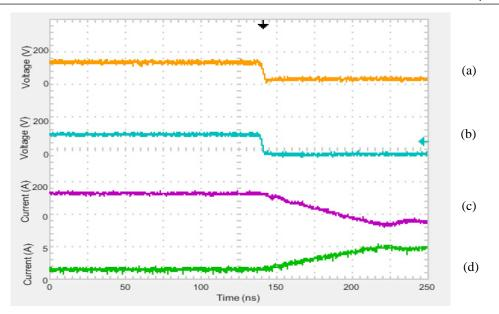
*Fig. 6.20 Primary switch turn on for 1.3V super-capacitors. (a) Q1 Switch Voltage (Vds), (b) Q2 Switch Voltage (Vds), (c) Secondary (L2) inductor current, (d) Primary (L1) inductor current*
