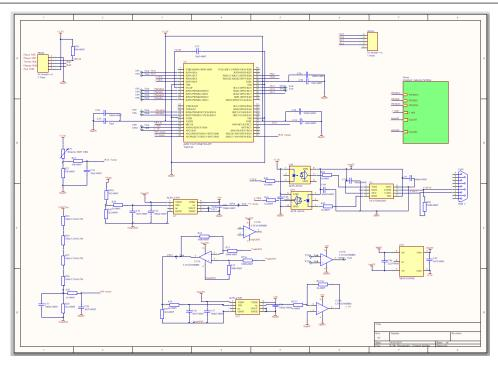
Fig. 6.4 Control and measurements Altium schematic
