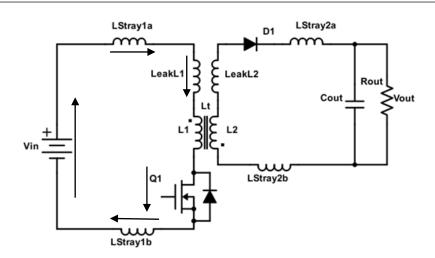
Fig. 2.11 Non idealities on primary side of flyback converter, referred back from the secondary The referred voltage is givens by
