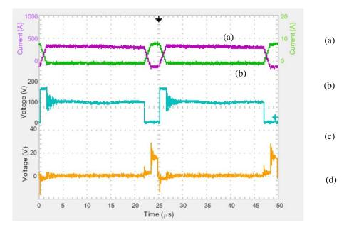
Fig. 6.10 Maximum operation with secondary switch voltage at 29V. (a) Secondary (L2) inductor current, (b) Primary (L1) inductor current, (c) Q1 Switch Voltage (Vds), (d) Q3 Switch Voltage (Vds)
