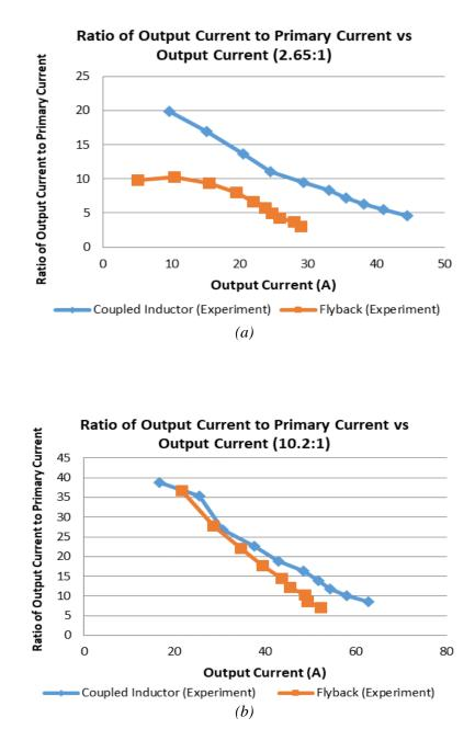
*Fig. 3.10 Ratio of output current to primary current plotted against output current by varying duty cycle, for a turns ratio of: (a) 2.65:1 and (b) 10.2:1.*
