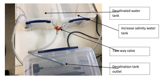
Fig. vi Tubing to determine the path of the flow at the output of the cell.
