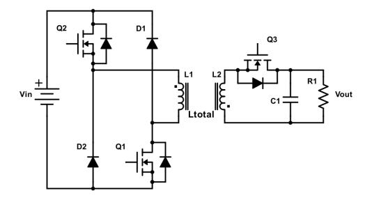
Fig. 6.1 Asymmetrical half-bridge flyback converter
