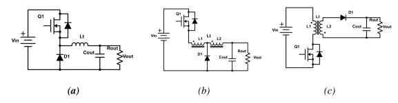
*Fig. 3.1 Circuit schematics of (a) Buck converter, (b) Coupled-inductor buck converter, (c) Flyback converter*
