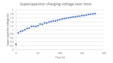
Fig. 6.29 capacitor voltage (charging) 350A
