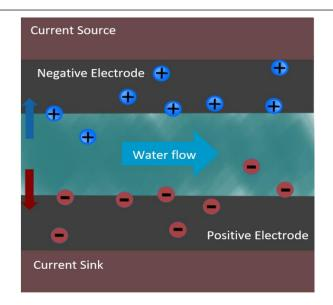
Fig. 1.2 Capacitive deionisation electrode cross section
