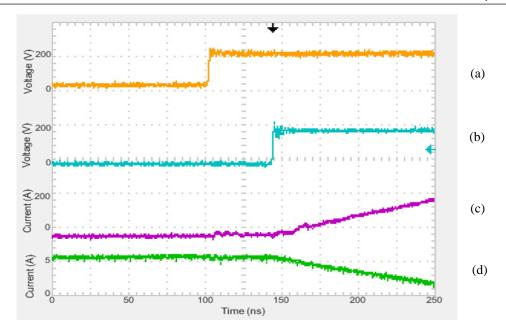
Fig. 6.18 Primary switch turn off showing delay to reduce zero volt ringing at 0.8V. (a) Q1 Switch Voltage (Vds), (b) Q2 Switch Voltage (Vds), (c) Secondary (L2) inductor current, (d) Primary (L1) inductor current
