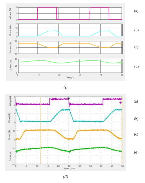
Fig. 3.7 Flyback circuit waveforms with 10.2:1 turns ratio at a 36% duty cycle: (i) simulated and (ii) experimental. (a) Q1 Gate Signal (Vgs), (b) Primary (L1) inductor current, (c) Secondary (L2) inductor current, (d) Load Voltage R1
