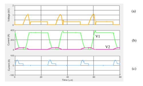
Fig. 4.3 Simulation of regenerative snubber, voltage across Q1 and primary and secondary currents showing conventional operation. (a) Q1 Switch Voltage (Vds), (b)(V1) Secondary (L2) inductor current, (b)(V2) Primary (L1) inductor current, (c) T1 primary current (n1)
