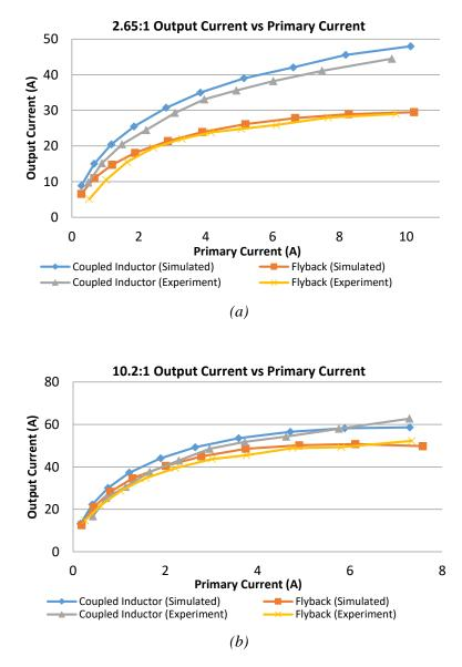
*Fig. 3.9 Output current versus average primary current by varying duty cycle, turns ratio of: (a)* 2.65:1 and (b) 10.2:1.
