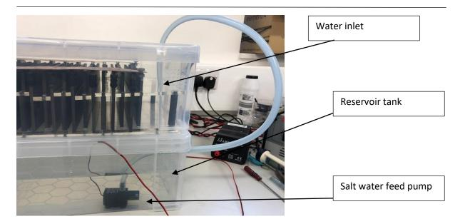
Fig. v Use of water pumps within the test rig
