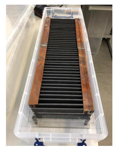
Fig. iv Assembled desalination cell desalination test tank
