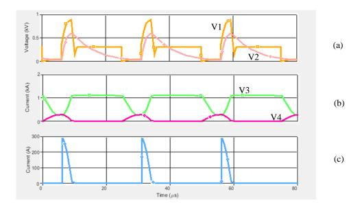
Fig. 2.30 RC snubber simulation with 3:1 turns ratio, C2=700nF, R2=10ohm. (a)(V1) Q1 Switch Voltage (Vds), (a)(V2) C2 Voltage, (b)(V3) Secondary (L2) inductor current, (b)(V4) Primary (L1) inductor current, (c) Snubber Diode (D1) current
