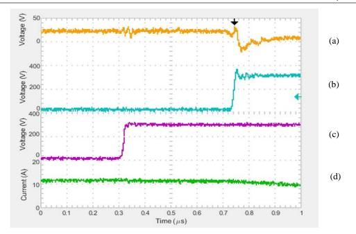
*Fig. 6.13 Rising edge showing the delay of the second switch. (a) Q3 Switch Voltage (Vds), (b) Q1 Switch Voltage (Vds), (c) Q2 Switch Voltage (Vds), (d) Primary (L1) inductor current*
