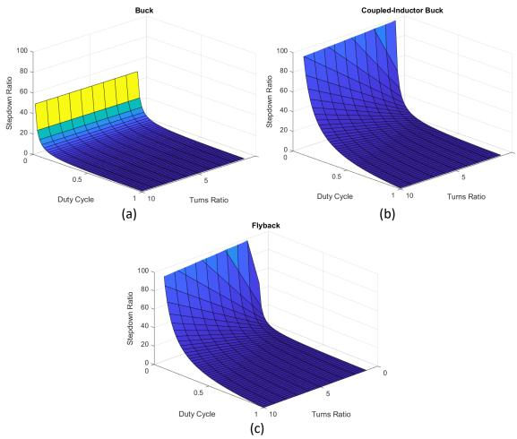
*Fig. 3.2 Voltage transfer ratio versus turns ratio, (a) buck, (b) coupled-inductor buck and (c) flyback.*
