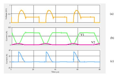
Fig. 2.31 RC snubber simulation with 10:1 turns ratio, C2=700nF,  $R2=10\Omega$ . (a) Q1 Switch Voltage (Vds), (b)(V1) Secondary (L2) inductor current, (b)(V2) Primary (L1) inductor current, (c) Snubber Diode (D1) current
