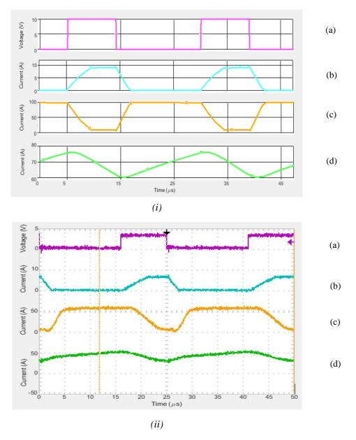
*Fig. 3.8 Coupled-inductor converter waveforms with a 10.2:1 turns ratio at a 36% duty cycle: (i) simulated and (ii) experimental. (a) Q1 Gate Signal (Vgs), (b)Primary (L1) inductor current, (c) Secondary (L2) inductor current, (d) Load Voltage R1*
