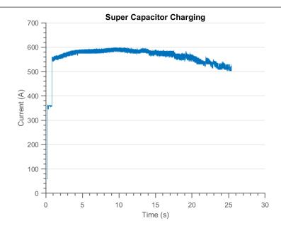
Fig. 6.27 Capacitor charging current (Approx)
