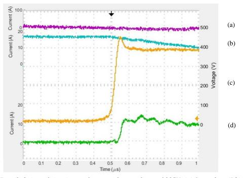
*Fig. 4.17. Detailed view of circuit waveforms at clamp voltage of 385V. (a) Secondary (L2) inductor current, (b) Primary (L1) inductor current, (c) Q1 Switch Voltage (Vds), (d) Snubber diode current (D1)*
