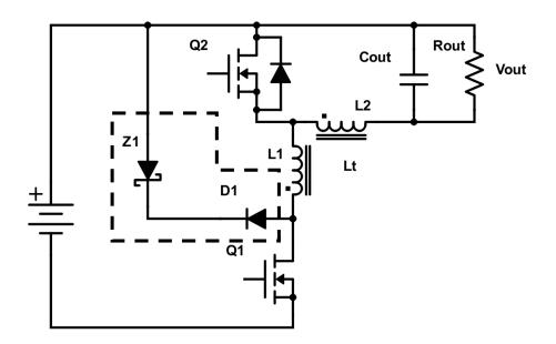
Fig. 2.34 Zener diode snubber circuit
