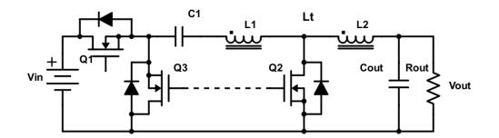
Fig. 2.14 Ultra high step-down ratio converter [50]
