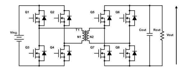
Fig. 2.6 Dual active bridge converter
