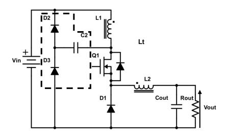
Fig. 2.18 Coupled-inductor buck converter S5+/- with DCD snubber, (Fig. 4 in [44]).
