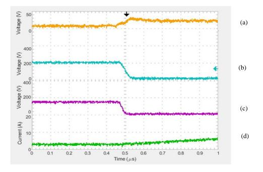
Fig. 6.14 Falling edge. (a) Q3 Switch Voltage (Vds), (b) Q1 Switch Voltage (Vds), (c) Q2 Switch Voltage (Vds), (d) Primary (L1) inductor current
