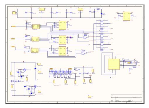
Fig. 6.5 Power and gate driver Altium schematic
