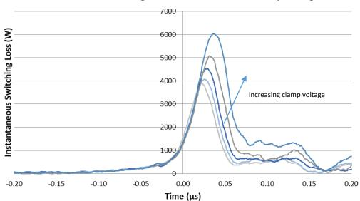
Instantaneous Switching Power Loss at Different Clamp Voltages
