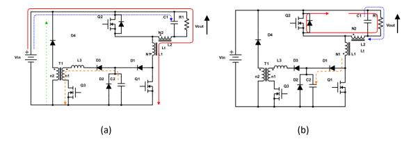
Fig. 4.2 (a)Mode 1 - energising coupled inductor Lt, (b) Q1 turned off discharging Lt.
