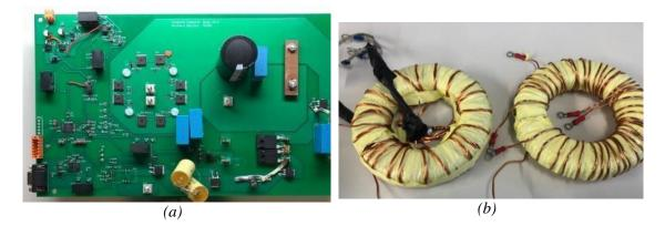
Fig. 3.4 (a) Experimental circuit for testing flyback and coupled-inductor converters and (b) wound coupled inductors  $N_1:N_2=2.65:1$  and 10.2:1 used for both circuits.
