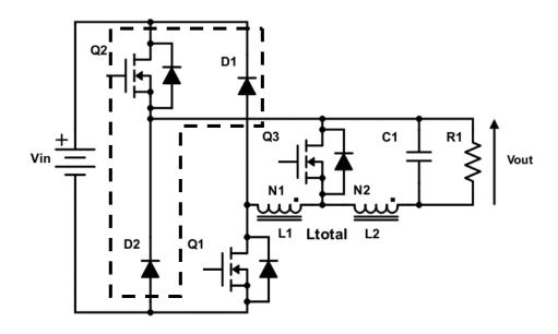
Fig. 5.1 Asymmetrical half-bridge coupled-inductor circuit.
