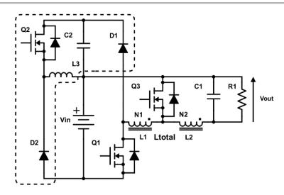
*Fig. 4.11.* Voltage clamp circuit for single-ended coupled-inductor circuit. The dotted line shows the added buck-boost converter with capacitor C2 referenced to V<sub>in</sub>.
