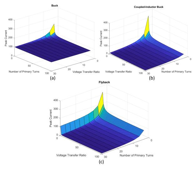
Fig. 3.3 Maximum switch current for 100A load current versus voltage step-down ratio for each circuit against an increasing No. Primary Turns and (Fixed secondary turns = 3) (a) Buck converter (total turns = No. Primary Turns + 3) (b) Coupled-inductor buck converter (c) Flyback converter
