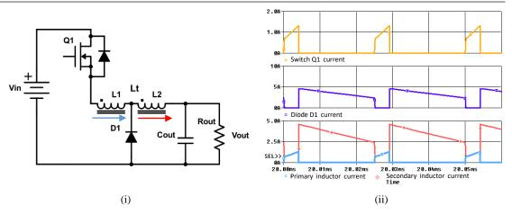
*Fig. 2.9. Coupled-inductor buck converter* S5+/- [46]: (*i*) *Schematic and* (*ii*) *simulated currents for switch Q1, diode D1 and the primary and secondary of Lt.*
