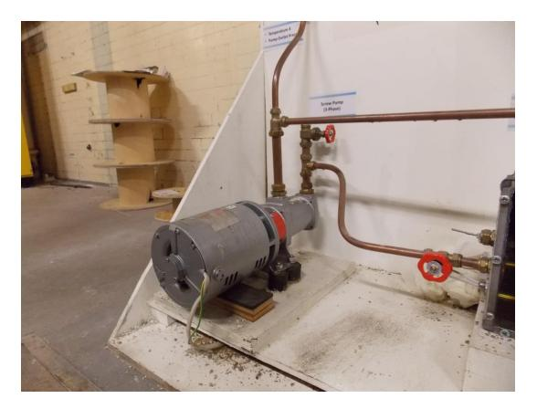
Figure 6.4. Mono CMM263 Progressive Cavity Pump [104].
