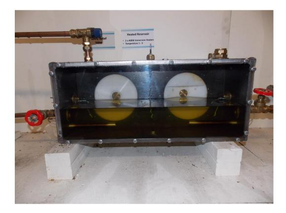
Figure 6.5. Reservoir with 6l of XMP320 lubricant contained inside.
