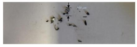
Figure 6.46. Sample of wear particles used for testing morphology.
