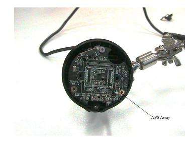
Figure 6.13. APS Array visible in centre of exposed webcam device.
