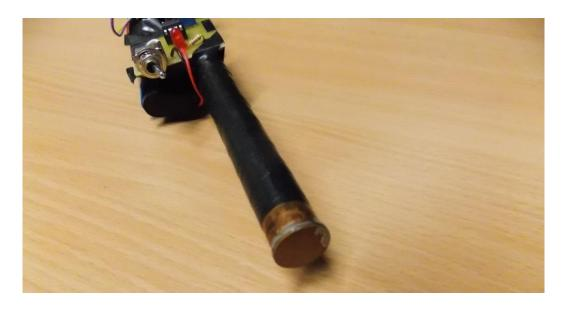
Figure 7.16. Sealed end of pipe to allow samples to be held while IR sensor transmits voltage signal.
