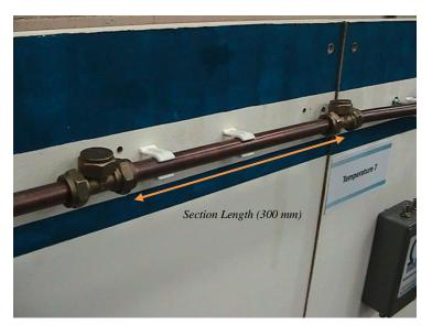
Figure 6.16. Rig with 300 mm copper pipe sections visible.
