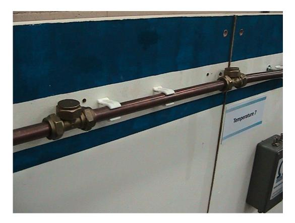
Figure 6.3. Rig with 300 mm copper pipe sections visible.
