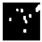
Figure 8.21. Despite low light levels, small 125µm particles could be distinguished from lubricant.
