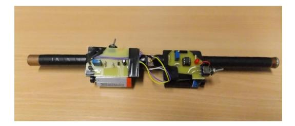
Figure 7.15. Circuit mounted on copper pipe.
