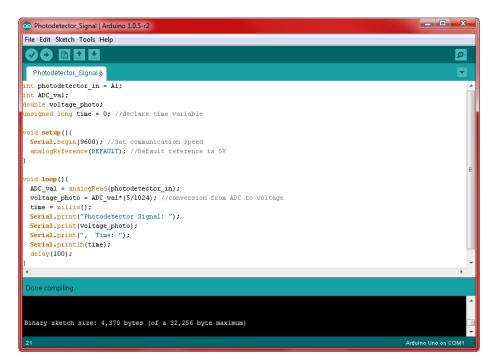
Figure 7.18. Arduino program used to view and log voltage signal.
