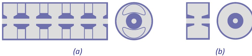
Figure 1.5: Schematic showing the comparison between a five gap EIK (a) to a single-gap klystron cavity (b).
