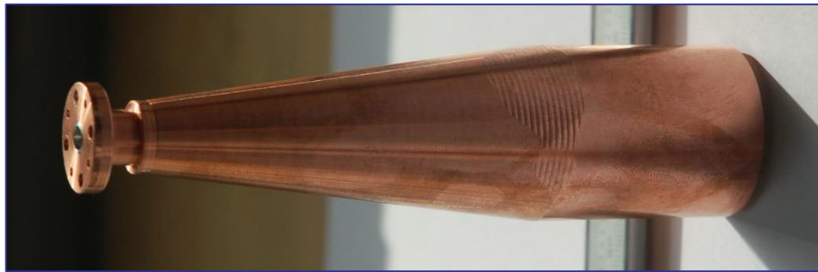
(a) Machined copper on aluminium former
