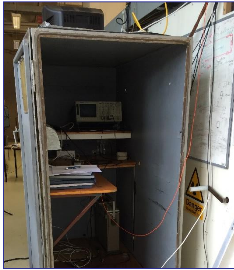
Figure 8.4: Electromagnetically screened room
