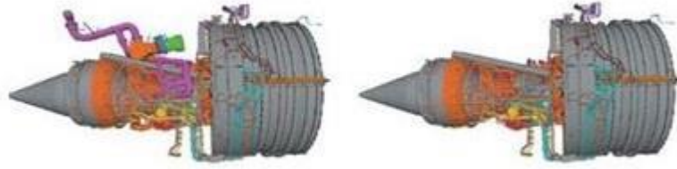
Figure 1. Comparison of a conventional jet engine (left) and a bleed-less (right) [19].
