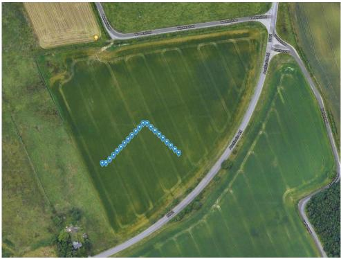
Figure 102. Energy optimised waypoints plotted on satellite map
