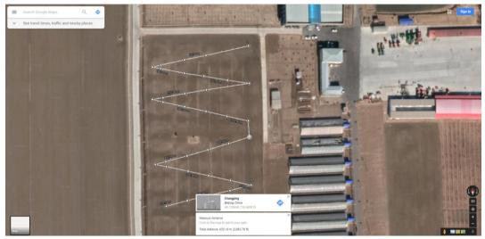
Figure 109. A complete robotic soil sampling plan for the NERCITA selected farms
