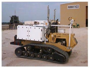
Figure 8. All-Purpose Remote Transport System (Wit, 2000)
