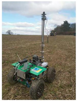
Figure 2. AgriRover, prototype with soil sampling and analysis system in a field
