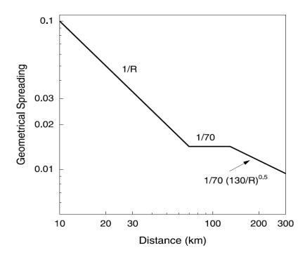
**Figure 5.3** *Geometrical spreading function developed by Boore and Atkinson (1995).*  $R_0 = 1$ ,  $R_1 = 70$ ,  $R_2 = 130$ ,  $p_1 = 0.0$  and  $p_2 = 0.5$ . Taken from Boore (2003).
