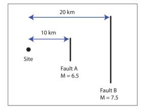
Figure B.1 Fault sources with different associated magnitudes and source-to-site distances. Taken from Baker (2015).
