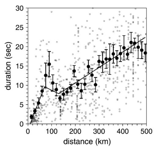
**Figure 5.5** Observed duration (once source duration is subtracted) for earthquakes from an arbitrary region. The solid circles represent averages within 15 km wide bins. The error bars are +/- one standard deviation of the mean. The three-part solid line is the path-dependent duration function developed by Atkinson and Boore (1995). Taken from Boore (2003).
