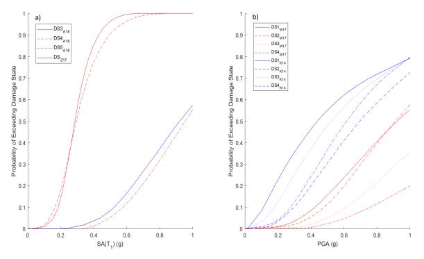
Figure 8.6 Considered fragility curves for (a) FSJ platforms and (b) 5-MW offshore wind turbines.
