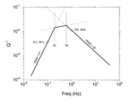
**Figure 5.4** *Illustration of* Q(f). The specification is composed of three line segments in log-log space. Taken from Boore (2003).
