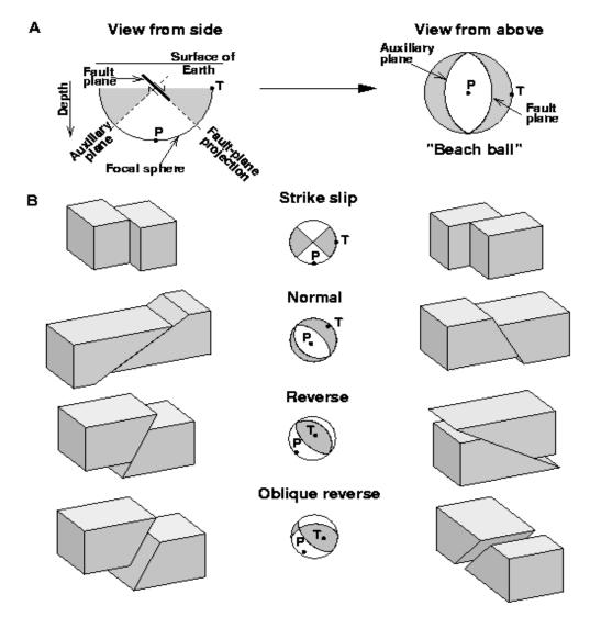
Figure A.4 Schematic diagram for earthquake focal mechanisms. Taken from Earthquake.usgs.gov (2018).
