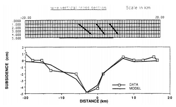
**Figure D.3** Comparison between observed and calculated surface displacements due to fault slips for the Lacq field. Calculated surface displacements from Grasso (1992) two-part mechanism for temporal strain modelling. Adopted from Grasso (1992).
