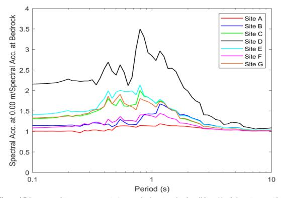
**Figure 4.7** *Recomputed (response spectra) site transfer functions for the offshore North Sea sites considered by Rognlien (1987).* Subsurface profiles for each site are provided in Tab. 4.1.
