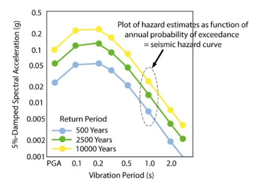
Figure B.8 Arbitrary uniform hazard spectrum for three return periods. Adapted from Goda et al. (2014).
