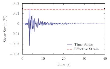
**Figure C.5** Comparison of strain time-series and corresponding effective stress for a target layer within an *ELSR analysis*. Taken from Kottke and Rathje (2008).
