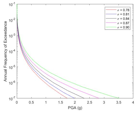
**Figure 5.0** Seismic hazard curve demonstrating the impact of modifying  $\sigma$  within a PSHA. Predicted groundmotion was computed using the Bindi et al. (2017) GMPE for a North Sea site (latitude = 66, longitude = 16,  $\lambda = 0.0758$ ) using the seismic zonation of Bungum et al. (2000).
