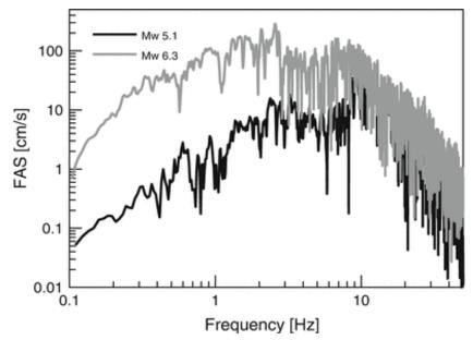
**Figure 3.6** Fourier amplitude spectra for acceleration time series recorded for different sized earthquakes recorded at the same site and similar source-to-site distances. Taken from Pacor and Luzi (2014).
