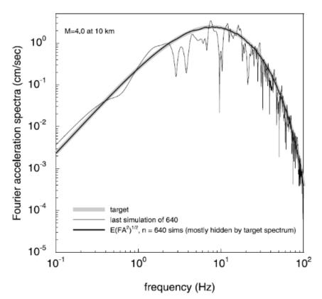
**Figure 5.10** *The target spectrum, the spectrum from a single realisation and the spectrum from an average of 640 realisations.* The simulations were undertaken using an arbitrary seismological model. Taken from Boore (2003).
