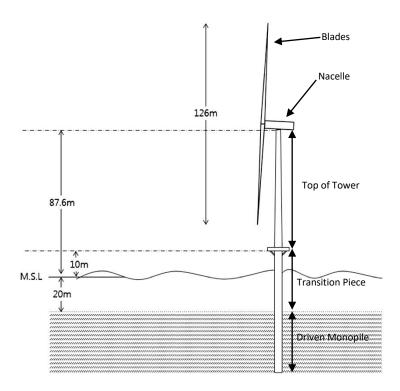
**Figure 8.4** *Simple two-dimensional schematic of a 5-MW offshore wind turbine*. M.S.L = mean sea level. Adapted from Kim et al. (2014).
