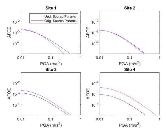
**Figure 7.6** *PGA seismic hazard curves for the considered North Sea sites.* AFOE = annual frequency of exceedance. Site locations provided in Fig. 7.5.
