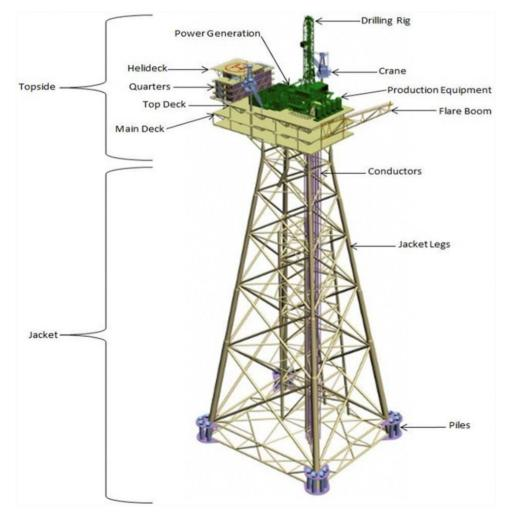
Figure 8.3 Simple schematic diagram of a fixed-steel jacket platform. Taken from Bull and Love (2019).
