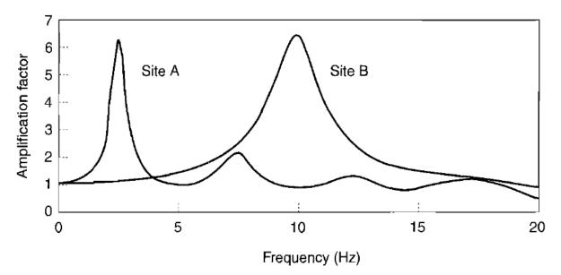
**Figure C.0** *Amplification factor against frequency for a low stiffness site (Site A) and a high stiffness site (Site B).* Taken from Kramer (2014).
