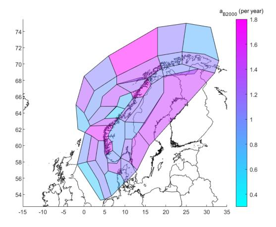
**Figure 7.0** Seismogenic source zonation model of Bungum et al. (2000) with the original a-values ( $a_{B2000}$ ). The a-value for each source zone has been normalised by the duration of the Bungum et al. (2000) earthquake catalogue.
