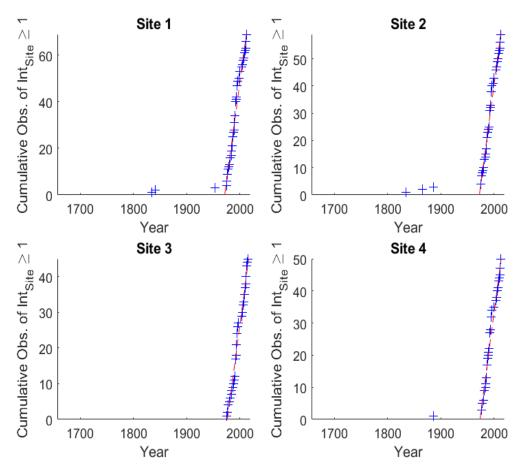
**Figure 7.9** *Plots of cumulative number of MDPs (intensity*  $\geq 1$ ) *against time.* Red dashed line indicates periods for which approximately stable rates of occurrence are observed.
