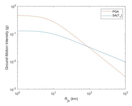
Figure 8.8 Ground-motion intensity vs.  $R_{jb}$  for an  $M_L$  6.5 earthquake using the Akkar et al. (2014) GMPE.
