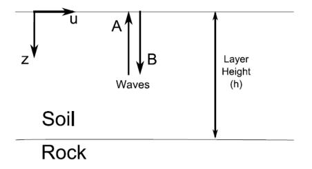
**Figure C.1** *Notation for the one-dimensional wave form equation (equation C.3).* Taken from Kottke and Rathje (2008).
