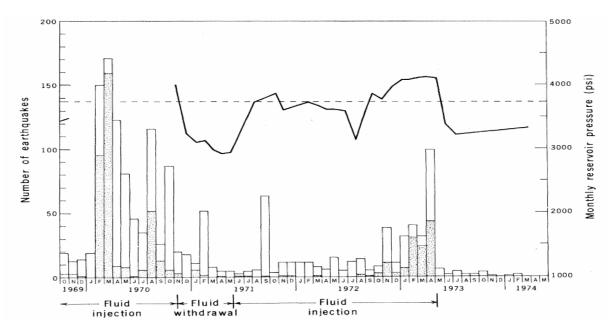
**Figure D.0** Frequency of earthquakes at Rangely field and temporal association with fluid injection. Stippled bars indicate earthquakes  $\leq 1$  km of the experimental injection wells. Clear areas indicate all others. Pressure history shown by heavy line; predicted critical pressure by dashed line. Taken from Rayleigh et al. (1976).
