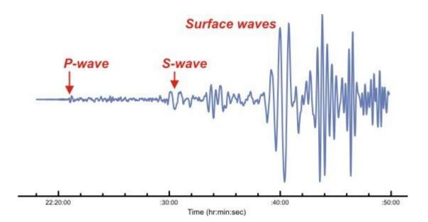
**Figure A.1** Seismogram for an arbitrary earthquake demonstrating arrival time offset for *P*-waves, *S*-waves and surface waves. Adapted from Earthquakes.bgs.ac.uk (2020b). Contains British Geological Survey materials @NERC 2020.
