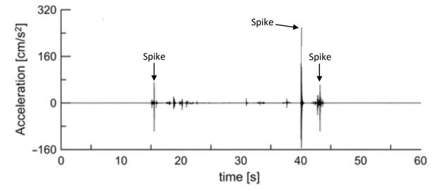
Figure 3.1 Example of spurious spikes in a digitised record. Adapted from Pacor and Luzi (2014).
