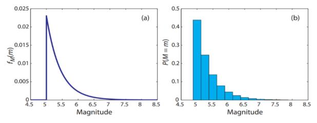
**Figure B.4** Conversion of a continuous magnitude distribution (a) into a discrete magnitude distribution (b) for a hypothetical source with a truncated Gutenberg-Richter distribution with a minimum considered magnitude of 5, a maximum magnitude of 8 and a b parameter of 1. Taken from Baker (2015).
