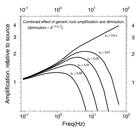
**Figure 5.7** *Combined effect of the site amplification and the path-independent attenuation.* Taken from Boore (2003).
