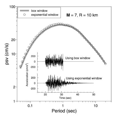
**Figure 5.9** Comparison of waveforms and peak surface velocity (PSV) response spectra for time-domain simulations using the box and exponential (shaped) windows to shape the noise. The response spectra are averages from a suite of 640 simulations. The time series are for a single realisation. The simulations were undertaken using an arbitrary seismological model. Taken from Boore (2003).
