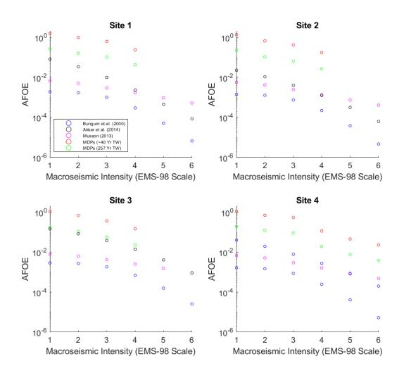
Figure 7.10 Intensity hazard curves computed from the MDPs and the North Sea PSHA calculations.
