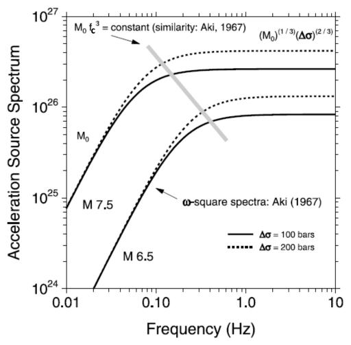
**Figure 5.2** Source scaling for single corner frequency  $\omega$ -square model. For constant stress drop  $M_0 f_0$  is a constant (Aki, 1967). The dependence of the corner frequency ( $f_0$ ) on the seismic moment ( $M_0$ ) (represented by the shaded line) determines the scaling of the spectral shapes. Taken from Boore (2003).
