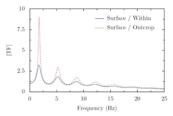
**Figure C.3** *Transfer function for a site with given geotechnical properties, considering different inputs.* These geotechnical conditions are provided in Tab. C.0. See below for an explanation of "within" and "outcrop" motion terminology. Taken from Kottke and Rathje (2008).
