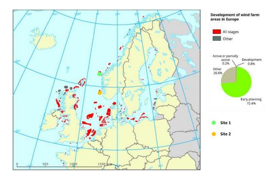
**Figure 8.5** *Spatial distribution of offshore wind farm development in northwestern Europe.* The locations for which seismic hazard estimates are computed below are also provided. Adapted from eea.europa.eu. (2015). This image has been modified and is available for reuse under the creative commons license (CC BY 2.5 DK) as per https://creativecommons.org/licenses/by/2.5/dk/deed.en\_GB:
