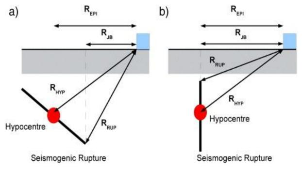
**Figure A.3** Schematic diagram for the four common source-site distance metrics for a) dipping fault, and b) a vertical fault.  $R_{epi}$  = epicentral distance,  $R_{hyp}$  = hypocentral distance,  $R_{jb}$  = Joyner–Boore distance and  $R_{rup}$  = rupture distance. Taken from Weatherill and Burton (2010).
