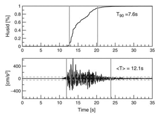
**Figure 3.5** Acceleration time series with bracketed duration (bottom) and corresponding Husid plot with significant duration (top). Values within 5% and 95% of the integral of the square of ground-acceleration were considered. Taken from Pacor and Luzi (2014).
