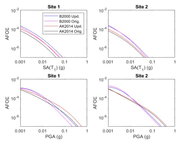
**Figure 8.7** *Seismic hazard curves for sites in the North Sea.* B2000 = Bungum et al. (2000) GMM. AK2014 = Akkar et al. (2014) GMPE. Upd. = updated source zone parameters. Orig. = original source zone parameters.
