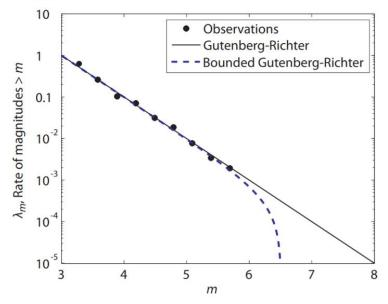
**Figure B.3** *A Gutenberg-Richter distribution, a bounded Gutenberg-Richter distribution and observed data for an arbitrary region.* Taken from Baker (2015).
