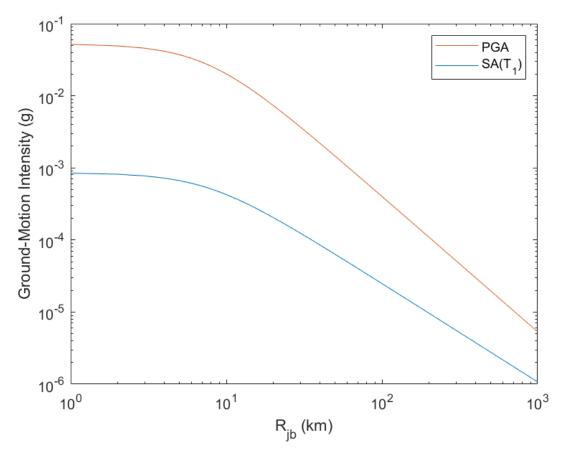
Figure 8.9 Ground-motion intensity vs.  $R_{jb}$  for an  $M_L$  4.2 earthquake using the Akkar et al. (2014) GMPE.
