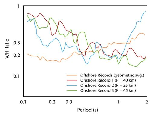
**Figure 4.6** V/H spectra for the geometric average of the offshore SEMS sites and select onshore records. The onshore sites are underlain by soils with S-wave velocities similar to those estimated to lie beneath the SEMS sites. Adapted from Boore and Smith (1999).
