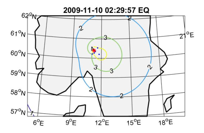
**Figure 7.8** *Isoseismal contours (EMS-98 scale) generated for the 1979/06/14 21:24:12 and 2009-11-10 02:29:57 earthquakes.* Red asterisk represents the earthquake epicentres. Blue dots represent existing MDPs for the earthquakes.
