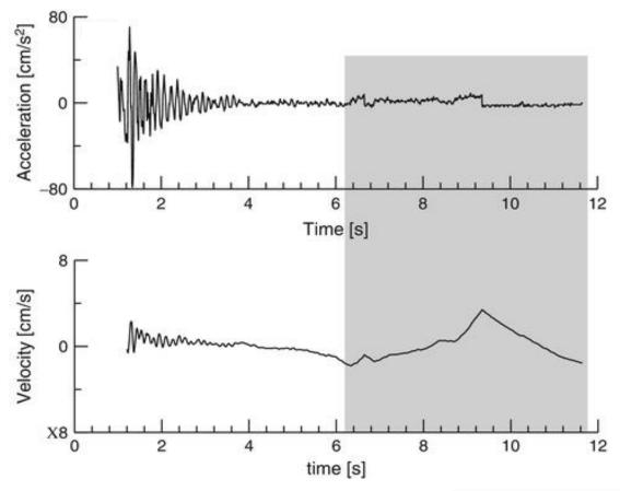
**Figure 3.2** *Example of baseline shift and its effect on the velocity time series.* The grey box highlights the differences. Taken from Pacor and Luzi (2014).
