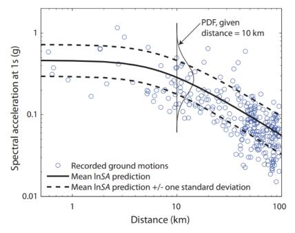
**Figure B.7** Observed spectral accelerations for a period of 1 second from the 1999 Chi-Chi, Taiwan earthquake and a predicted distribution computed using the Campbell and Bozorgnia 2008 GMPE. Taken from Baker (2015).
