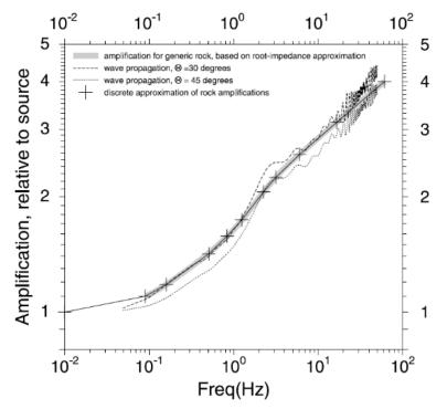
**Figure 5.6** Amplification vs. frequency. The segmented-line function used in the stochastic method is represented by the lines joining the plus symbols. Taken from Boore (2003).
