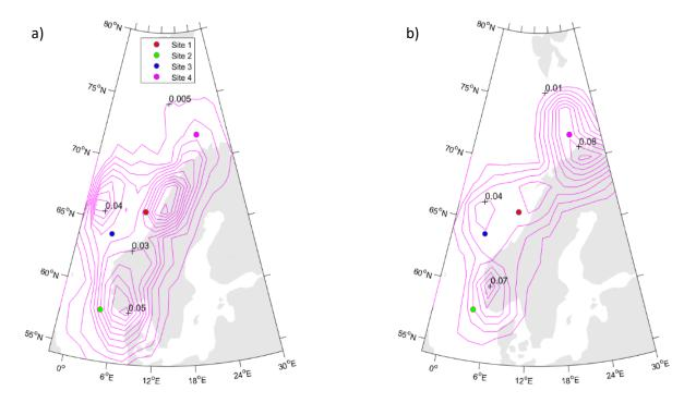
**Figure 7.5** (a) North Sea PGA seismic hazard map computed using the (normalised) updated source parameters computed within this investigation and (b) North Sea PGA seismic hazard map computed using the (normalised) original source parameters of Bungum et al. (2000). PGA is in m/s<sup>2</sup>. Seismic hazard maps were computed for a return period of 475 years using the Bungum et al. (2000) GMM.
