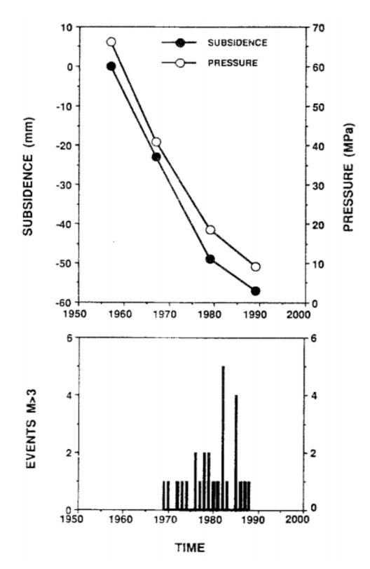
**Figure D.2** Seismic and aseismic deformation of the Lacq gas field as a function of pressure decrease within the gas reservoir. Taken from Grasso (1992).
