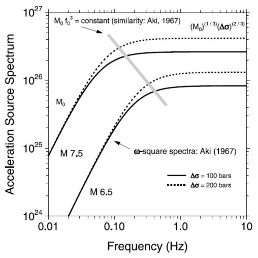
**Figure A.2** Source scaling for single corner frequency  $\omega^2$  model spectral shape. For constant stress drop  $M_0 f_0$  is a constant (Aki, 1967) The dependence of the corner frequency  $(f_0)$  on the seismic moment  $(M_0)$  (represented by the shaded line) determines the scaling of the spectral shapes. Taken from Boore (2003).
