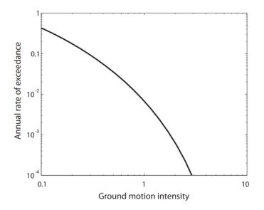
Figure B.0 Seismic hazard curve for an arbitrary return period. Taken from Baker (2015).
