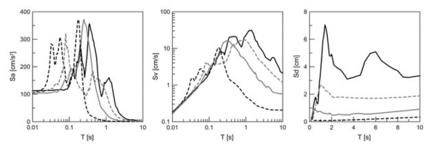
**Figure 3.7** Acceleration response spectra (Sa), velocity response spectra (Sv) and displacement spectra (Sd) for 4 arbitrary acceleration time series. Different axis scales are used to emphasise the different spectral shapes associated with each type of response spectrum. Taken from Pacor and Luzi (2014).
