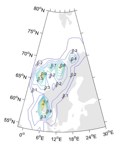
**Figure B.9** *PGA seismic hazard contour map for the Norwegian economic sector of the North Sea computed using the Bungum et al. (2002) logic tree approach (see section X.7 for more information on logic trees in PSHA).* Return period is 475 years. PGA in m/s<sup>2</sup>. Reproduced from Bungum et al. (2002) (see their Fig. 4) using their North Sea source zone data, which was kindly provided by Conrad Lindholm.
