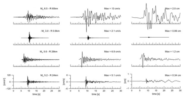
**Figure 3.4** *Example of acceleration time series with similar PGAs*  $(105 - 112 \text{ cm/s}^2)$  but different PGVs and PGDs. Taken from Pacor and Luzi (2014).
