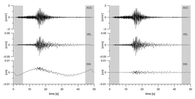
**Figure 3.3** *Example of low-cut filtering with a 0.01 Hz cut-off (left) and a 0.02 Hz cut-off (right).* Taken from Pacor and Luzi (2014).
