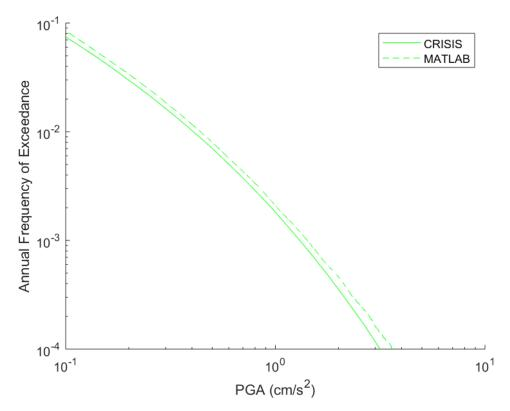
**Figure 4.16** *PGA seismic hazard curves generated using the CRISIS seismic hazard software and the Monte Carlo PSHA program (MATLAB) for an example (low hazard) test site (longitude = 20, latitude = 58).*
