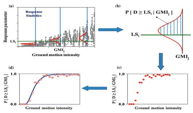
**Figure 8.2** Schematic representation of the fragility curve generation procedure: (a) response statistics, (b) probability of exceeding a limit state at a specific ground-motion intensity, (c discrete fragility information for a predetermined limit state and (d) continuous fragility function. Taken from Erberik (2015).
