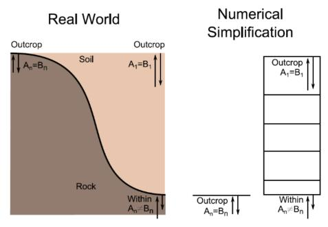
**Figure C.4** Diagram explaining outcrop motion and within motion conditions. Outcrop = upwardly and downwardly propagating ground-motions are equal  $(A_n = B_n)$ . Within = upwardly and downwardly propagating ground-motions are not equal  $(A_n \neq B_n)$ . Taken from Kottke and Rathje (2008).
