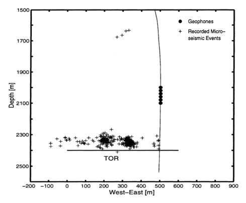
**Figure 2.4** *Vertical section showing locations of 328 micro-earthquakes detected by the seismic array operational in the Valhall field between June 1 and July 27, 1998.* The thin black line represents well path. The thick black line represents the boundary between the overburden and the overlying reservoir. Tor refers to the Tor formation within which the Valhall reservoir is located (rather than the Tor field shown in Fig. 2.2). Taken from Zoback and Zinke (2002).
