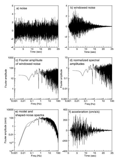
Figure 5.8 Schematic of the time-domain procedure Taken from Boore (2003).
