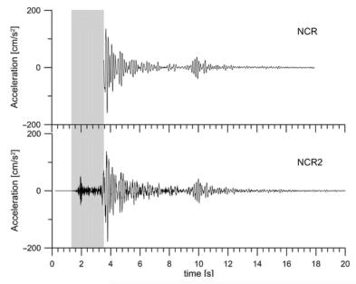
**Figure 3.0** Acceleration time series for the 1997 Umbria-Marche seismic sequence, central Italy recorded at analogue station NCR (top) and digital station NCR2 (bottom). Taken from Pacor and Luzi (2014).
