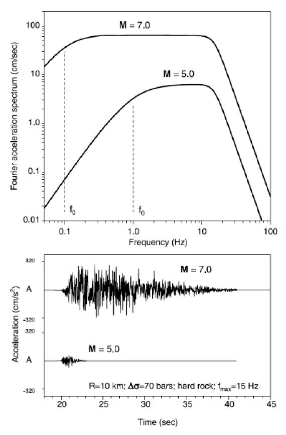
**Figure 5.1** Fourier amplitude spectrums of ground-motion at a particular distance and site condition for earthquakes of magnitudes 5 and 7 based on a standard seismological model and the corresponding timeseries for these ground-motion spectrums. Adapted from Boore (2003).
