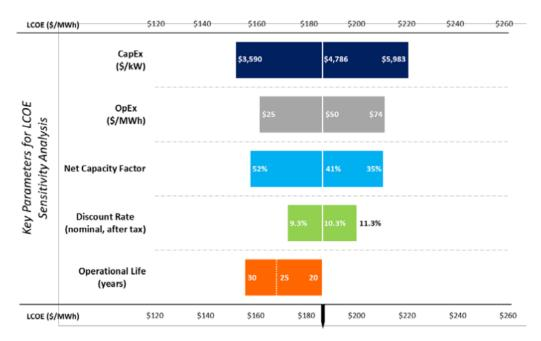
Figure 2.1: Key sensitivity analysis parameters for fixed-bottom offshore wind LCOE from [9].
